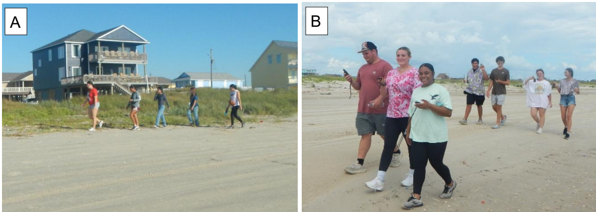
Figure 3. Students mapping (A) the vegetation line and (B) the shoreline (wet/dry line) using handheld GPS units.
