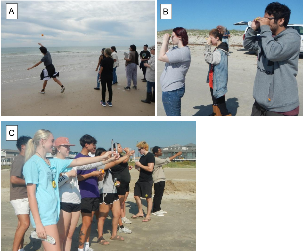
Figure 4. Students (A) throw an orange into the surf to determine longshore current speed and direction, (B) using a sighting compass to determine wind and wave direction, and (C) measuring wind speed using a Dwyer hand-held wind meter.
