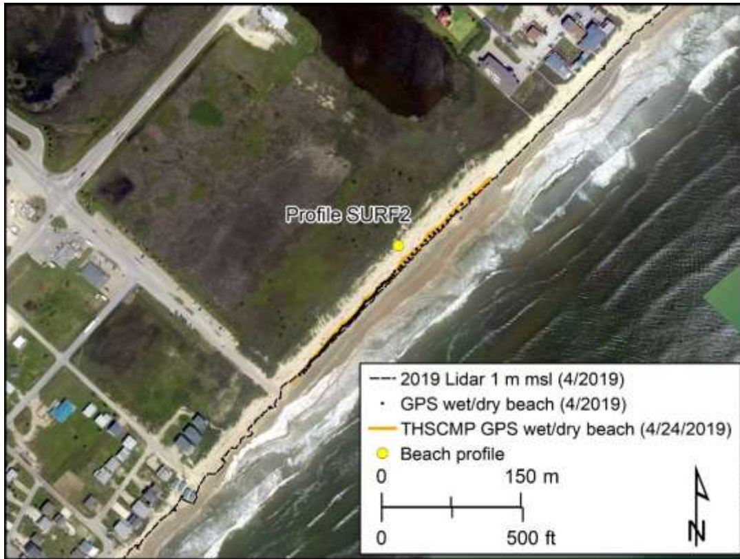
Figure 12. Shoreline position comparison at Surfside Beach site SURF2. Shorelines include the wet-beach/dry-beach boundary mapped on April 24, 2019, by THSCMP students and Bureau staff using ground GPS and the 1 m (3.3 ft) above mean sea level shoreline proxy extracted from airborne lidar data acquired in spring 2019, superimposed on 2019 Bureau imagery. From Paine and others (2021).
