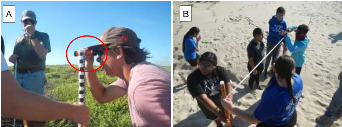
Figure 2. Students use (A) a sighting level to determine vertical offset between Emery rods and (B) a metric tape to measure horizontal distance.
