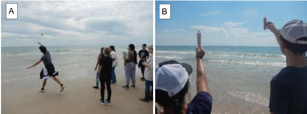
Figure 4. Students (A) throw an orange into the surf to determine longshore current speed and direction and (B) measuring wind speed.
