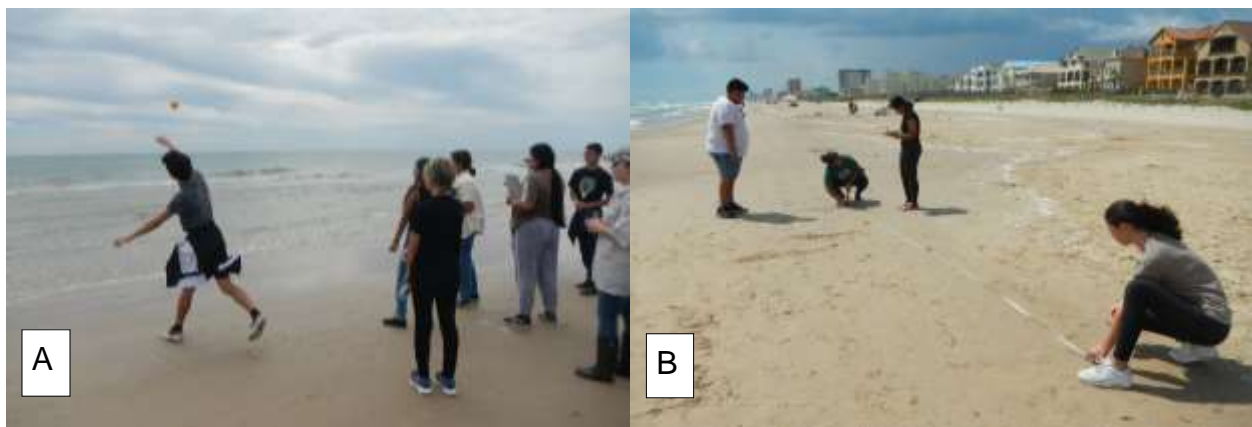
Figure 4. Students (A) throwing an orange to determine longshore current speed and direction and (B) measuring how far along the shoreline the orange drifted to calculate longshore current speed.
