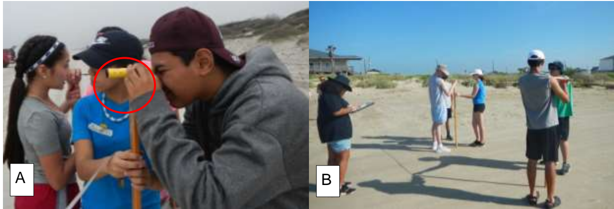
Figure 2. Students using (A) a sighting level to determine vertical offset between Emery rods and (B) a metric tape to measure horizontal distance.
