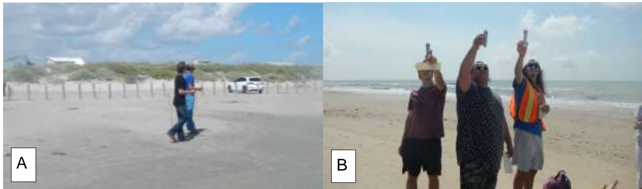
Figure 3. Students mapping (A) the shoreline (wet/dry line) using handheld GPS units and (B) using wind meters to determine wind speed.
