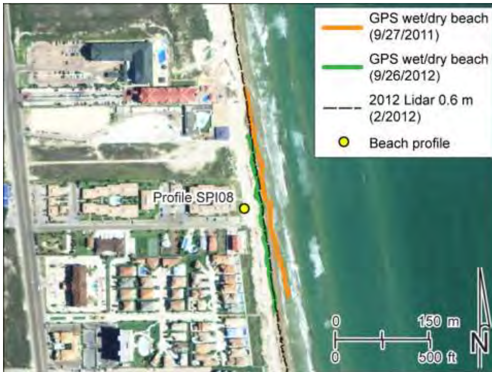
Figure 13. Shoreline position comparison at South Padre Island site SPI08. Shorelines include the wet-beach/dry-beach boundary mapped on September 27, 2011, and September 26, 2012, by THSCMP students using GPS and the shoreline proxy extracted from airborne lidar data acquired in February 2012. Shorelines are superimposed on NAIP imagery acquired on April 23, 2012. From Paine and other (2014).
