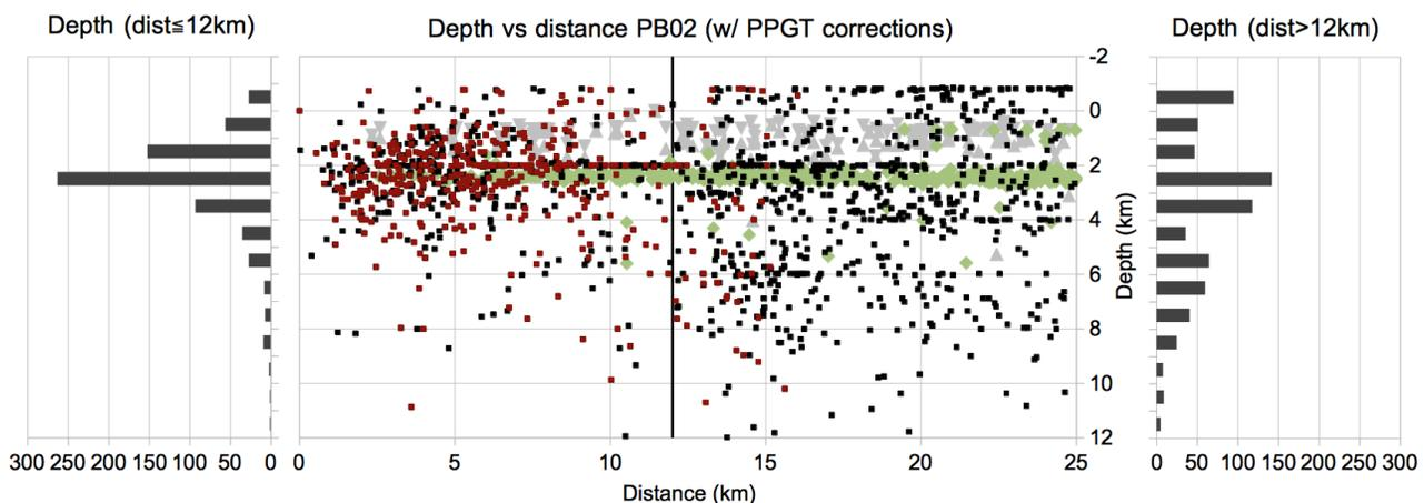
**Figure 1.** Section views showing (Middle) depth as a function of distance from station PB02 and corresponding depth histograms within 12-km distance from station PB02 (left) and 12-25 km distance (right) for relocations using PPGT corrections.
