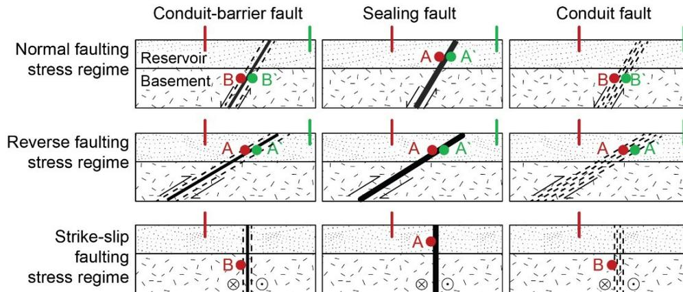
**Figure 1.** Location of fault reactivation relative to position of injector for an optimally oriented fault in normal, reverse, and strike-slip stress regimes and for a conduit-barrier, conduit, and sealing fault permeability structure. Fault reactivation location indicated with letter A or A' for the reservoir and B or B' for the basement section of the fault.
