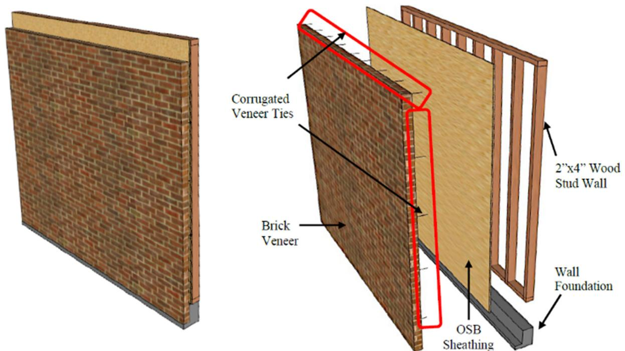
Figure 1. Renderings of brick veneer wall: (a) Actual wall panel as constructed, (b) Actual wall with individual elements labeled.
