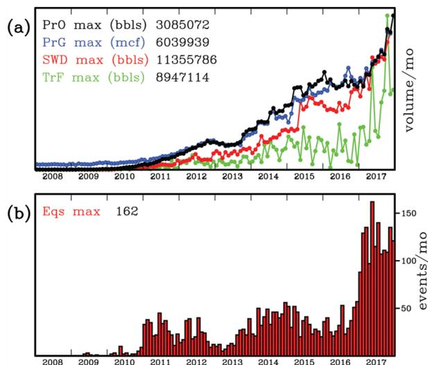
**Figure 1.** Petroleum-production operations and seismicity in 10 km around Pecos City. (a) Monthly volumes for produced oil (PrO), produced gas (PrG), wastewater disposal (SWD), and hydraulic fracturing treatment fluid (TrF). Plotted values on vertical axes are normalized to maximum monthly values, given at upper left. (b) Monthly earthquake numbers in TXAR catalog.
