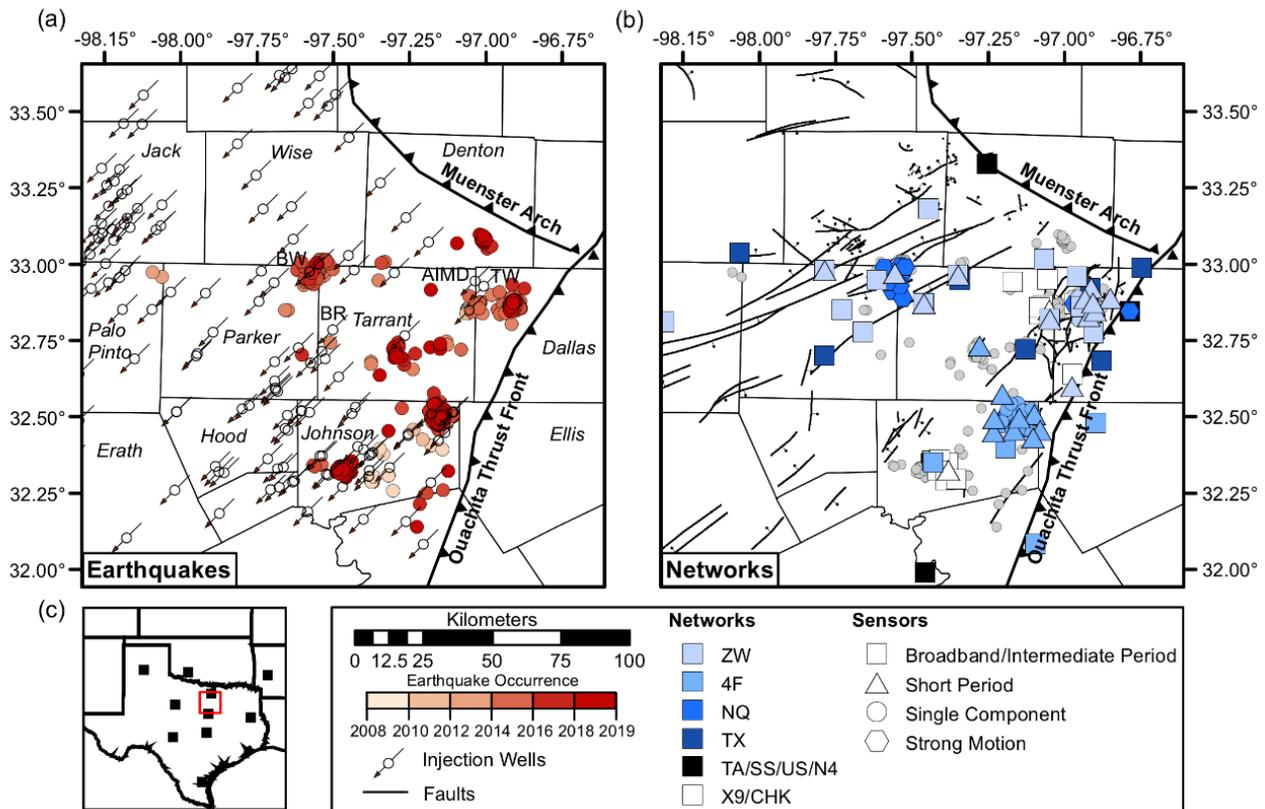
**Figure 1.** Map views showing the (a) locations of the NTXES earthquakes (circles) and injection wells (arrows) with important wells labeled (BR, BW, TW, A1MD), and (b) showing the locations of all stations whose symbol represents the station type. Faults on this map taken from Hennings *et al.*, 2019. (c) General map view showing the locations of regional US and TA stations along with the highlighted study area (box).
