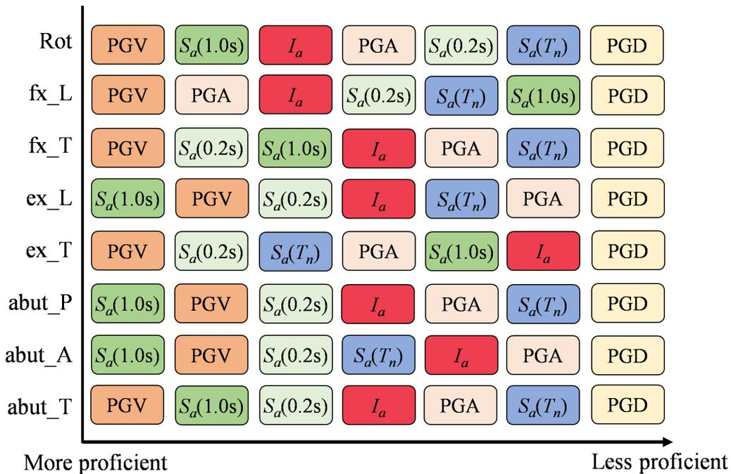
Figure 1. Proficiency evaluation of considered IMs for different demand parameters of steel girder bridges in Texas.
