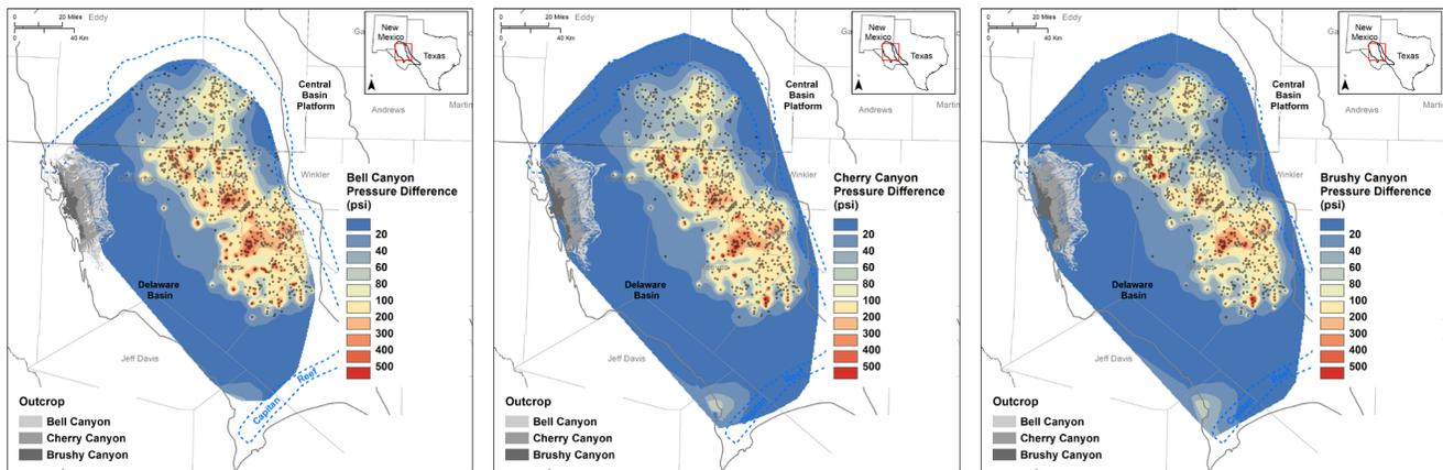
Figure 1. Pressure buildup due to injection from 1982-2018 in the formations of DMG.
