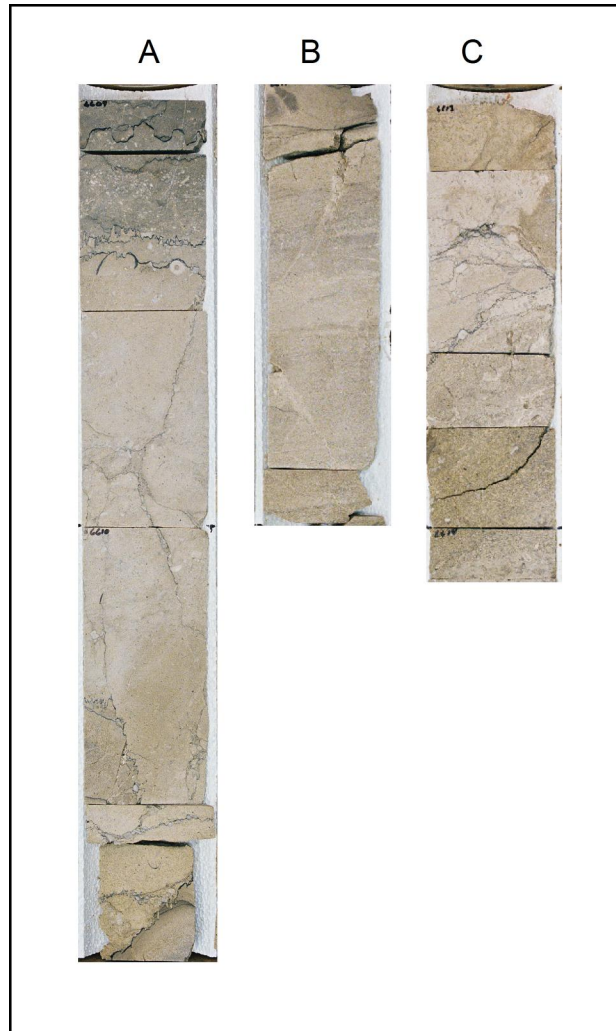
Figure 16. Core photographs showing evidence of karsting in injection interval at 6600–6620 ft log depth. (A) Compacted large breccia at 6609–6611 ft core depth. (B) Small dissolution vug and fractures at 6611–12 ft core depth. (C) Compacted breccia at 6612–6613 ft log depth.
