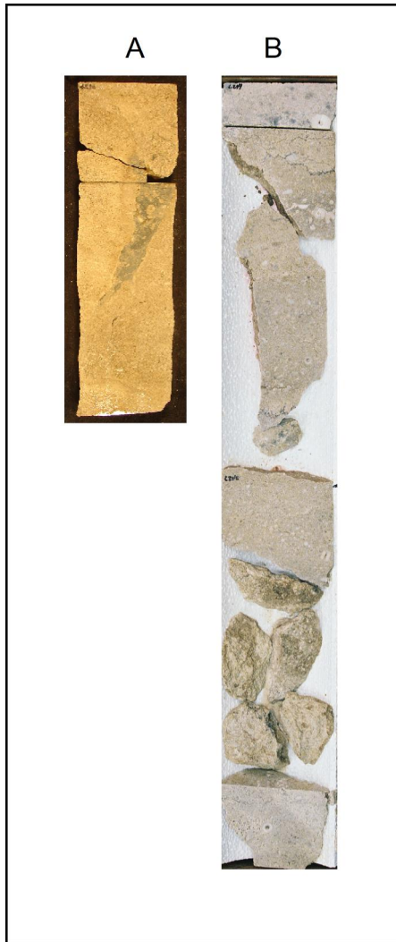
Figure 17. Core photographs showing evidence of karsting in injection interval at 6230–6241 ft log depth. (A) Wide extension fracture filled with breccia at 6232 ft core depth. (B) Broken core and rubble at 6241–6242 ft core depth.
