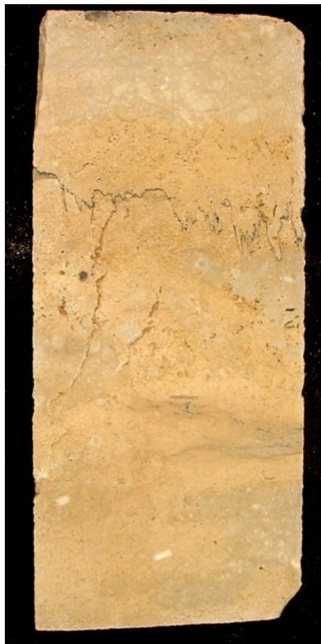
Figure 8. Example of tension-gash fractures associated with stylolites; 6215 ft core depth.
