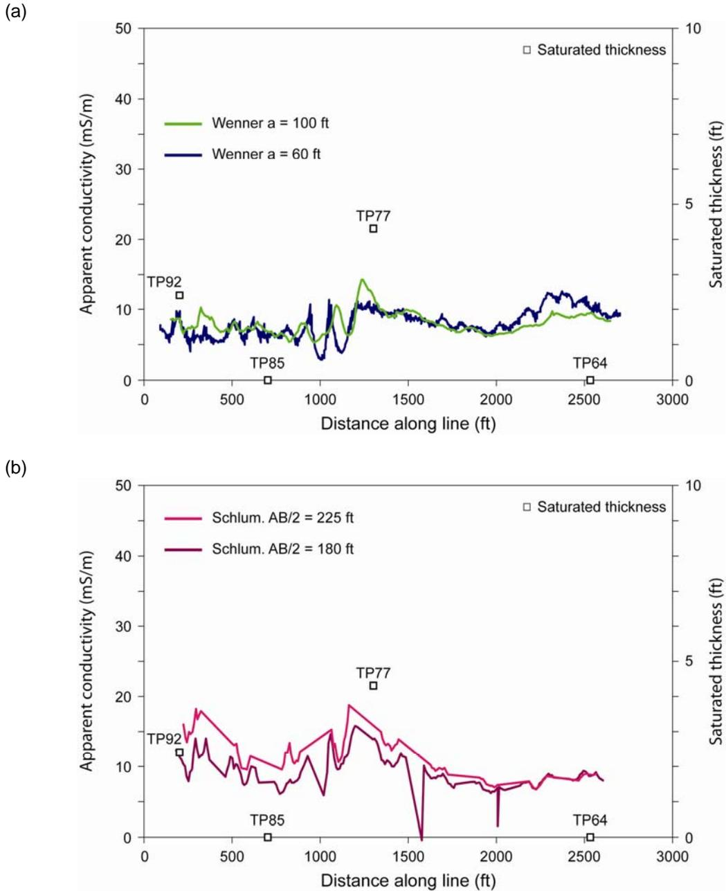
Figure 5. Comparison of apparent conductivity and water saturation along Line D. (a) Wenner 60- and 100-ft a-spacing data from Technos 2008c. (b) Schlumberger 180- and 225-ft AB/2 spacing data from raw resistivity data files.
