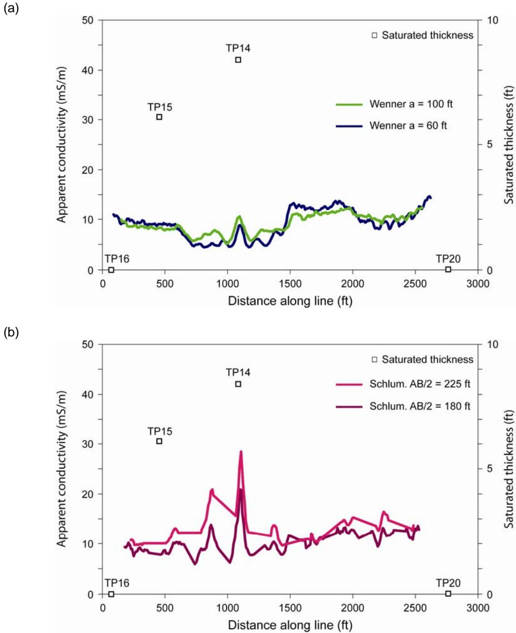
Figure 3. Comparison of apparent conductivity and water saturation along Line B. (a) Wenner 60- and 100-ft a-spacing data from Technos 2008c. (b) Schlumberger 180- and 225-ft AB/2 spacing data from raw resistivity data files.
