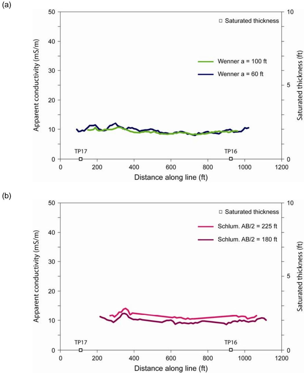
Figure 2. Comparison of apparent conductivity and water saturation along Line A. (a) Wenner 60- and 100-ft a-spacing data from Technos 2008c. (b) Schlumberger 180- and 225-ft AB/2 spacing data from raw resistivity data files.
