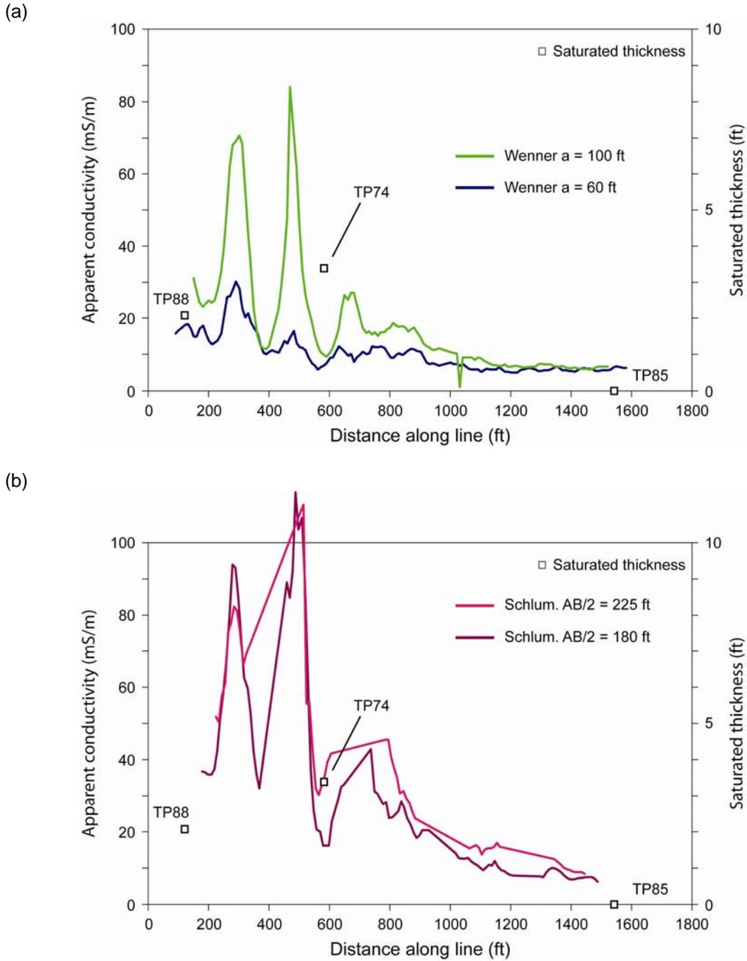
Figure 4. Comparison of apparent conductivity and water saturation along Line C. (a) Wenner 60- and 100-ft a-spacing data from Technos 2008c. (b) Schlumberger 180- and 225-ft AB/2 spacing data from raw resistivity data files.
