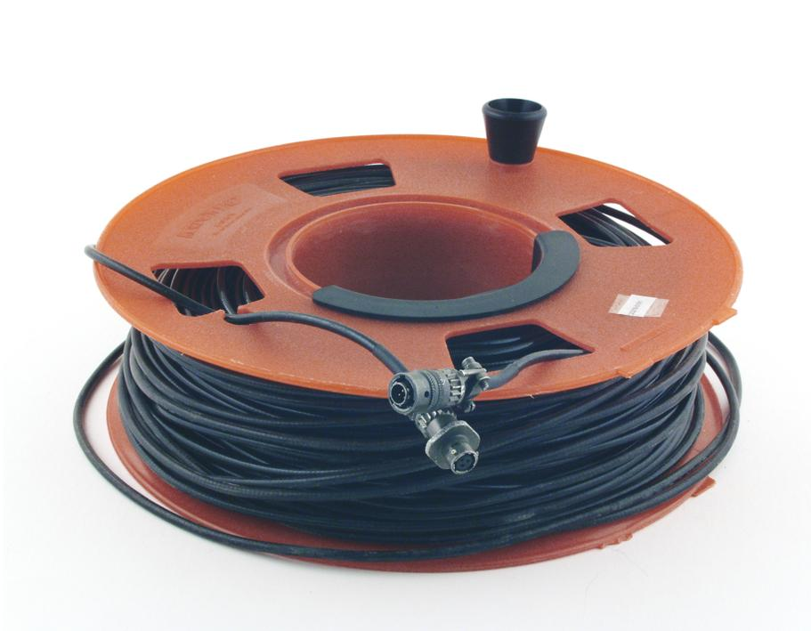
Figure 6. Trigger extension cable, a 100-m long cable connecting the seismograph (lower connector) with the trigger (upper connector).
