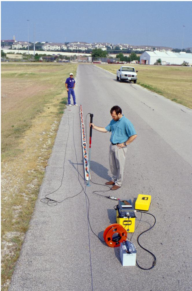
Figure 1. SRBA seismograph, geophone array, power supply, and seismic source deployed and ready to acquire data.
