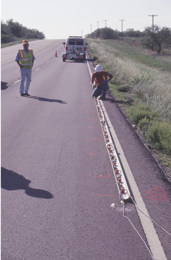
Figure 3. The geophone array, unfolded and deployed on asphalt pavement.
