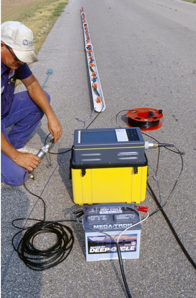
Figure 4. Geometrics SmartSeis seismograph. Power cable, geophone array cable, and trigger link spool cable are attached to seismograph.
