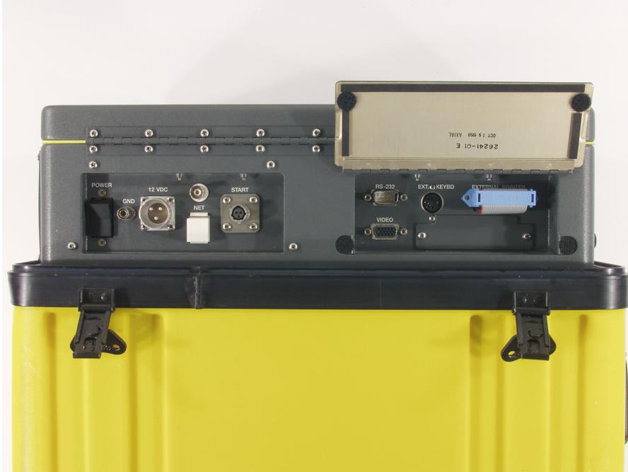
Figure 5. Back panel of the Geometrics SmartSeis seismograph. At left are the on/off switch, the power receptacle, and the trigger receptacle. At right are the RS-232 serial port, the external video port, and the external keyboard port.
