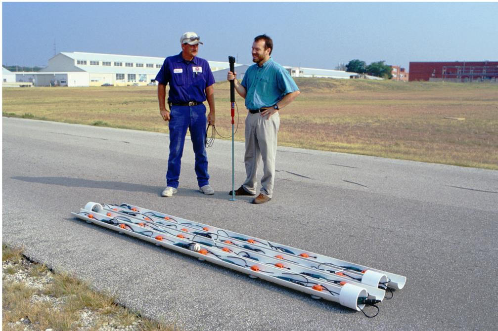
Figure 9. Geophone array folded for transport.
