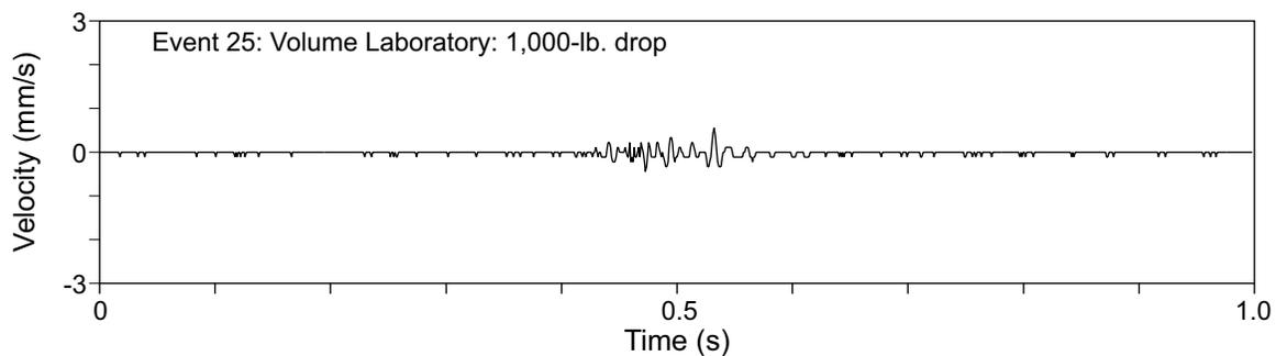
Figure 10. Vertical ground speed recorded over a 1-s interval in the VL during the lowering of a 1,000-lb weight onto the floor in the LML.
