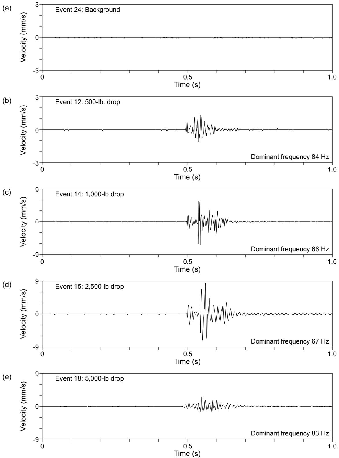
Figure 7. Vertical ground speed recorded over a 1-s interval in the LML (a) during normal laboratory activities but no hoist operation and, (b) through (e), during the lowering of 500-, 1,000-, 2,500-, and 5,000-lb weights onto the floor.
