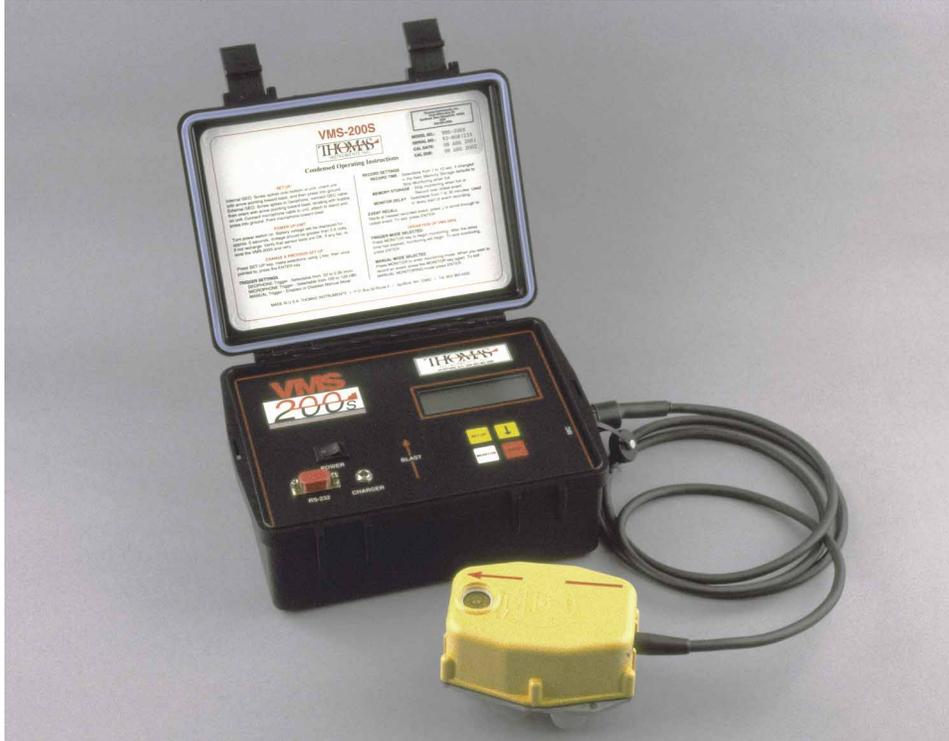
Figure 2. Photograph of the VMS-200S Vibration Monitoring System manufactured by Thomas Instruments Inc. This instrument was used to measure ground motion inside and outside the Metrology Laboratory. Photograph by David M. Stephens.
