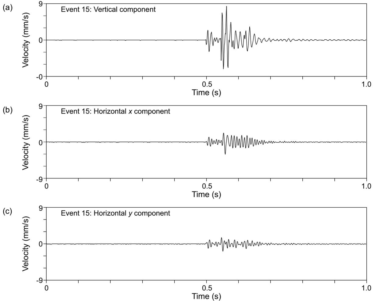
Figure 8. Vertical and horizontal ground speeds recorded over a 1-s interval in the LML during the lowering of a 2,500-lb weight onto the floor.
