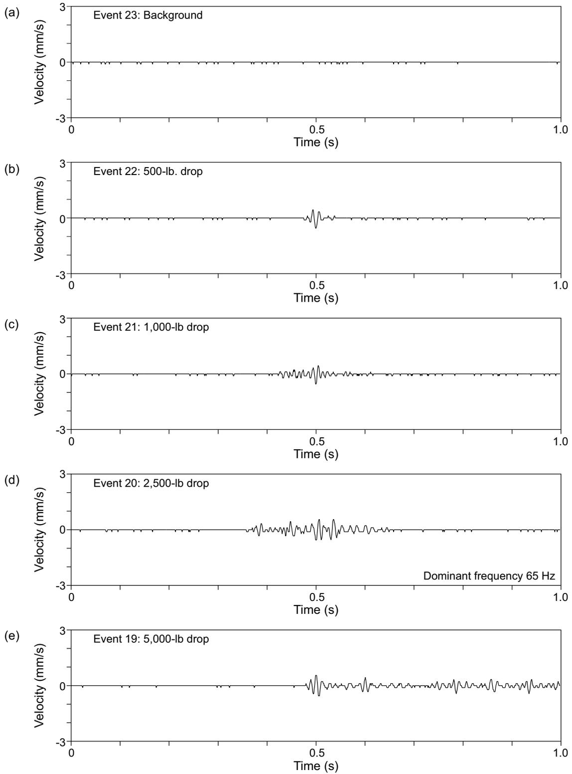
Figure 9. Vertical ground speed recorded over a 1-s interval in the SML (a) during normal laboratory activities but no crane operation and, (b) through (e), during the lowering of 500-, 1,000-, 2,500-, and 5,000-lb weights onto the floor in the LML.
