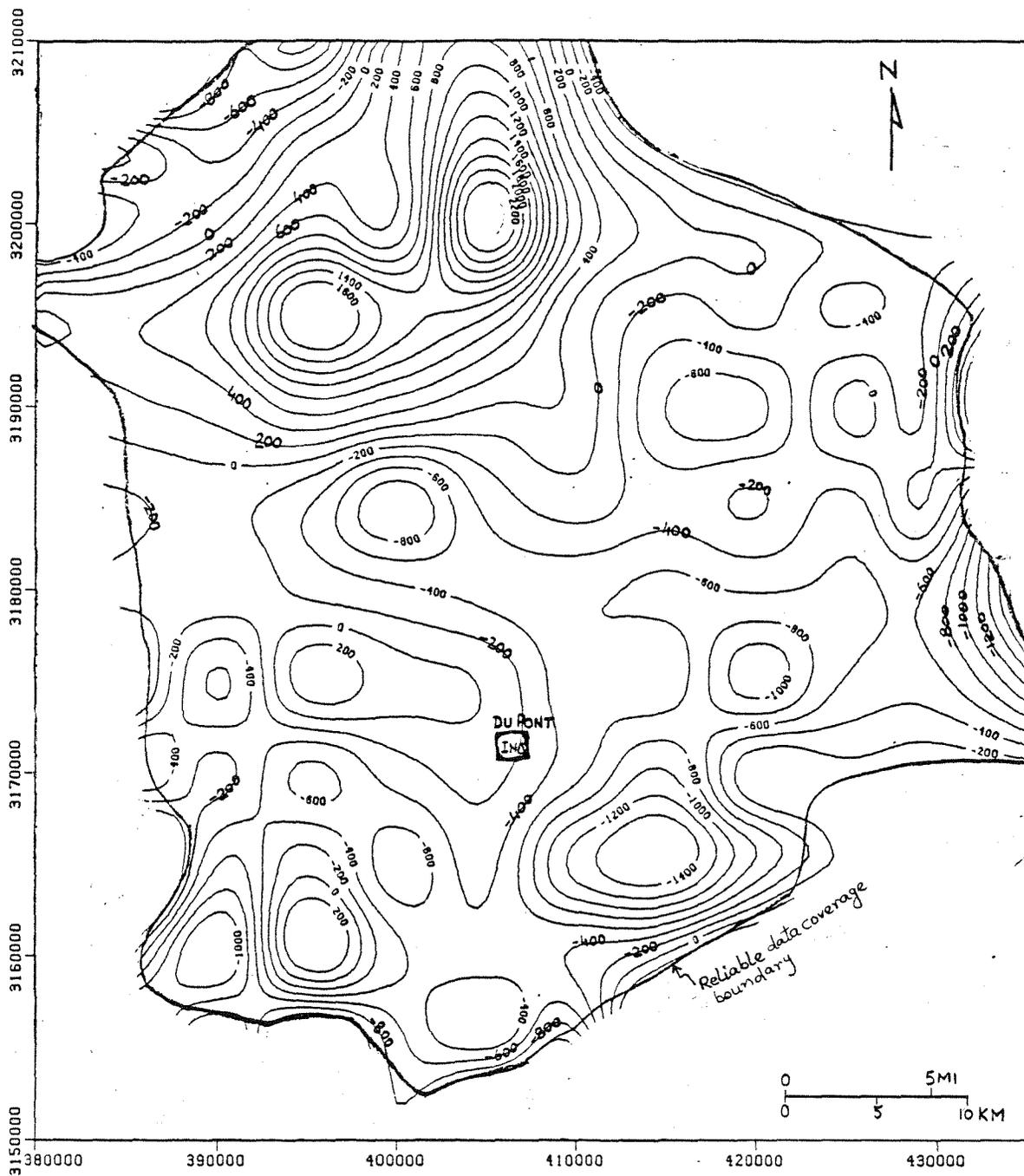
Figure 14. Potentiometric surface, 4000-6000 ft slice, Victoria Co., all formations, all classes, 1965-85 data. Includes formation pressure at Du Pont facility.
