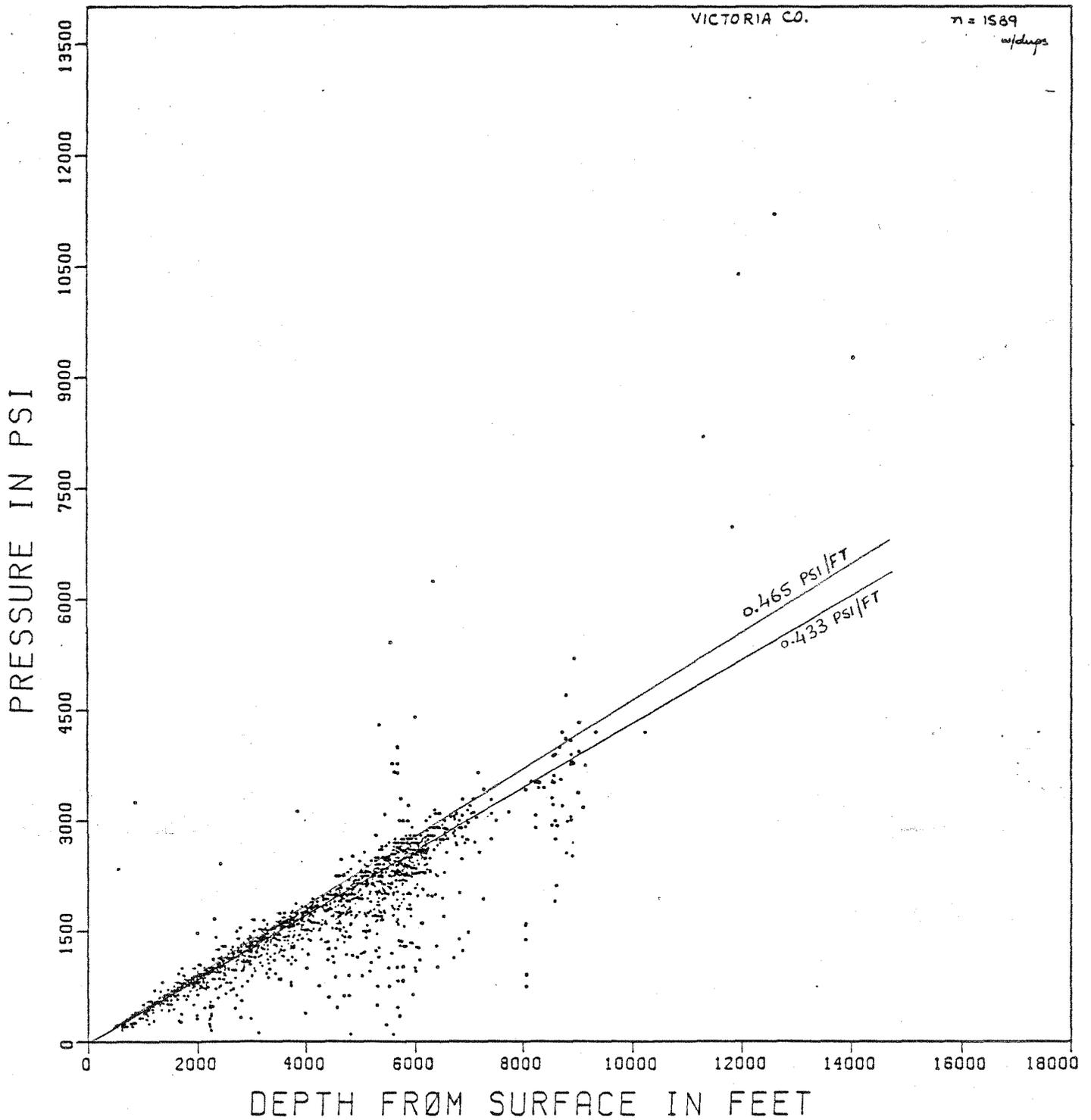
Figure 9. Pressure-depth diagram for Victoria County data.
