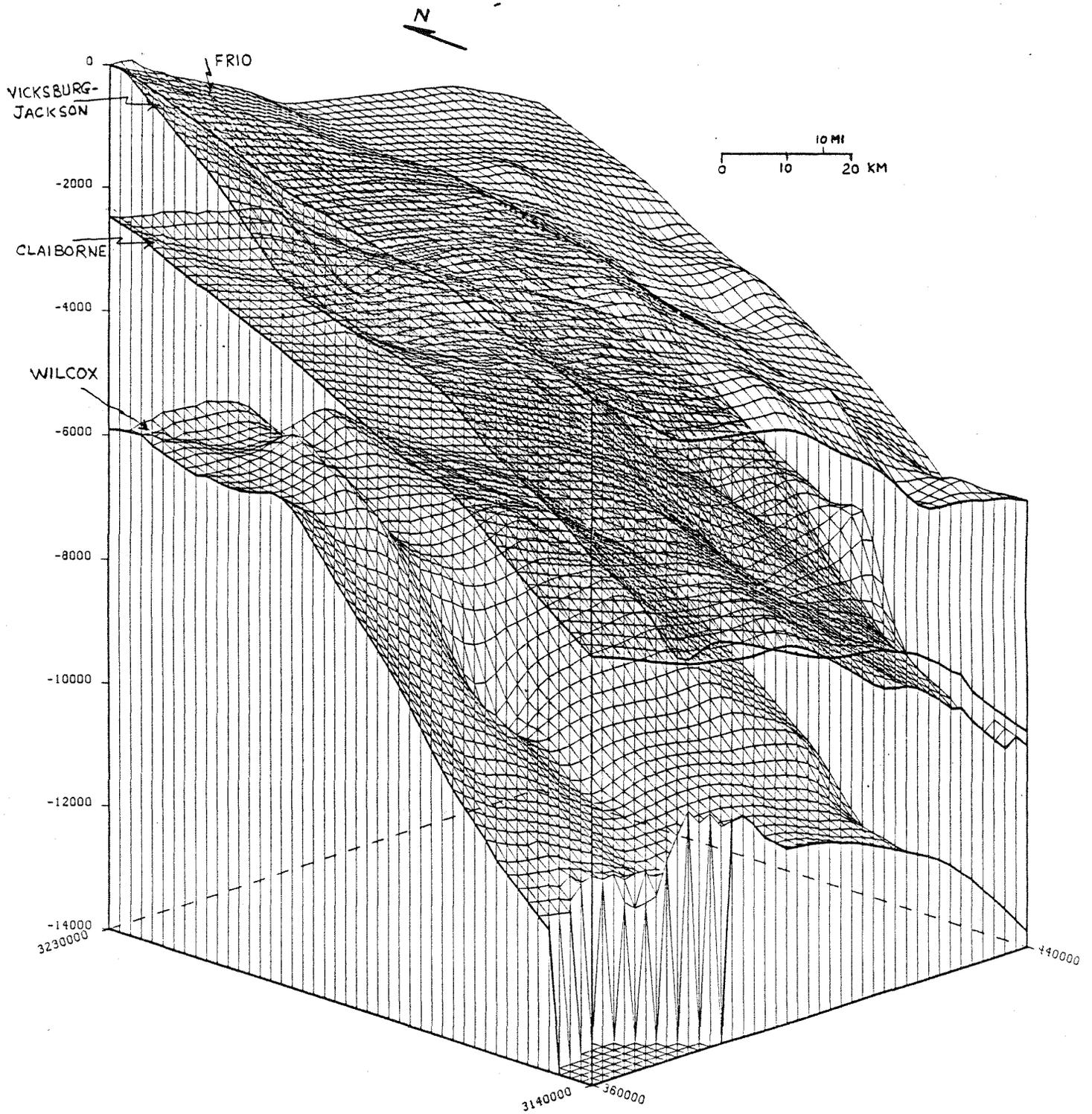
Figure 10. Isometric view of structure tops, Tertiary system, Victoria County (tops of Frio, Vicksburg-Jackson, Claiborne, and Wilcox Formations).
