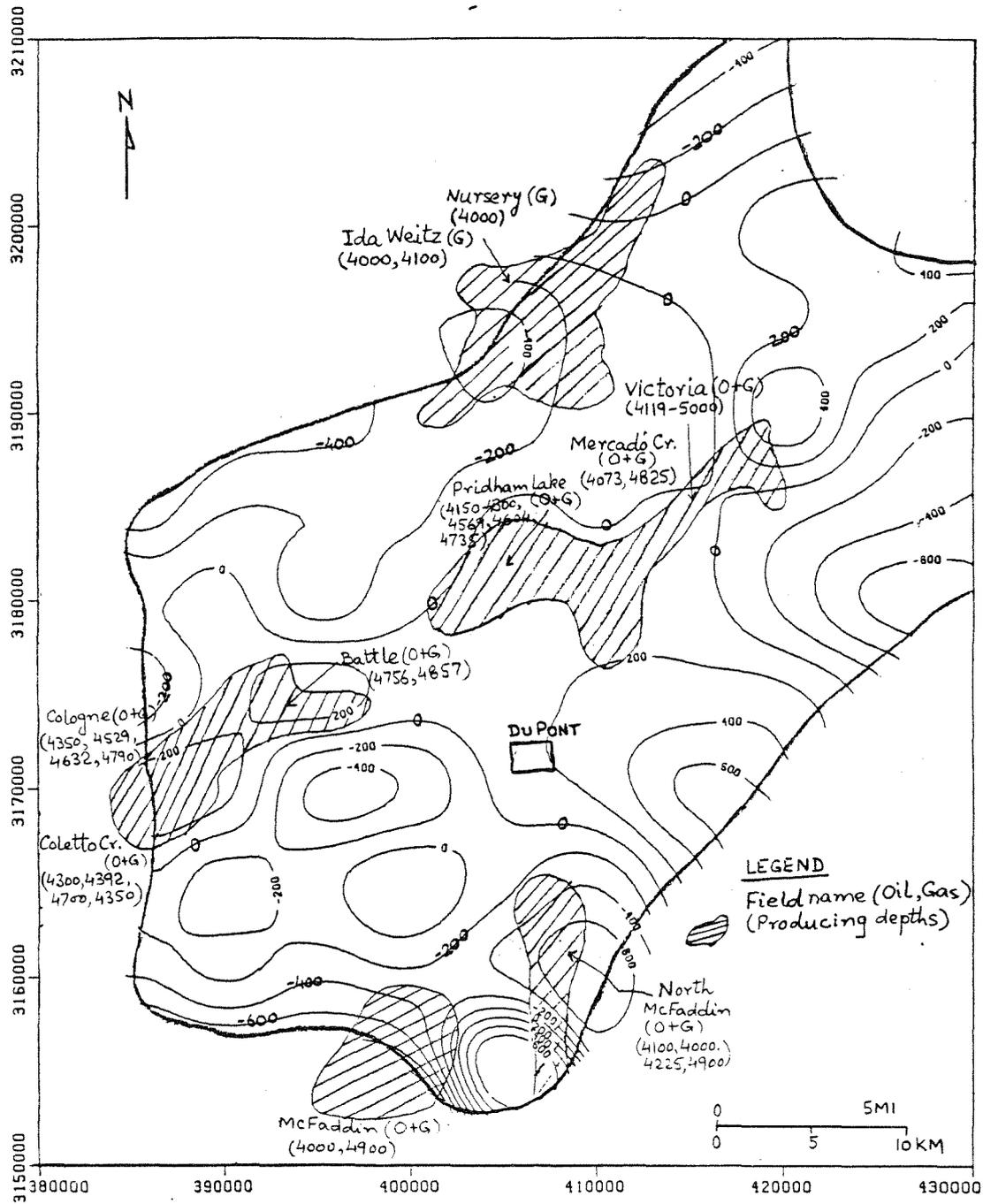
Figure 16. Potentiometric surface, 4000-4900 ft slice, Victoria Co., all formations, all classes, data for all years. Includes formation pressure at Du Pont facility.
