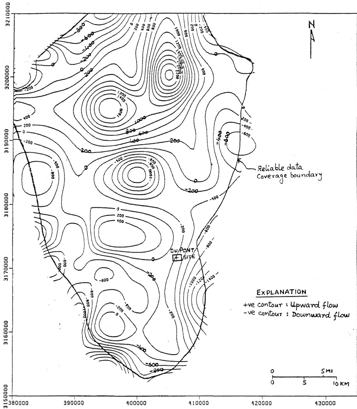
Figure 18. Residual potential surface, 4000-6000 ft minus 0-2000 ft slice, Victoria Co., all formations, all classes, 1965-85 data. Positive contours indicate upward flow, and negative contours indicate downward flow.
