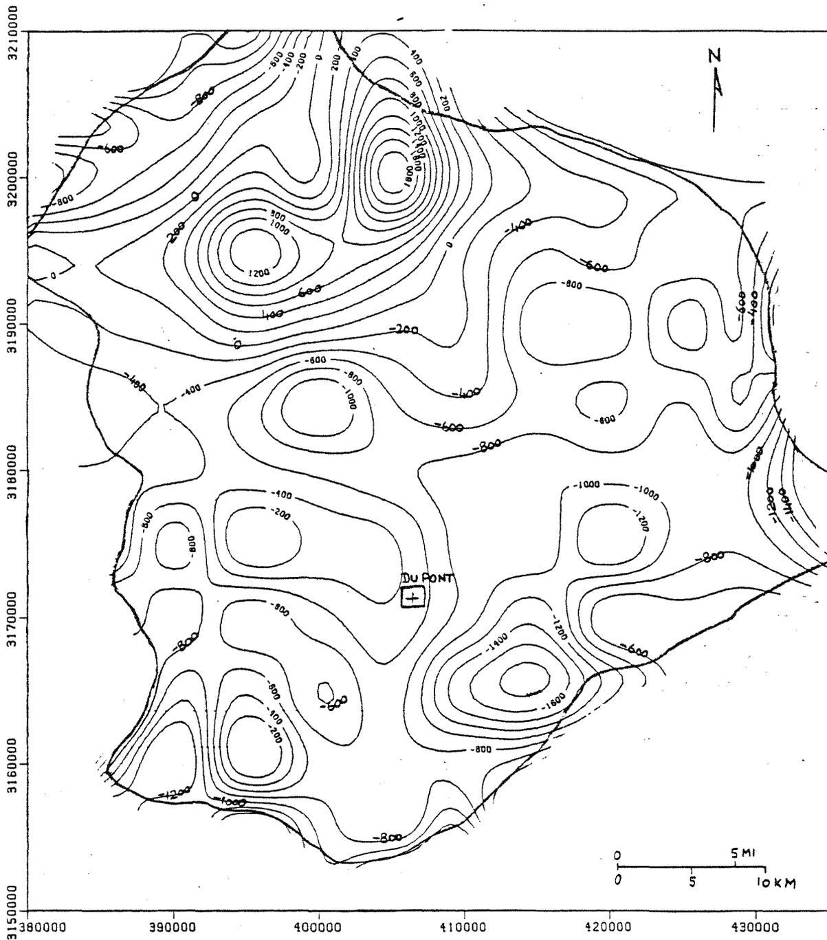
Figure 22. Potentiometric surface, 4000-6000 ft slice, Victoria Co., with 0.465 gradient, all formations, all classes, 1965-85 data. Includes formation pressure at Du Pont facility.
