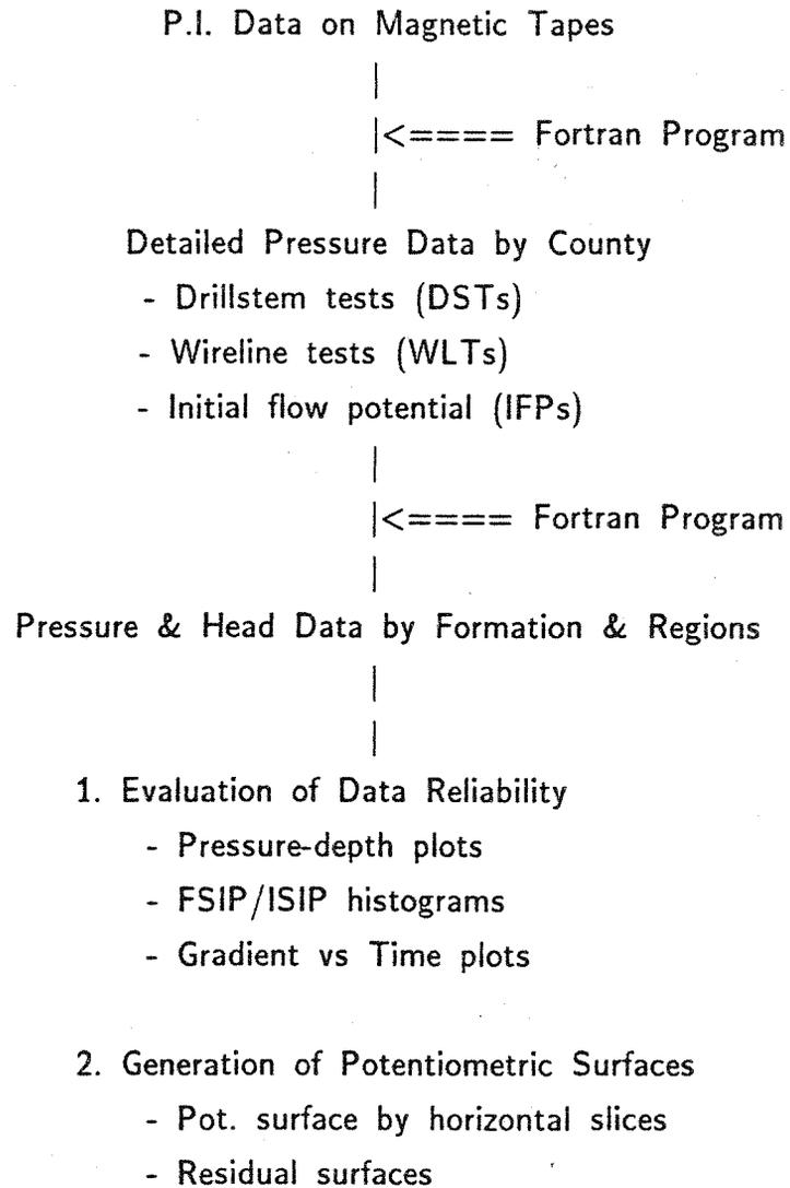
Figure 5. Schematic flow diagram for data processing.
