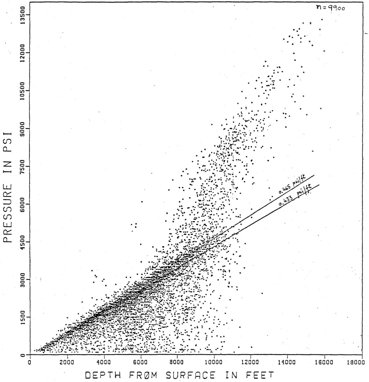
Figure 6. Pressure-depth diagram for Frio regions B and C data.
