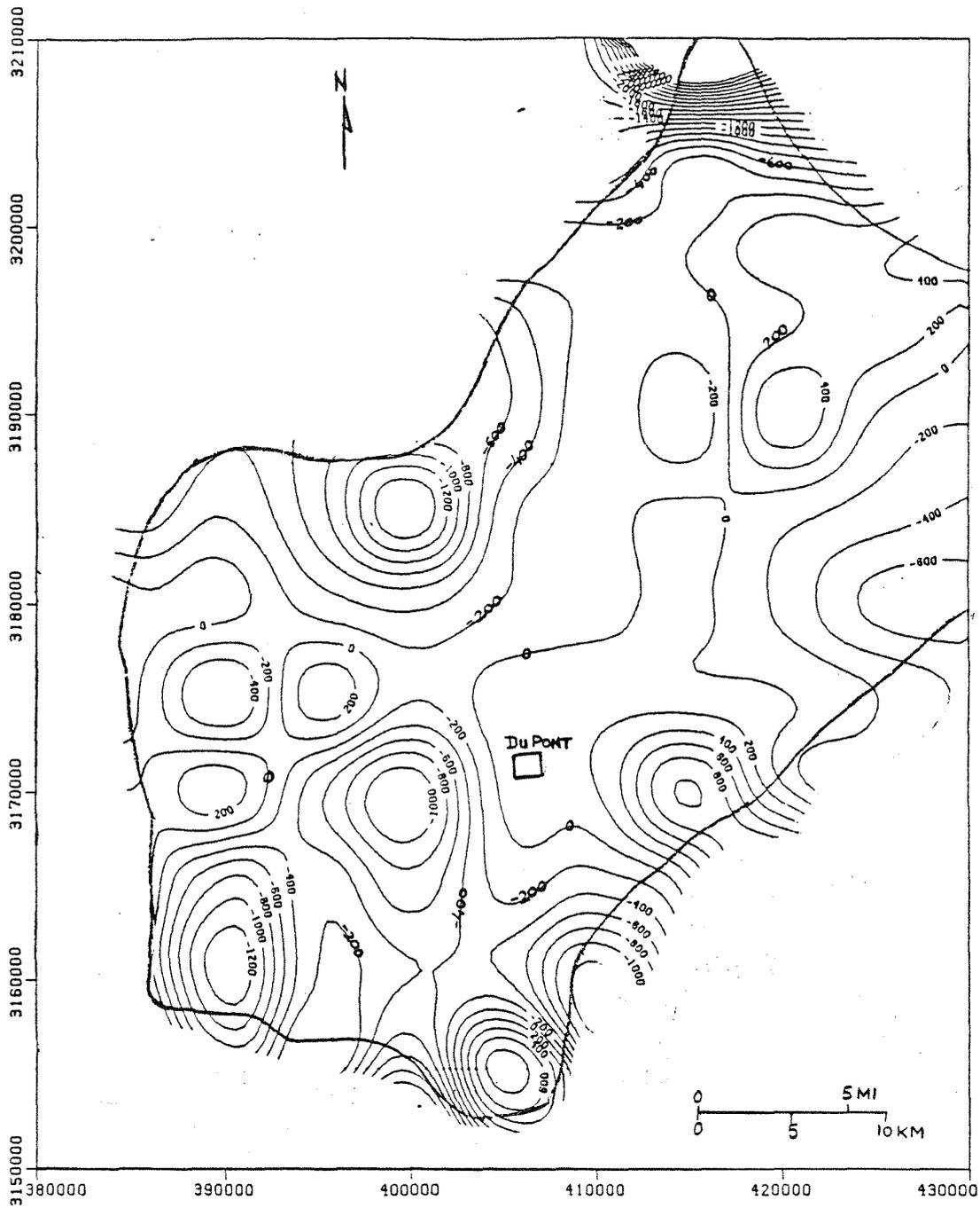
Figure 21. Potentiometric surface, 4000-4900 ft slice, Victoria Co., includes extreme heads, all classes, all formations, all years. Includes formation pressure at Du Pont facility.
