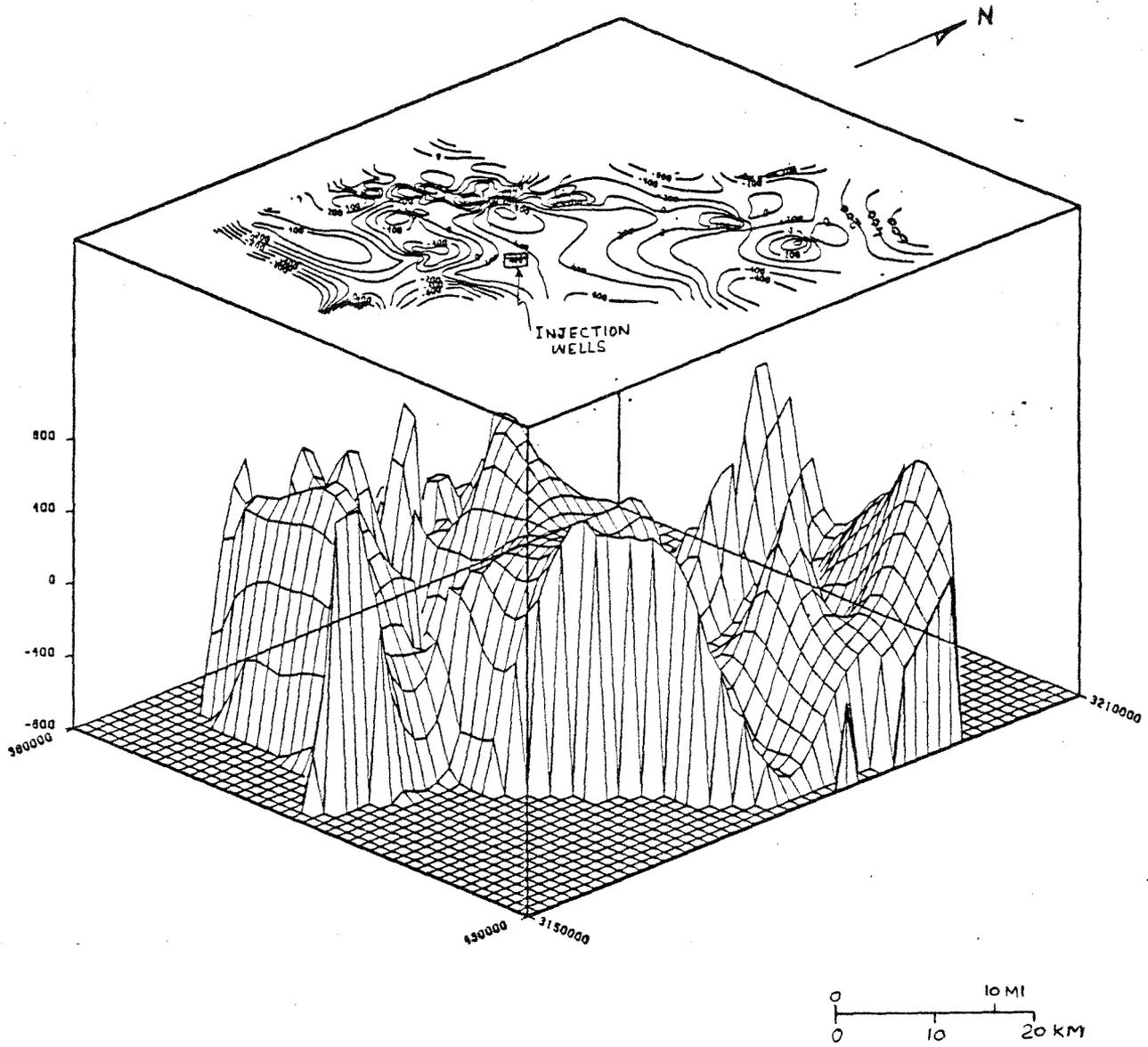
Figure 17. Isometric view of potentiometric surface, 4000-4900 ft slice, Victoria Co., all formations, all classes, data for all years. Includes formation pressure at Du Pont facility.
