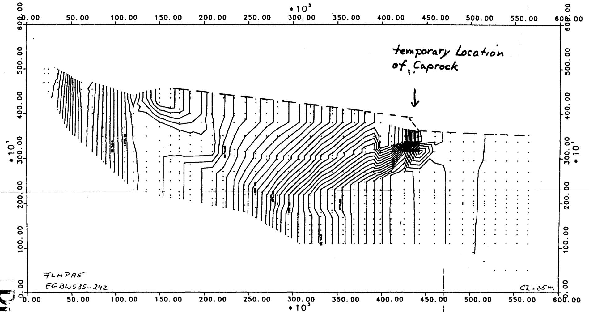
Figure 28. Hydraulic head distribution from Simulation P-1 showing possible effects of erosional unloading conditions 800,000 years after gradual retreat (18 cm/yr) of the Caprock Escarpment from the eastern boundary of the model. The unloading causes local, temporary underpressuring beneath the Caprock Escarpment.
