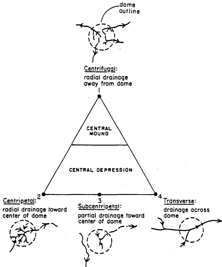
Figure 4. Qualitative classification of drainage systems above domes: four ideal types as a guide to relative movement of the land surface. Toroidal drainage is not shown.
