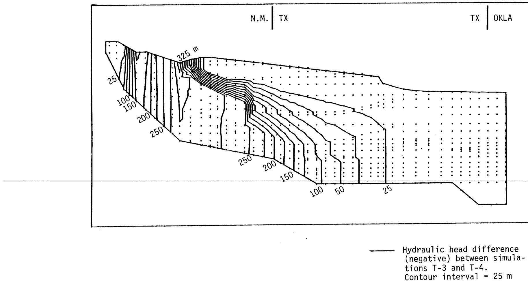
Figure 8. Difference in hydraulic heads before and after Pecos River erosion.
