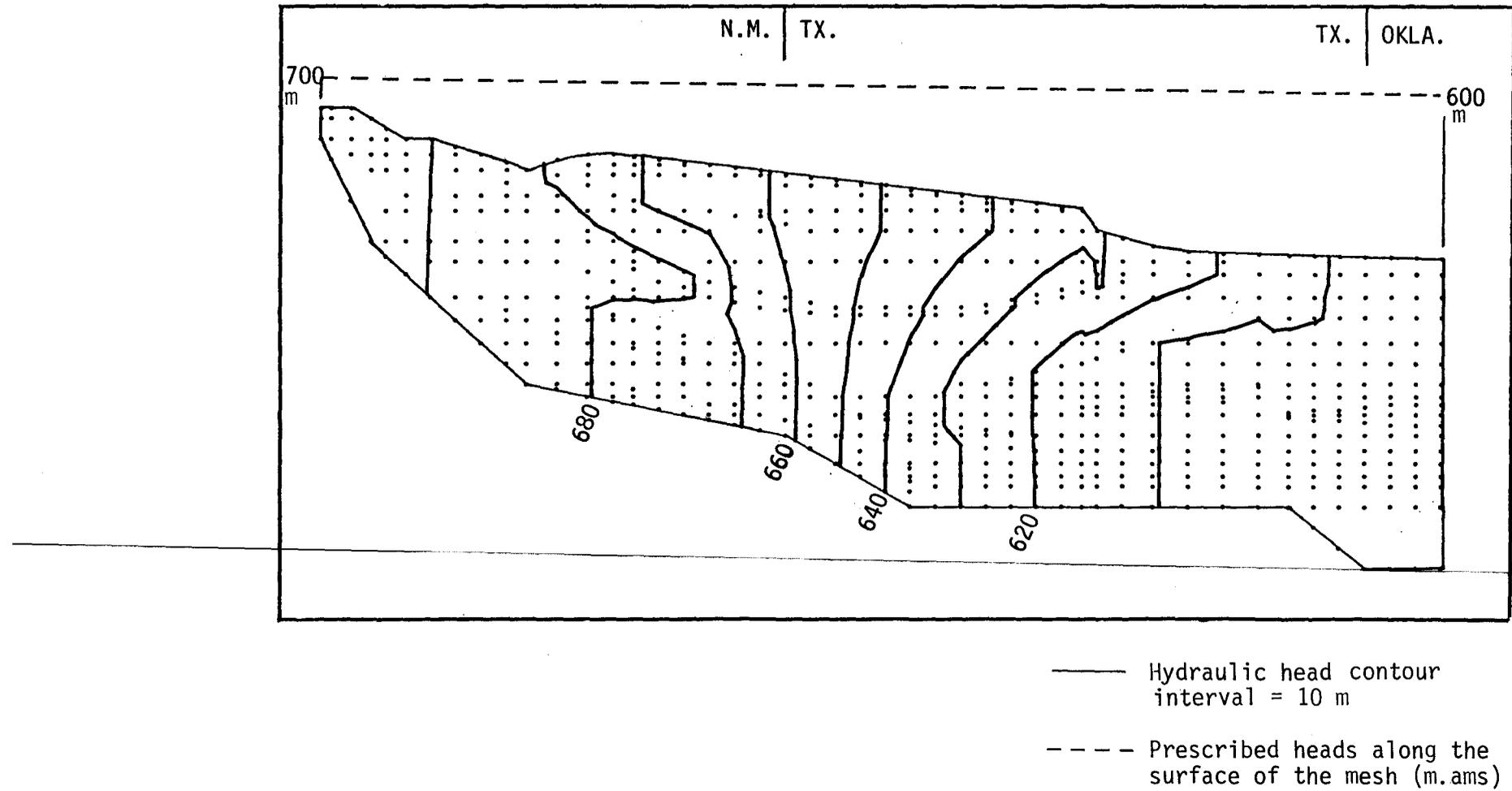
Figure 4. Simulation T-1 of computed hydraulic head distribution with hydraulic conductivities from Table 2. Hydraulic head distribution represents the hypothetical pre-uplift hydrodynamic conditions assuming an overall hydraulic gradient across the surface of the model of 100 m.
