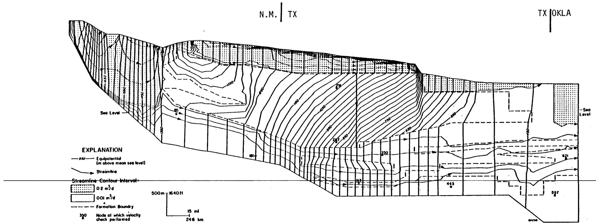
Figure 11. Steady-state hydraulic head distribution based on simulation A-2 (Senger and Fogg, 1984) which was considered to be the most realistic representation of the hydrologic flow regime in the Palo Duro Basin.
