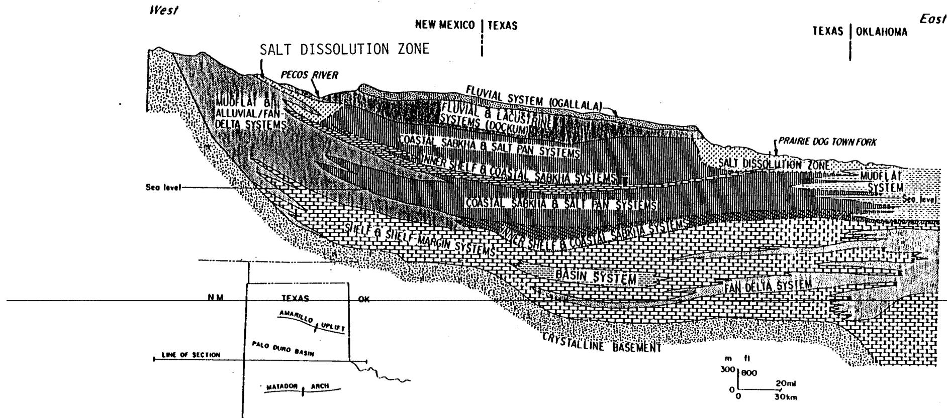
Figure 2. Regional east-west cross section illustrating spatial relationships of the major depositional systems in the Palo Duro Basin (after Bassett and others, 1981).
