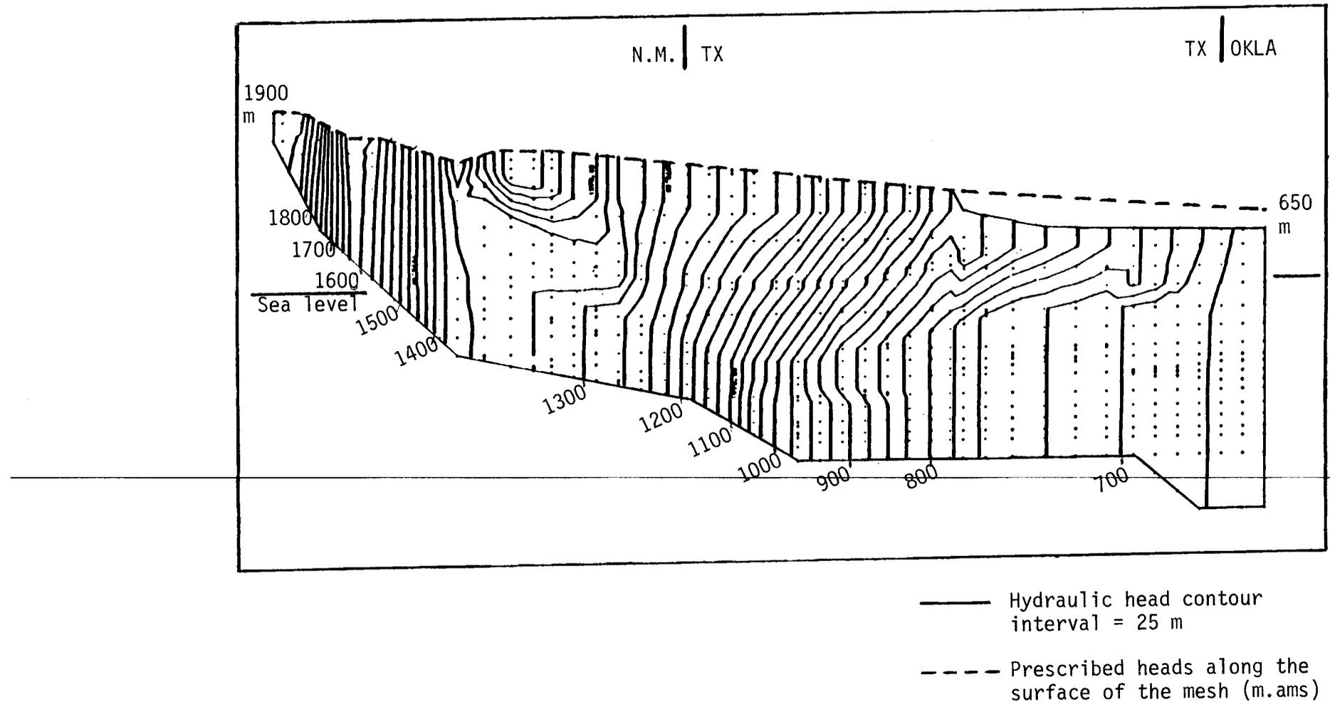
Figure 7. Simulation T-4 of computed hydraulic head distribution representing hydrodynamic conditions 5 million years after the onset of the Pecos valley erosion. Hydraulic heads at the boundary nodes of the area were gradually reduced during the first 4 million years to a level corresponding to the approximate valley topography. Initial conditions are the computed heads from simulation T-3.
