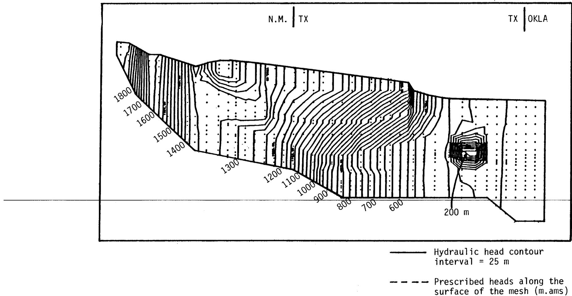
Figure 12. Simulation H-1 of computed hydraulic head distribution representing the hydrodynamic conditions as a result of hydrocarbon production 100 years after the beginning of gradual reservoir pressure decline.
