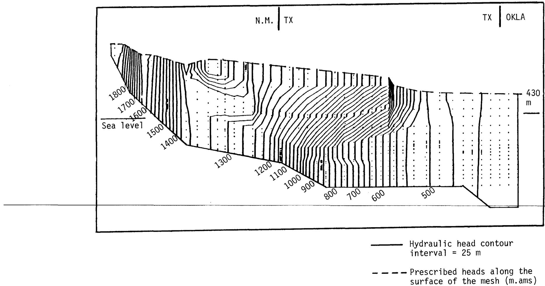
Figure 9. Simulation T-5 of computed hydraulic head distribution representing hydrodynamic conditions 1.1 million years after the gradual retreat (18 cm/yr) of the Caprock Escarpment starting at the eastern boundary of the model. Initial conditions are the computed heads from simulation T-4.
