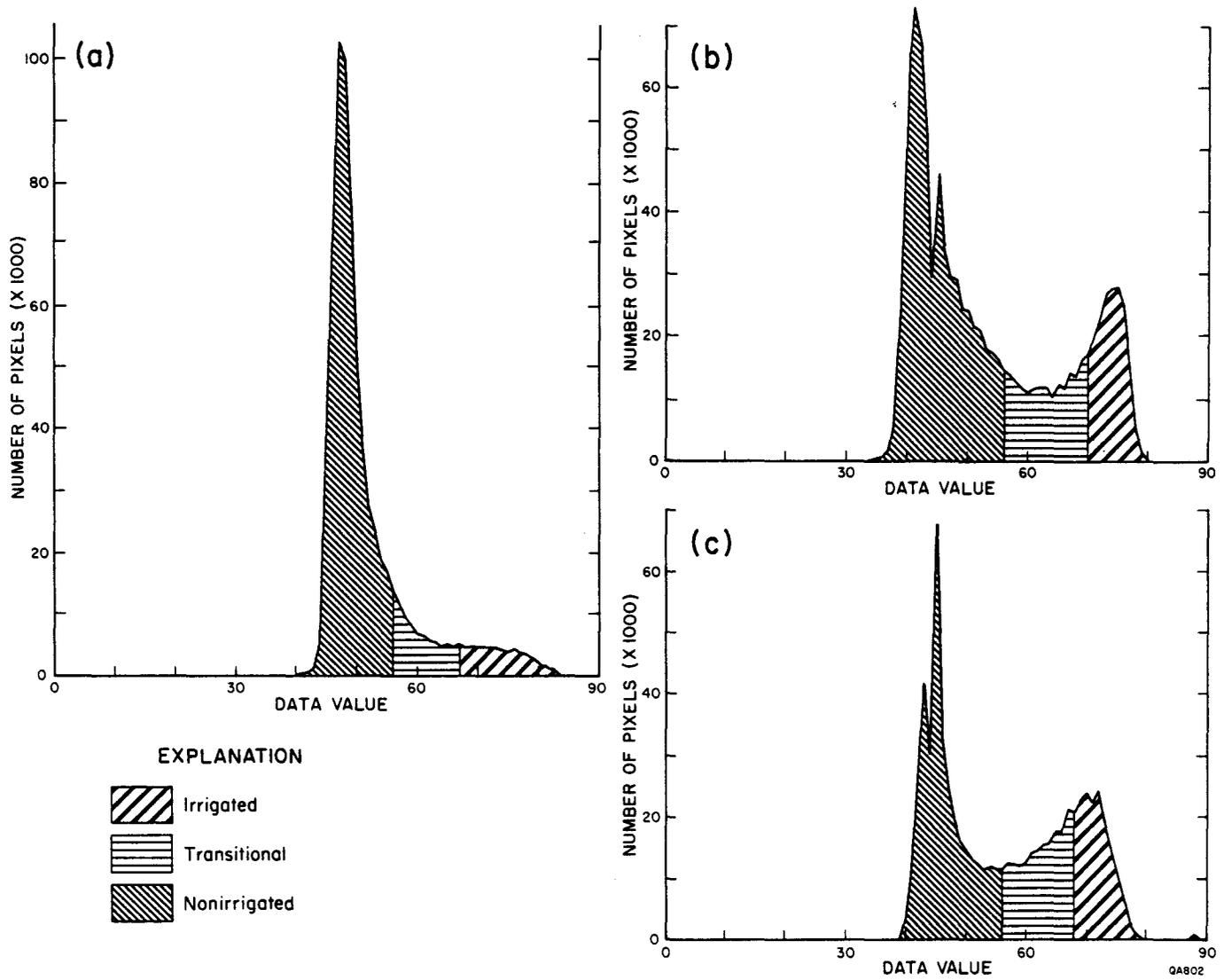
Figure 4. Histograms of band ratio data values from Landsat data for (a) May 13, 1980, (b) July 15, 1980, and (c) August 29, 1980. Band ratio is (B7/B5). Initial image analysis divided data values into three categories, as shown. Final image analysis reclassified transitional data values as nonirrigated.
