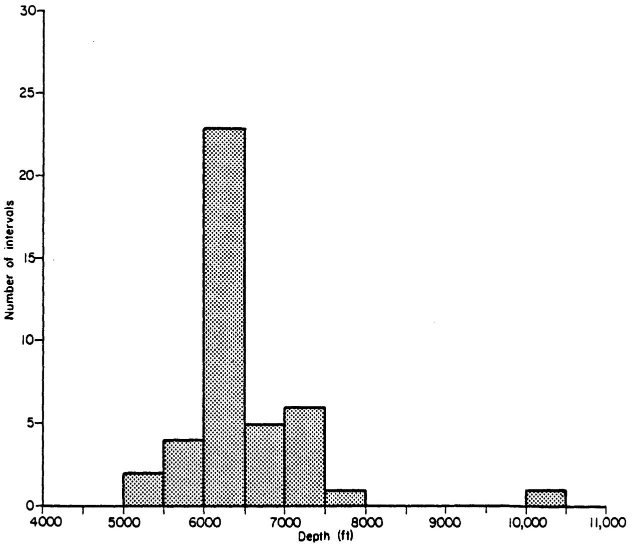
Figure 96. Depth to top of perforated interval for 43 gas well completions in the First Frontier, Frontier Formation, Greater Green River Basin.
