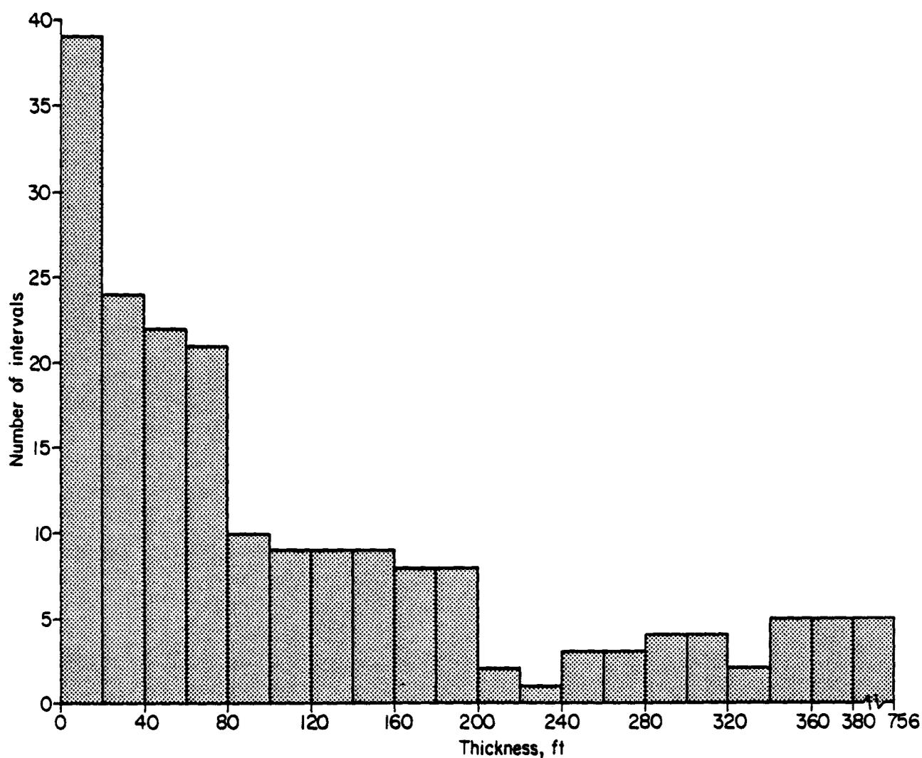
Figure 95. Thickness of gross perforated interval for 189 gas well completions in the Second Frontier of the Frontier Formation, Greater Green River Basin.
