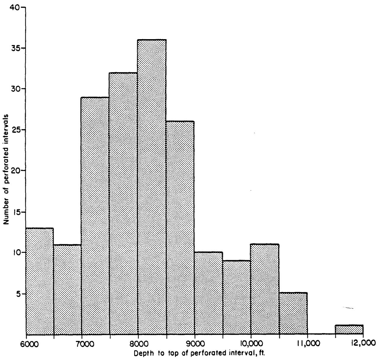
Figure 28. Depth to top of perforations for 191 gas wells completed in the Travis Peak Formation .
