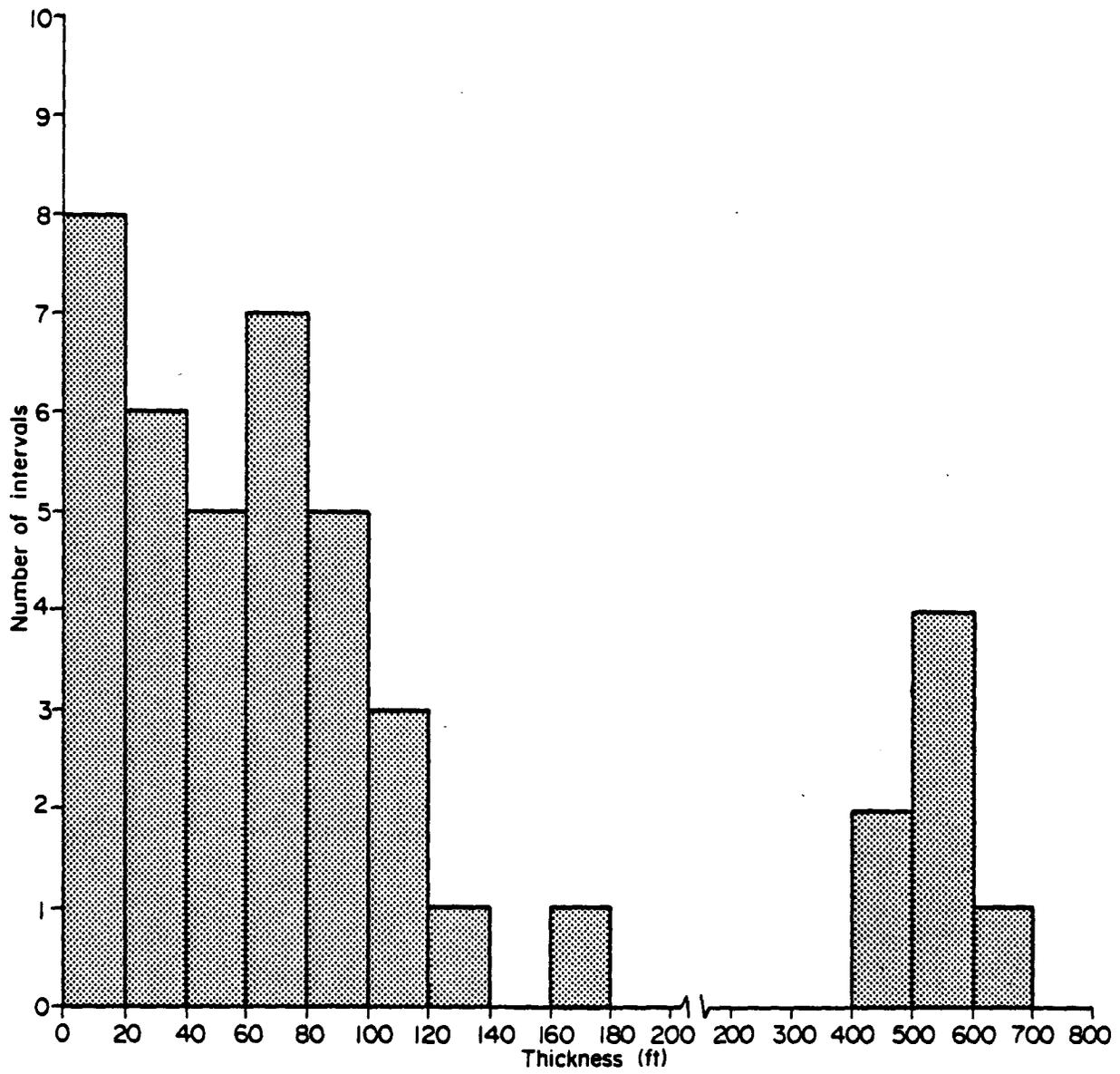
Figure 97. Thickness of gross perforated interval for 43 gas well completions in the First Frontier, Greater Green River Basin.
