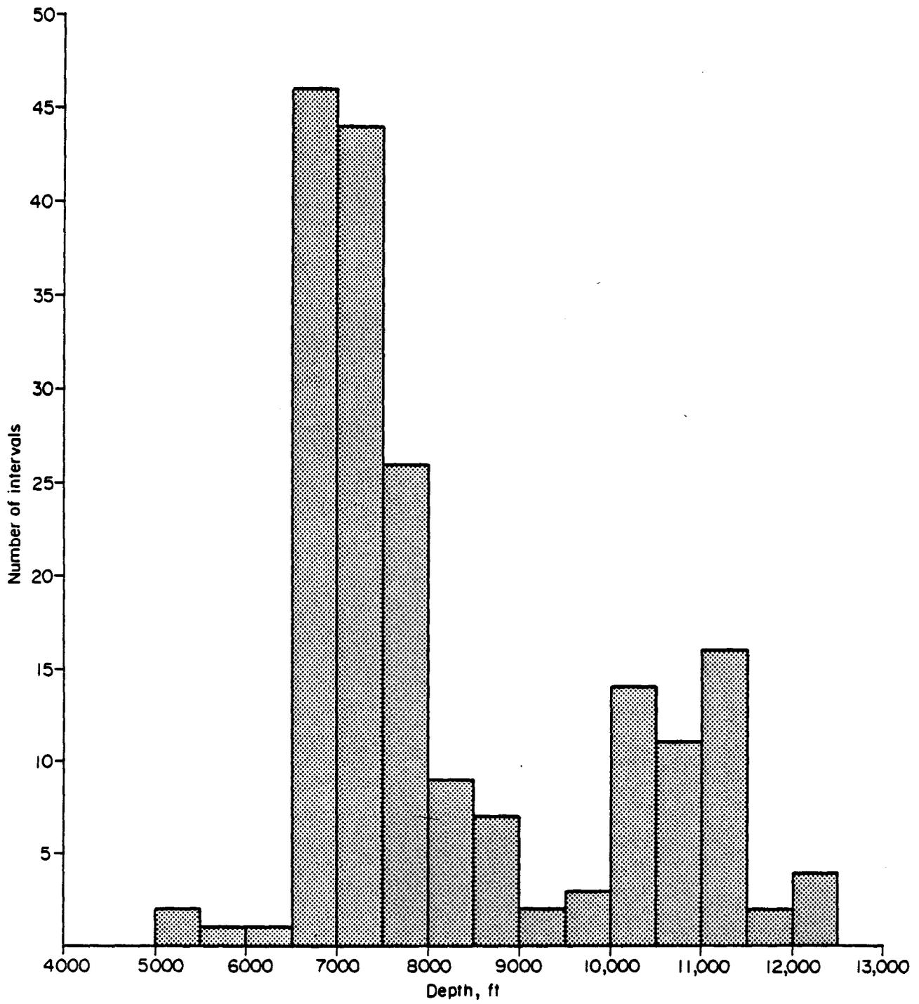
Figure 94. Depth to top of perforated interval for 186 gas well completions in the Second Frontier of the Frontier Formation, Greater Green River Basin.
