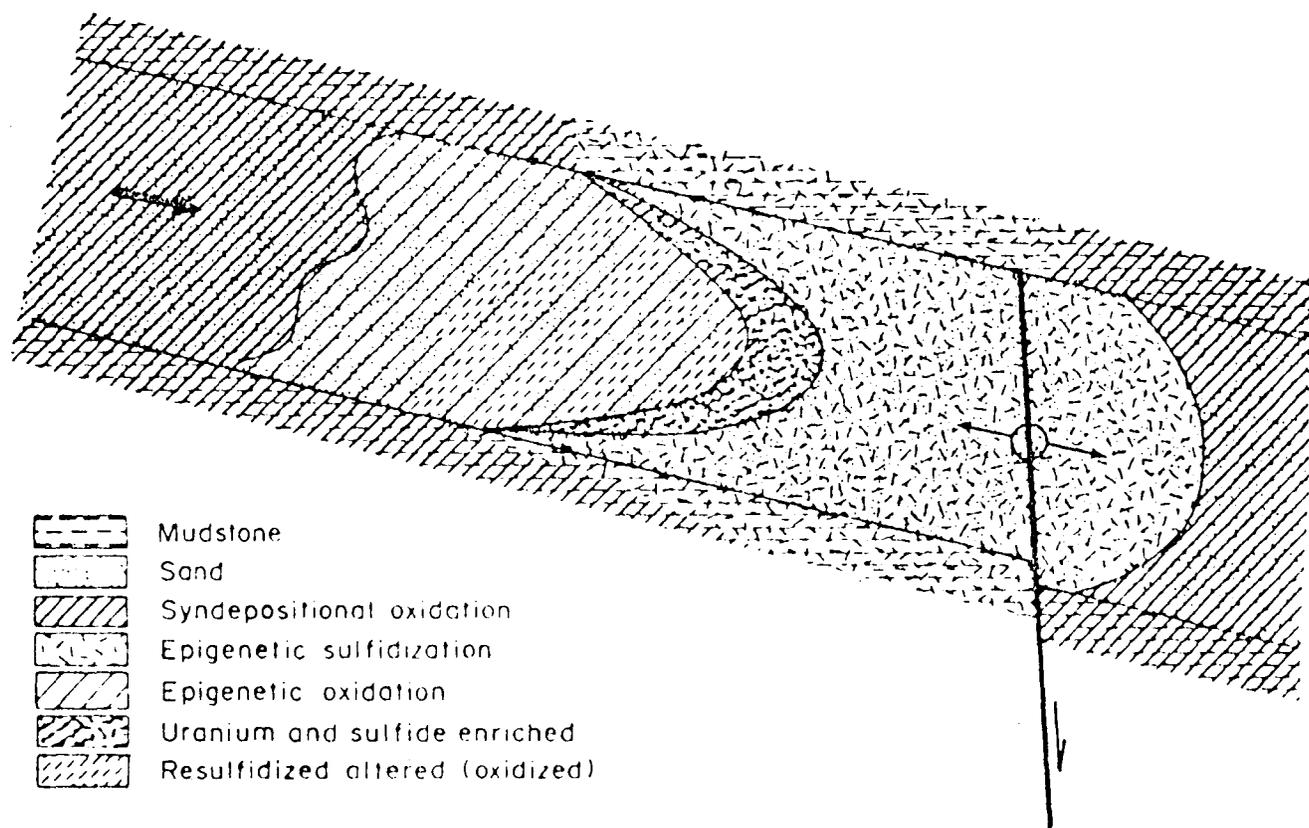
Figure 2. Diagrammatic alteration zonation produced by successive episodes of epigenetic sulfidic reduction, punctuated by mineralizing epigenetic oxidation within a syndepositionally oxidized aquifer.
