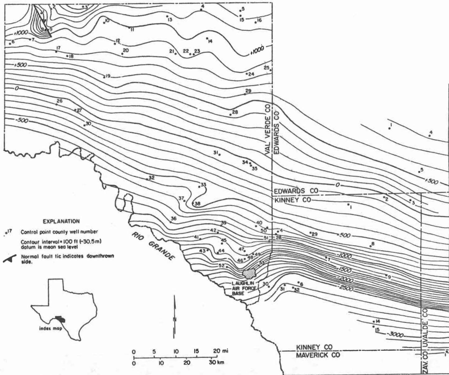
Figure H-16. Structure Contour Map on the Top of the Paleozoic Complex, Val Verde and Kinney Counties.
