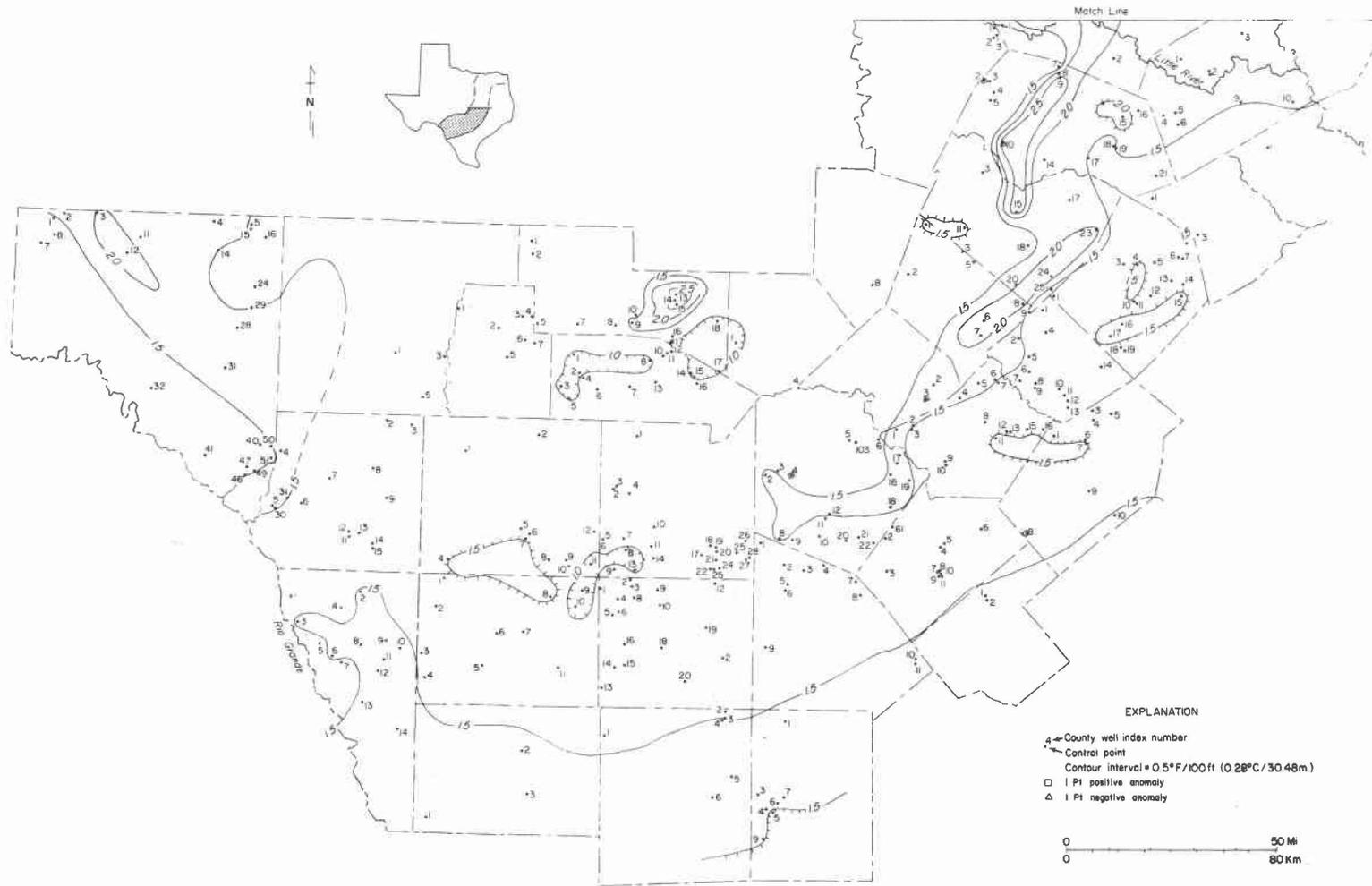
Figure H-2. Geothermal gradient map along southern part of Balcones/Ouachita trend.
