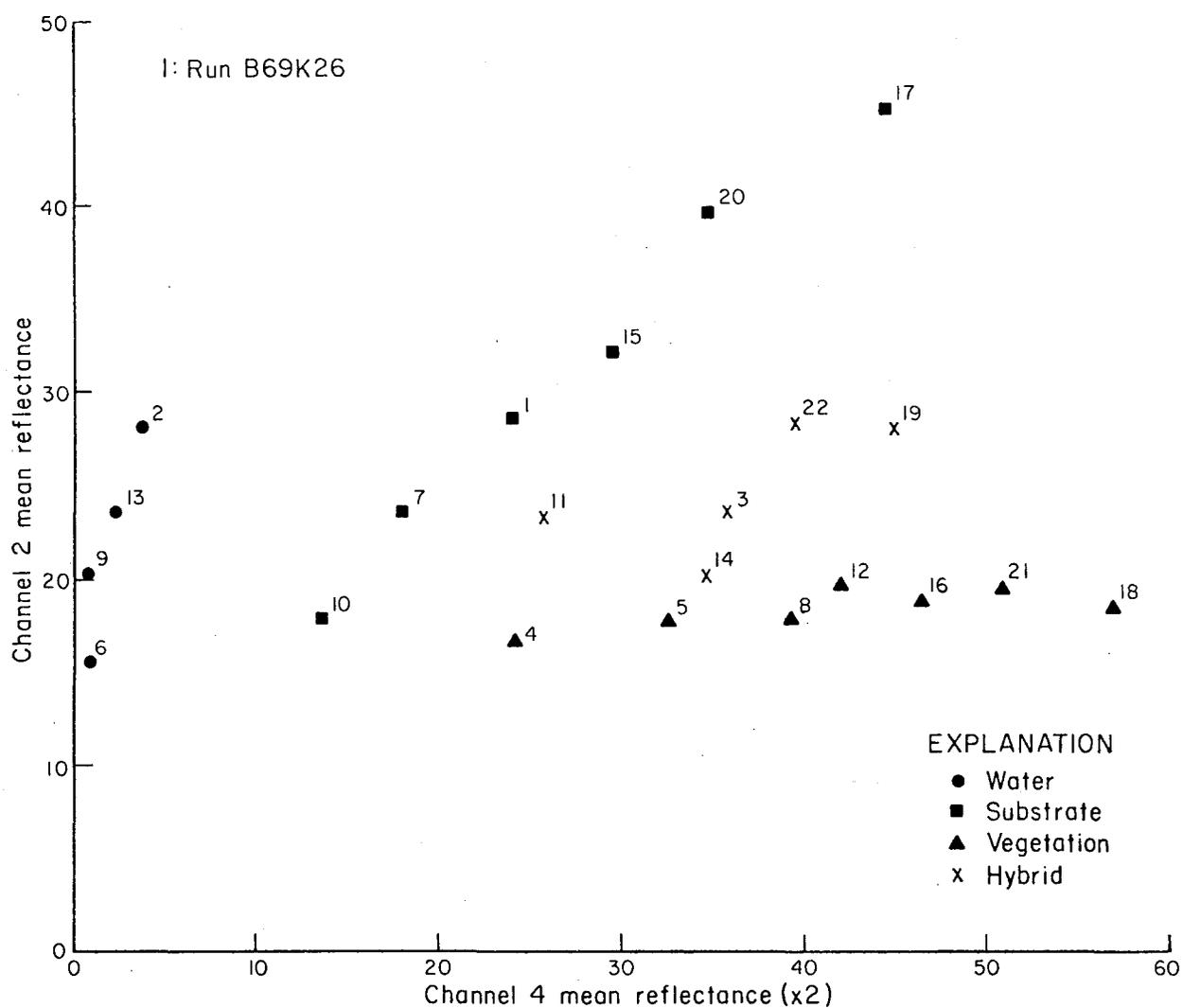
Figure 2. Plot of mean reflectance values in channel 2 and channel 4 for run B69K26. Channel 4 values are doubled. Four major types of clusters are seen here: water, substrate, vegetation, and hybrid. All but the hybrid clusters define lines radiating from a point near the y-axis. This and figures 4 through 6 are discussed in the text.
