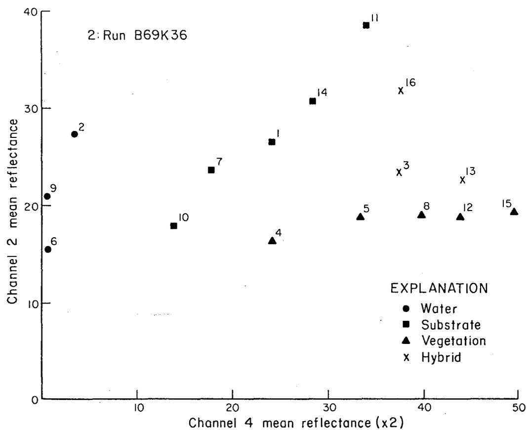
Figure 4. Plot of mean reflectance values in channel 2 and channel 4 for run B69K36. Channel 4 values are doubled. Four major types of clusters are seen here as in figure 2.
