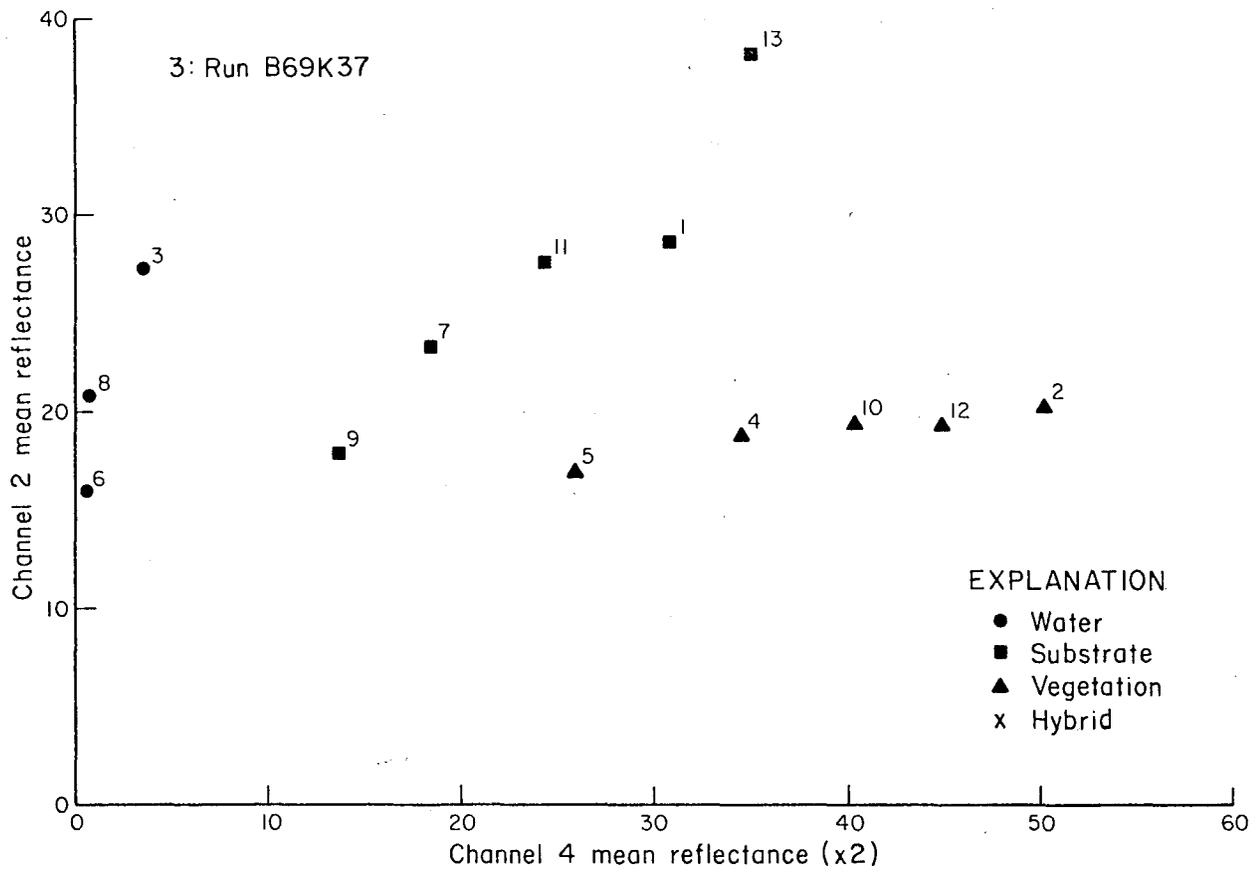
Figure 5. Plot of mean reflectance values in channel 2 and channel 4 for run B69K37. Channel 4 values are doubled. No hybrid clusters appear in this run.
