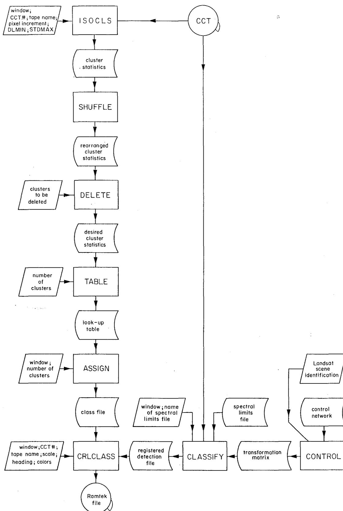
Figure 1. Flow diagram of Landsat data through classification programs to output on the Ramtek Graphics Display Terminal. Processing is usually interrupted after ISOCLS to examine cluster statistics and assign colors to clusters.
