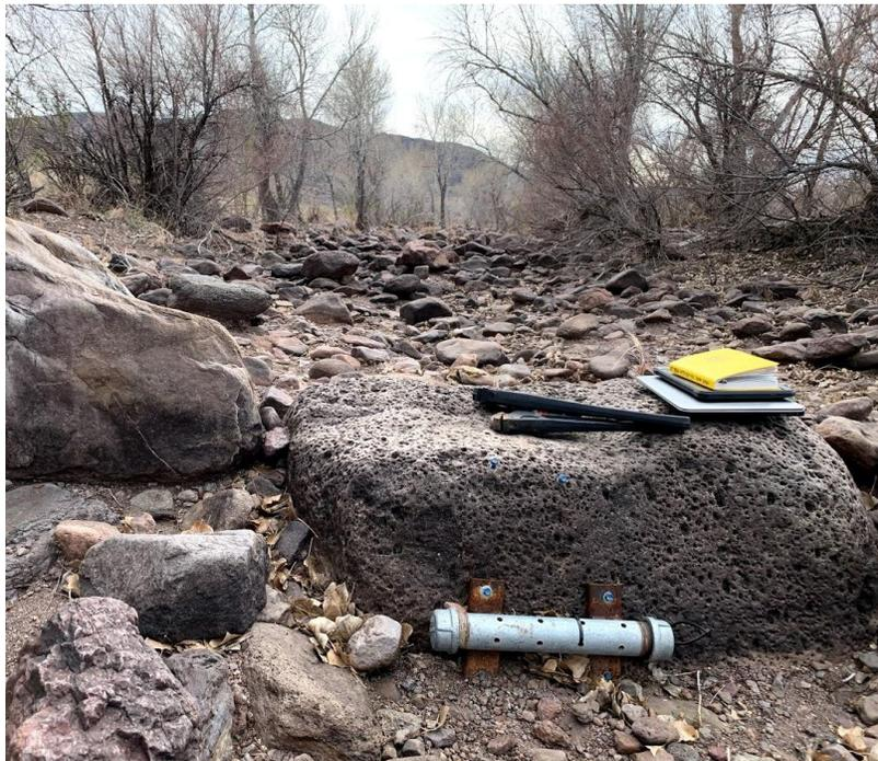
Photo 14. Limpia Lower Stream RuggedTroll on Leoncita Ranch, Limpia Pasture: upstream view of logger in pipe-housing
