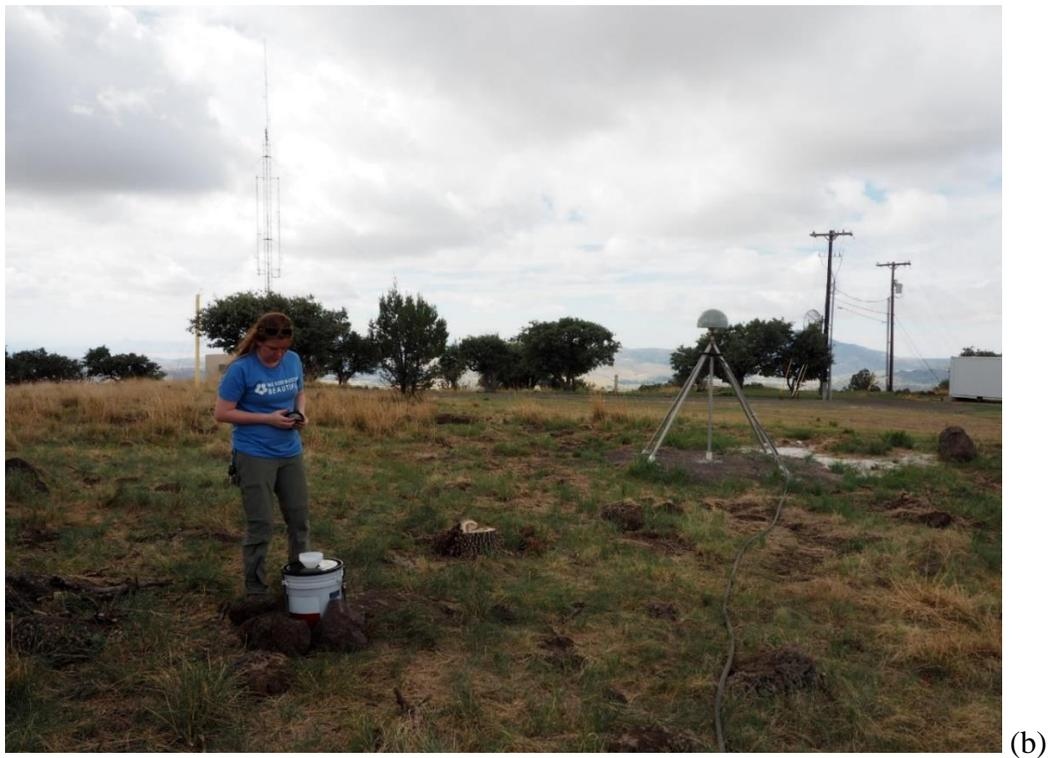
Photo 1. (a) TexNet Station at Balmorhea State Park: installing rain sample buckets near Balmorhea State Park TexNet station (Foreground) and rain sample jug inside bucket; (b) McDonald Observatory Affixing funnel to top of rain-sample bucket.
