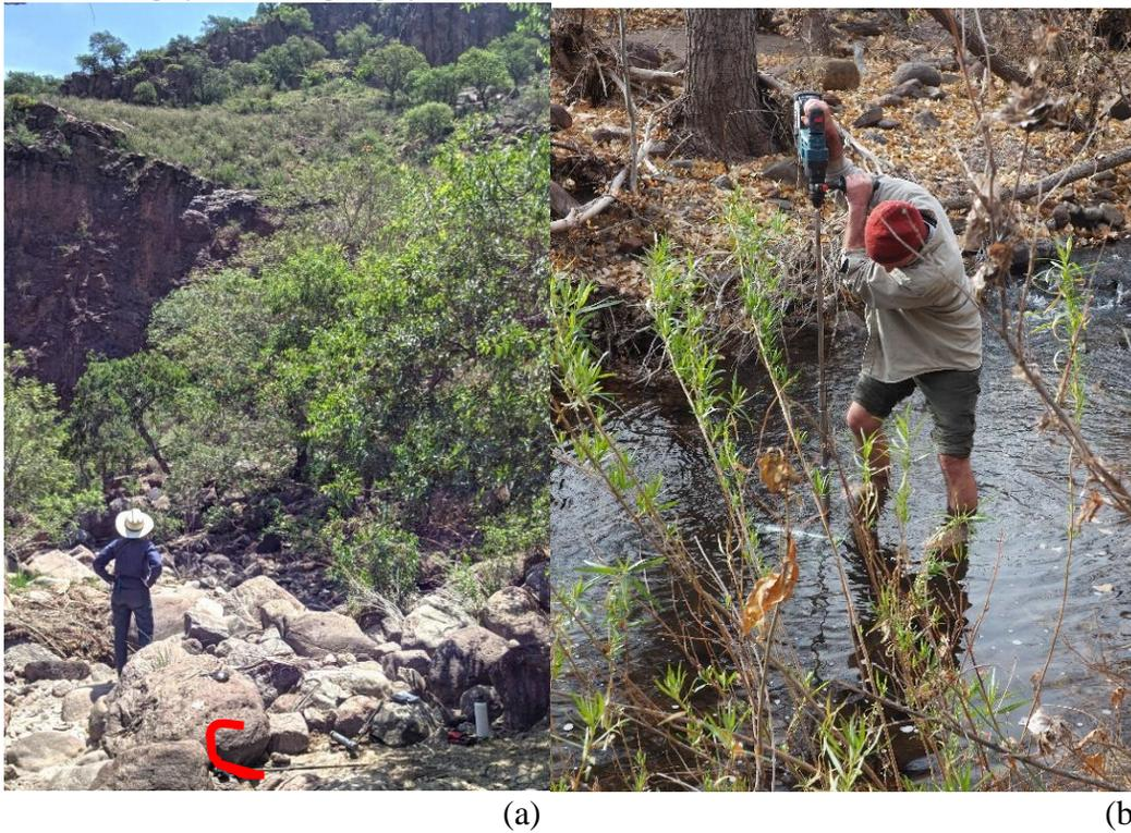
Photo 12. (a) Little Aguja Stream RuggedTroll on Buffalo Trail Scout Camp: logger in dry streambed (downstream view); (b) Big Aguja Stream AquaTroll on McCoy-Remme ranch property: installation of logger downstream from perennial springs (December 2018).
