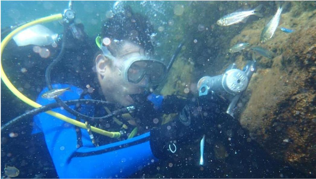
Photo 3. Installation of logger at the main orifice of San Solomon Spring in BSP pool.
