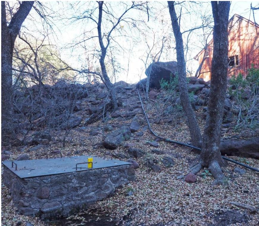
Photo 8. Igneous Willow Spring AquaTroll on Cherry Canyon Ranch, logger is mounted inside on bottom of spring box.
