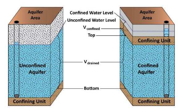
Figure 5-1. Schematic graph showing the difference between unconfined and confined aquifers (from Wade and Bradley, 2013).
