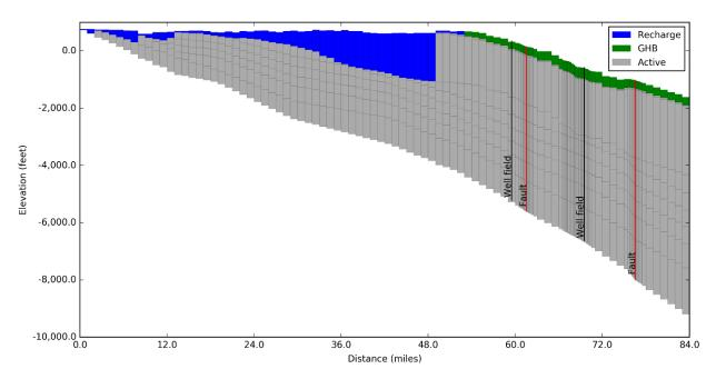
Figure 6-9. Vertical cross-section that shows the nine model layers and the hydraulic boundary conditions used in the groundwater model and the position of two well fields and three fault zones along the transect that intersects PPA #4.
