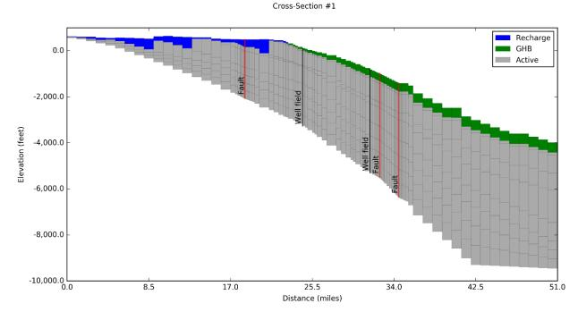
Figure 6-6. Vertical cross-section that shows the nine model layers and the hydraulic boundary conditions used in the groundwater model and the position of two well fields and three fault zones along the transect that intersects PPA #1.
