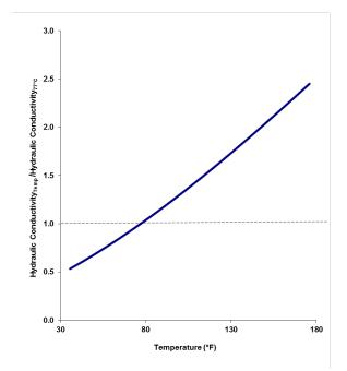
Figure 6-20. Relative change in hydraulic conductivity values caused by the temperature dependence of the density and viscosity of water.
