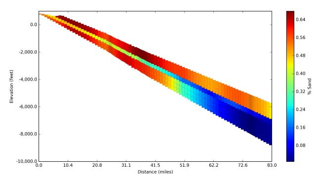
Figure 6-14. Sand fraction for model layers 5, 6, 7, 8, and 9 for a vertical cross-section cut through the three-dimensional model for PPA #3.
