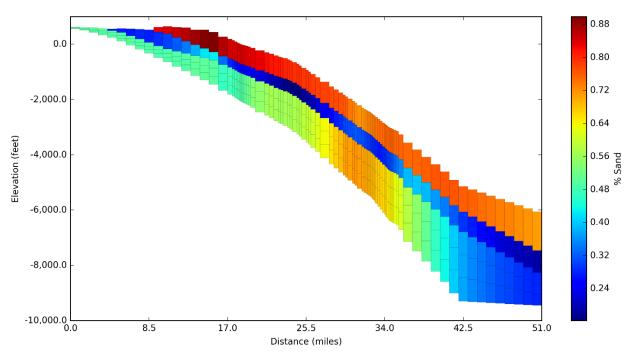
Figure 6-12. Sand fraction for model layers 5, 6, 7, 8, and 9 for a vertical cross-section cut through the three-dimensional model for PPA #1.
