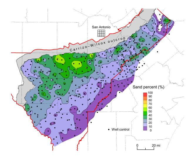
Figure 4-14. Middle Wilcox percent sand (net sand thickness / total interval thickness). The middle Wilcox is typically >50% shale (<50% sand), but in large parts of GMA 13, the middle Wilcox is >70% shale.
