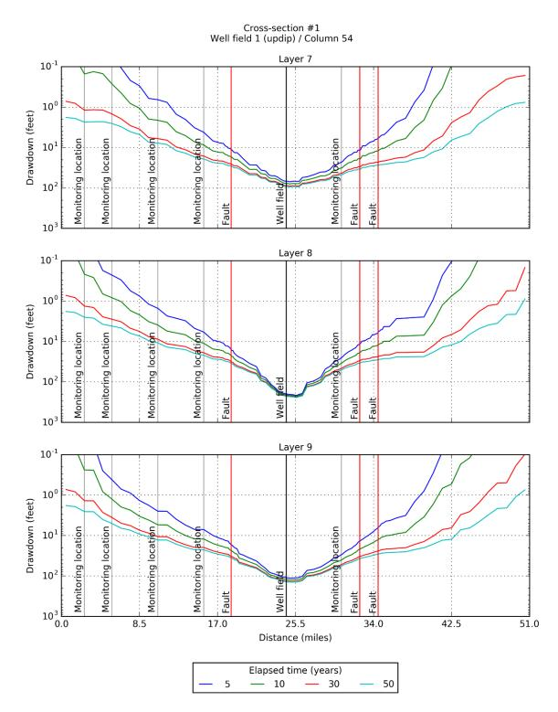
Figure 6-32. Simulated drawdown at 5, 10, 30, and 50 years for model layers 7, 8, and 9 after pumping the up dip Well Field #1 located in PPA #1 at 15,000 AFY as determined by the groundwater model with GHSM-based hydraulic properties for Carrizo-Wilcox Aquifer.
