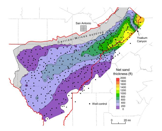
Figure 4-19. Lower Wilcox net sand thickness. Maximum sand thicknesses in the lower Wilcox are located in the northeast part of the study area. The shale-filled Yoakum Canyon erosionally truncates lower Wilcox sands.
