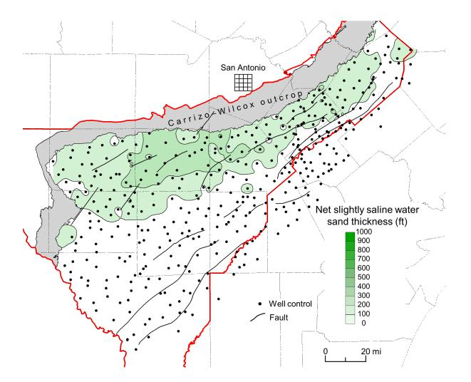
Figure 4-16. Net thickness of sand containing slightly saline groundwater in the middle Wilcox interval. Fault zones modified from Ewing (1990) and Hargis (2009).
