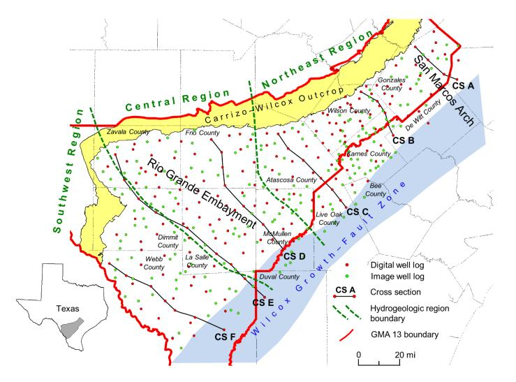
Figure 4-1. Location of study area in GMA 13 showing electric log well control, cross section lines, and Carrizo–Wilcox outcrop. The Wilcox growth-fault zone and selected updip fault zones are also shown (Ewing, 1990). The area was divided into hydrogeologic regions (Hamlin, 1988) for separate TDS/R<sub>0</sub> regressions.
