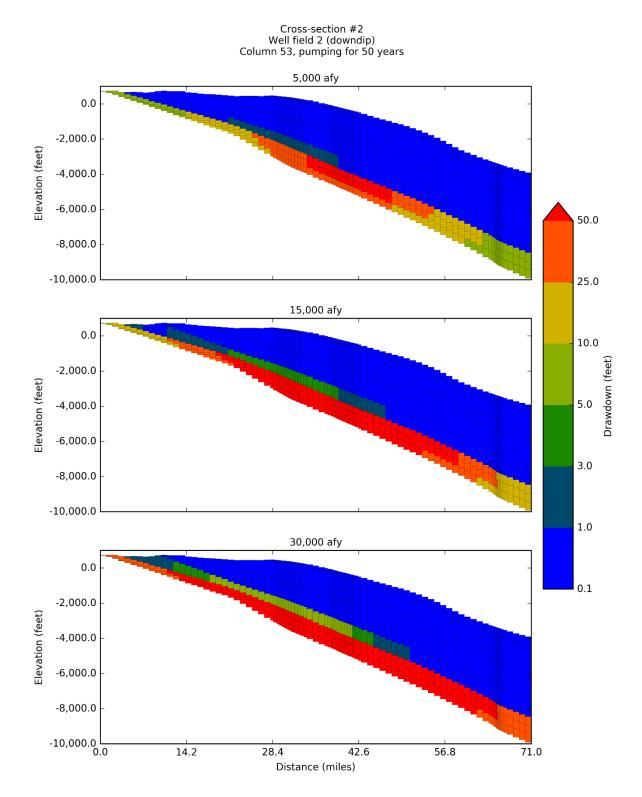
Figure 6-38. Simulated drawdown at 50 years after pumping the up dip Well Field #2 located in PPA #2 at 5,000 AFY, 15,000 AFY, and 30,000 AFY produced by the groundwater model with GAM-based hydraulic properties for Carrizo-Wilcox Aquifer.
