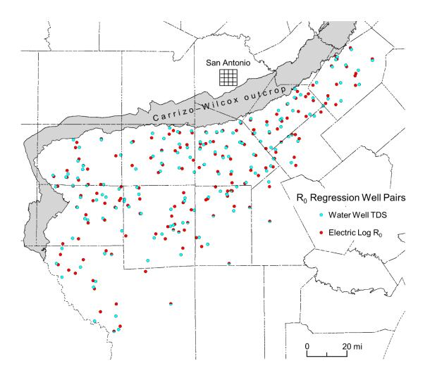
Figure 4-3. Wells used to develop TDS/R<sub>0</sub> regressions. Most TDS data (blue dots) come from water wells, whereas most resistivity data (red dots) come from petroleum wells. A few wells have both data types (red and blue dots).
