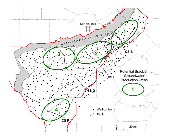
Figure 4-37. Potential brackish groundwater production areas in the Carrizo–Wilcox Aquifer in GMA 13. Structural cross sections show the vertical location and stratigraphic setting of each production area (Figures 4-32 – 4-35).
