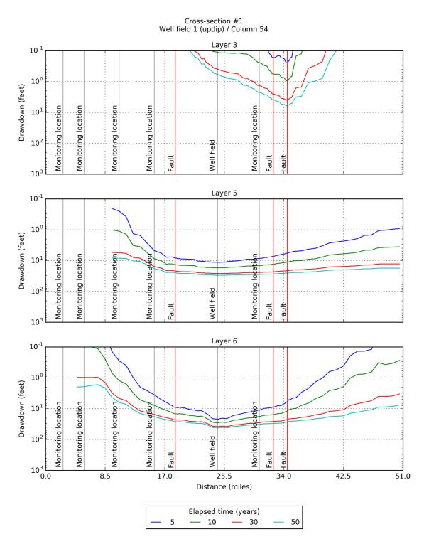
Figure 6-31. Simulated drawdown at 5, 10, 30, and 50 years for model layers 3, 5, and 6 after pumping the up dip Well Field #1 located in PPA #1 at 15,000 AFY as determined by the groundwater model with GHSM-based hydraulic properties for Carrizo-Wilcox Aquifer.
