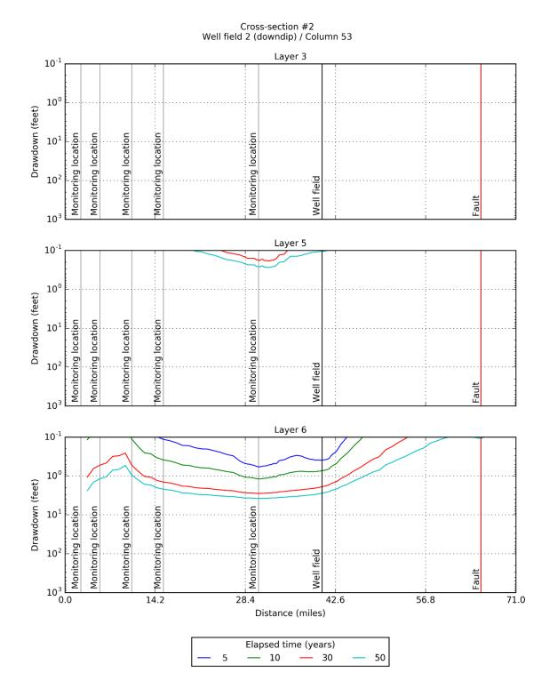
Figure 6-43. Simulated drawdown at 5, 10, 30, and 50 years for model layers 3, 5, and 6 after pumping the up dip Well Field #2 located in PPA #2 at 15,000 AFY produced by the groundwater model with GAM-based hydraulic properties for Carrizo-Wilcox Aquifer.
