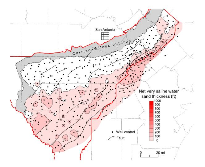
Figure 4-18. Net thickness of sand containing very saline groundwater in the middle Wilcox interval. Fault zones modified from Ewing (1990) and Hargis (2009).
