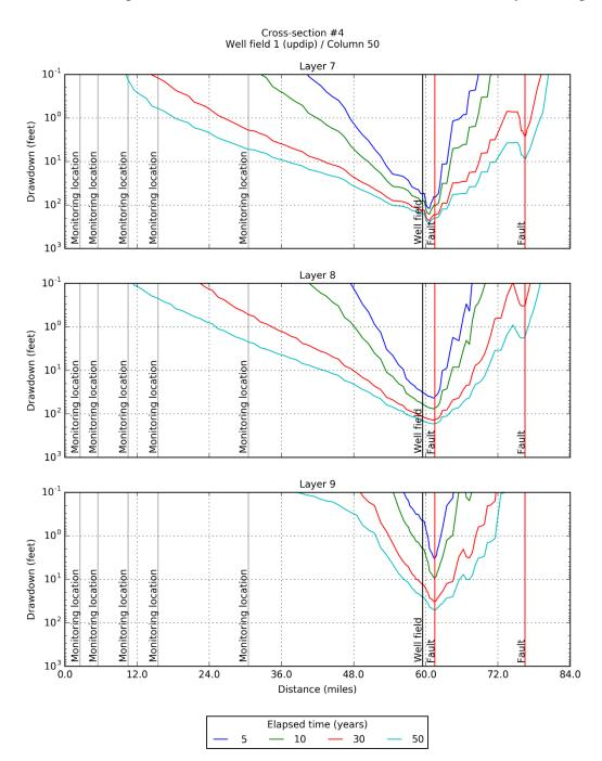
Figure 6-74. Simulated drawdown at 5, 10, 30, and 50 years for model layers 7, 8, and 9 after pumping the up dip Well Field #1 located in PPA #4 at 15,000 AFY produced by the groundwater model with GHSM-based hydraulic properties for Carrizo-Wilcox Aquifer.
