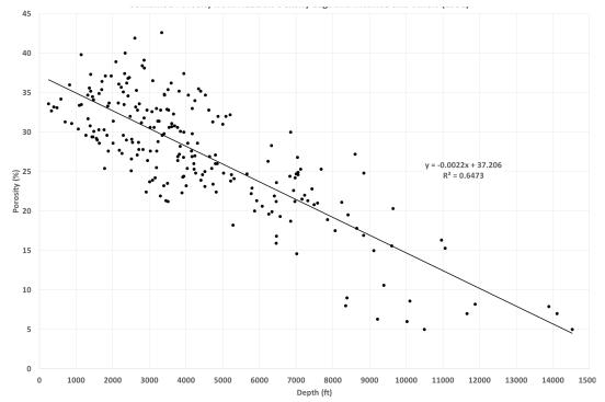
Figure 6-18. Porosity as a function of depth based on porosity data from this study and McBride and others (1991).
