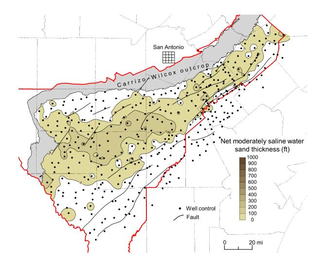
Figure 4-17. Net thickness of sand containing moderately saline groundwater in the middle Wilcox interval. Fault zones modified from Ewing (1990) and Hargis (2009).
