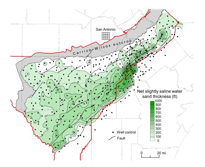
Figure 4-10. Net thickness of sand containing slightly saline groundwater in the Carrizo–upper Wilcox interval. Fault zones modified from Ewing (1990) and Hargis (2009).
