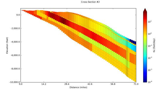
Figure 6-35. Horizontal hydraulic conductivity values in the groundwater model for PPA #2 with properties that are GAM-based for model layers 1 to 9.
