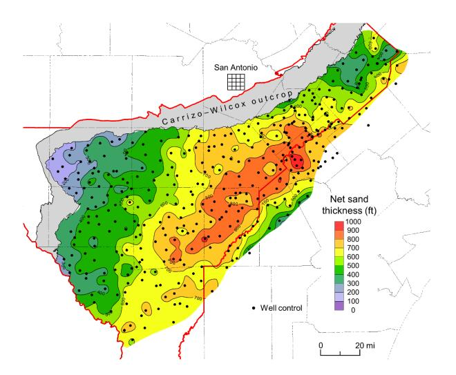
Figure 4-8. Carrizo-upper Wilcox net sand thickness. Maximum sand thicknesses in the Carrizo-upper Wilcox form a depocenter south of San Antonio.
