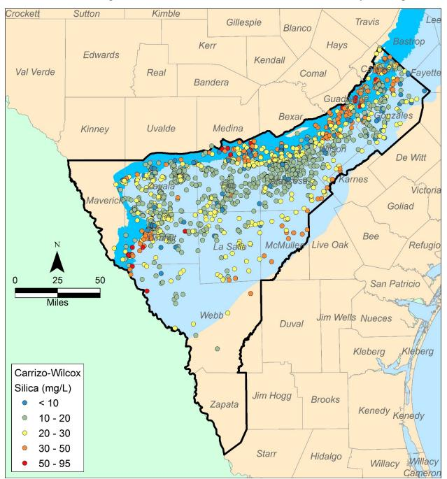
Figure 3-9. Distribution of groundwater silica (SiO2) concentrations in the Carrizo-Wilcox aquifer based on the most recent chemical analyses.
