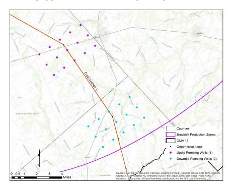
Figure 6-2. Location the two well fields along cross-section #1. Both well fields are illustrated using the 15 well network used to pump 30,000 AFY.
