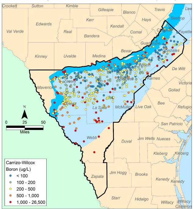
Figure 3-15. Distribution of groundwater boron (B) concentrations in the Carrizo-Wilcox aquifer based on the most recent chemical analyses.
