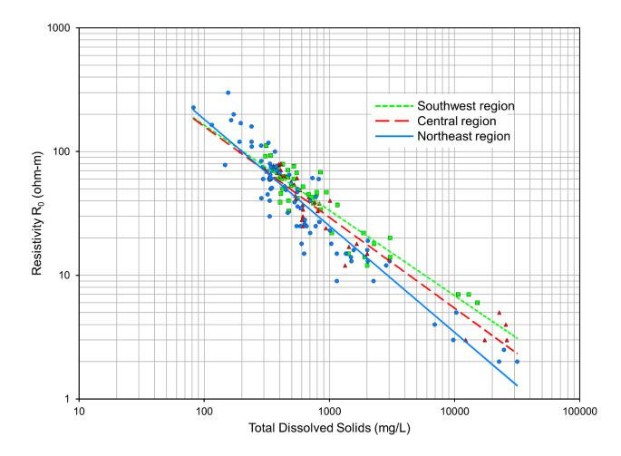
Figure 4-5. TDS versus deep resistivity (R<sub>0</sub>) showing separate regressions for each of the three hydrogeologic regions (Figure 4-1).
