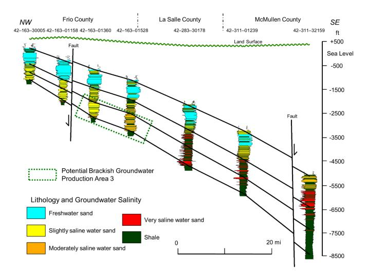
Figure 4-35. Structural cross section D (sea-level datum) showing lithologies and groundwater salinities. Faults and potential brackish groundwater production areas are also shown. See Figure 4-1 for location.
