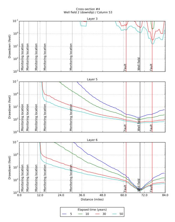
Figure 6-71. Simulated drawdown at 5, 10, 30, and 50 years for model layers 3, 5, and 6 after pumping the up dip Well Field #2 located in PPA #4 at 15,000 AFY produced by the groundwater model with GAM-based hydraulic properties for Carrizo-Wilcox Aquifer.
