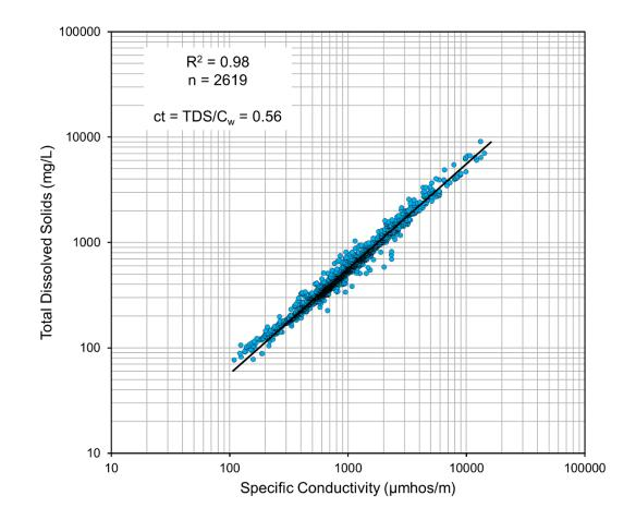
Figure 4-6. Graph of specific conductivity (C<sub>w</sub>) versus TDS for the study area. Both C<sub>w</sub> and TDS were measured in water well samples. C<sub>w</sub> and TDS are related by a proportionality constant (ct), which is specific to area and formation. In the South Texas, however, a single value of ct is valid for the entire Carrizo–Wilcox aquifer.
