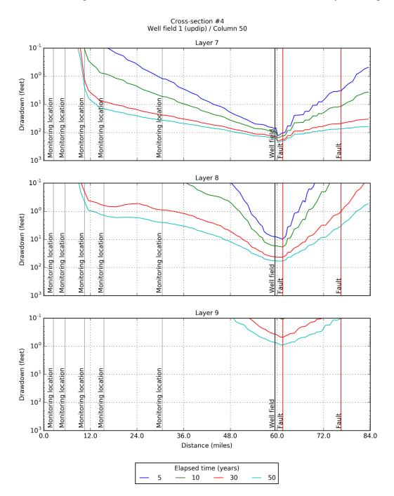
Figure 6-70. Simulated drawdown at 5, 10, 30, and 50 years for model layers 7, 8, and 9 after pumping the up dip Well Field #1 located in PPA #4 at 15,000 AFY produced by the groundwater model with GAM-based hydraulic properties for Carrizo-Wilcox Aquifer.
