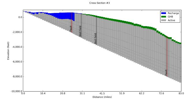
Figure 6-8. Vertical cross-section that shows the nine model layers and the hydraulic boundary conditions used in the groundwater model and the position of two well fields and three fault zones along the transect that intersects PPA #3.
