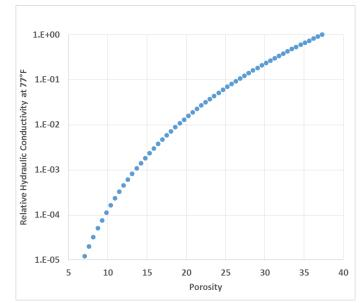
Figure 6-19. Change in relative hydraulic conductivity as a function of change in porosity based on data from Dutton and Loucks (2014).
