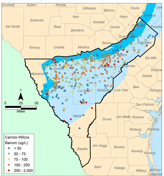
Figure 3-14. Distribution of groundwater barium (Ba) concentrations in the Carrizo-Wilcox aquifer based on the most recent chemical analyses.
