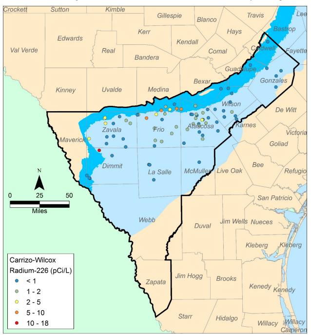
Figure 3-11. Distribution of groundwater radium-226 (Ra-226) concentrations in the Carrizo-Wilcox aquifer based on the most recent chemical analyses.
