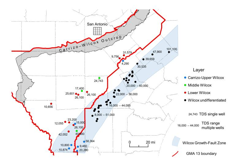
Figure 4-7. High groundwater salinities from oil and gas wells. Data from Taylor (1975) and Gaither (1986).
