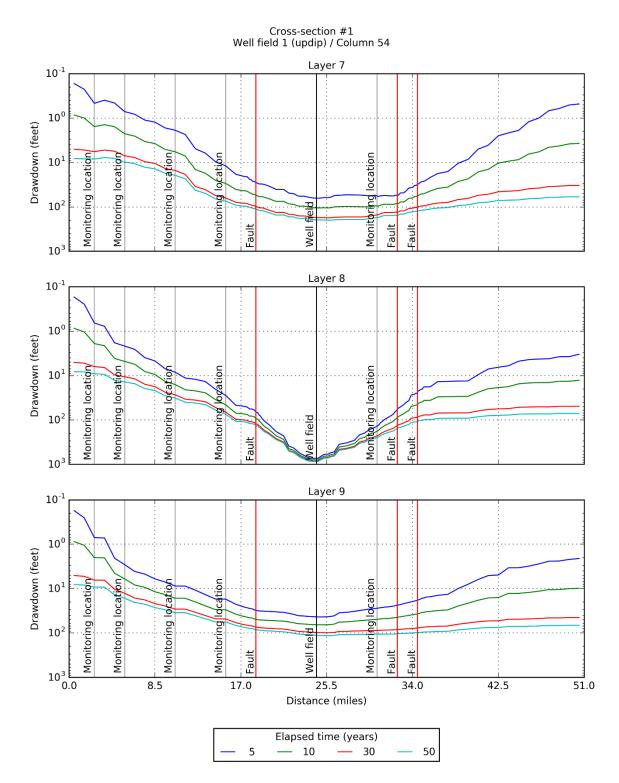
Figure 6-28. Simulated drawdown at 5, 10, 30, and 50 years for model layers 7, 8, and 9 after pumping the up dip Well Field #1 located in PPA #1 at 15,000 AFY as determined by the groundwater model with GAM-based hydraulic properties for Carrizo-Wilcox Aquifer.
