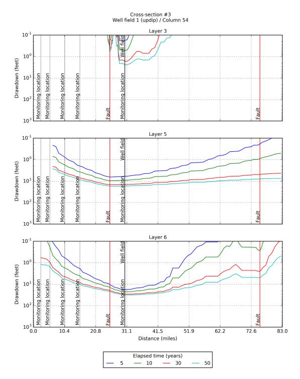
Figure 6-59. Simulated drawdown at 5, 10, 30, and 50 years for model layers 3, 5, and 6 after pumping the up dip Well Field #1 located in PPA #3 at 15,000 AFY produced by the groundwater model with GHSM-based hydraulic properties for Carrizo-Wilcox Aquifer
