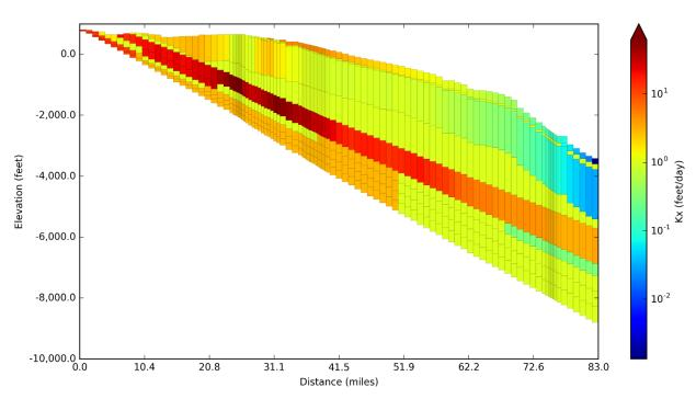
Figure 6-49. Horizontal hydraulic conductivity values in the groundwater model for PPA #3 with properties that are GAM-based for model layers 1 to 9.
