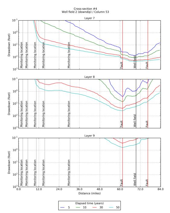
Figure 6-72. Simulated drawdown at 5, 10, 30, and 50 years for model layers 7, 8, and 9 after pumping the up dip Well Field #2 located in PPA #4 at 15,000 AFY produced by the groundwater model with GAM-based hydraulic properties for Carrizo-Wilcox Aquifer.
