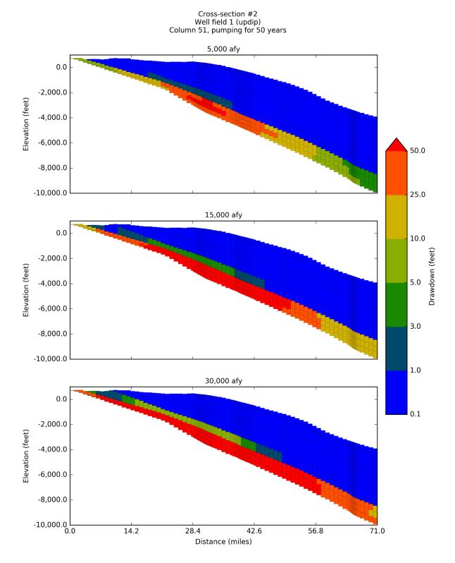
Figure 6-37. Simulated drawdown at 50 years after pumping the up dip Well Field #1 located in PPA #2 at 5,000 AFY, 15,000 AFY, and 30,000 AFY produced by the groundwater model with GAM-based hydraulic properties for Carrizo-Wilcox Aquifer.
