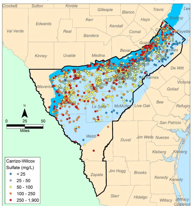
Figure 3-13. Distribution of groundwater sulfate (SO4) concentrations in the Carrizo-Wilcox aquifer based on the most recent chemical analyses.
