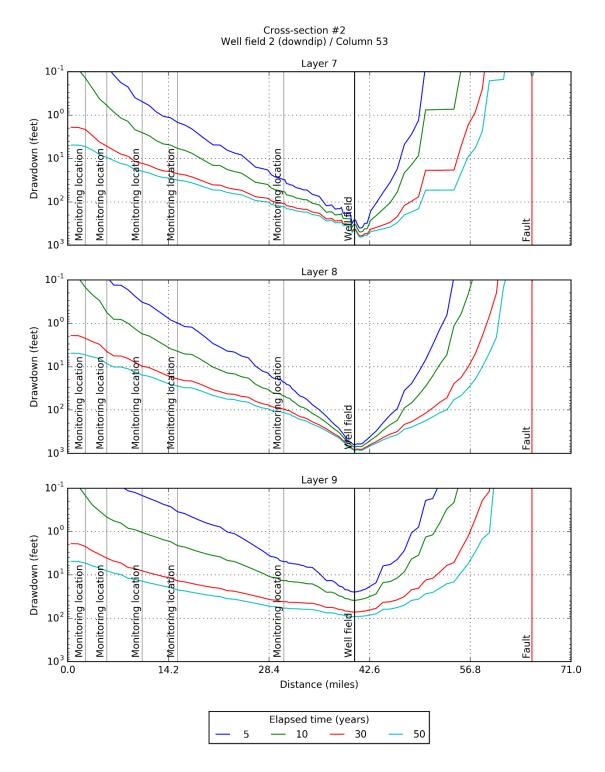
Figure 6-48. Simulated drawdown at 5, 10, 30, and 50 years for model layers 7, 8, and 9 after pumping the up dip Well Field #2 located in PPA #2 at 15,000 AFY produced by the groundwater model with GHSM-based hydraulic properties for Carrizo-Wilcox Aquifer.
