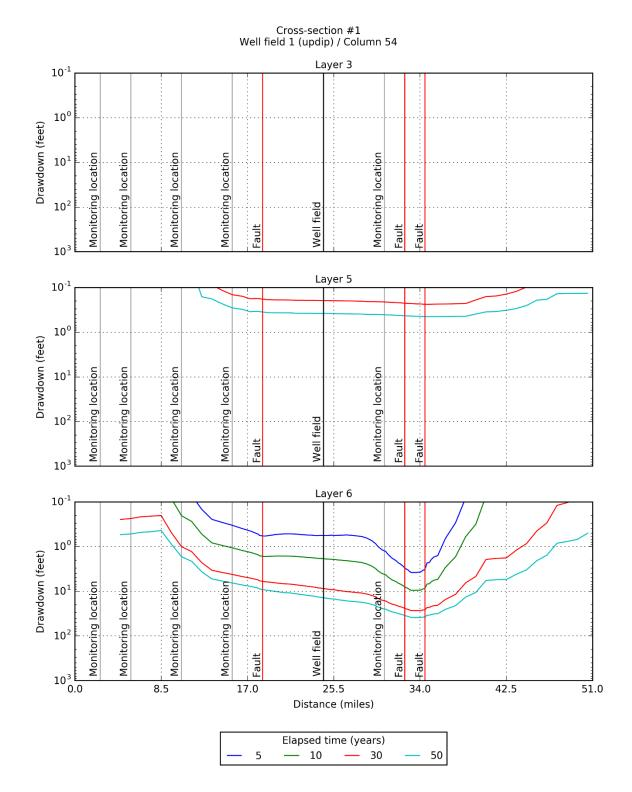
Figure 6-27. Simulated drawdown at 5, 10, 30, and 50 years for model layers 3, 5, and 6 after pumping the up dip Well Field #1 located in PPA #1 at 15,000 AFY as determined by the groundwater model with GAM based hydraulic properties for Carrizo-Wilcox Aquifer.
