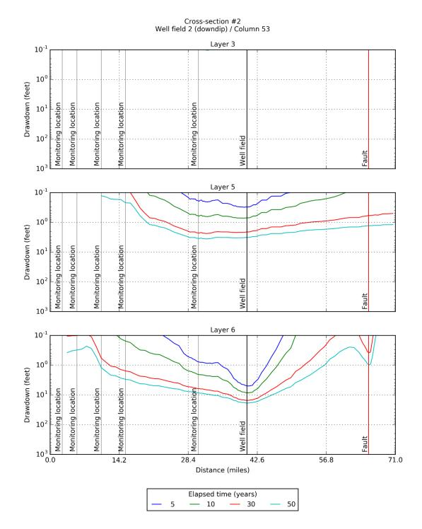
Figure 6-47. Simulated drawdown at 5, 10, 30, and 50 years for model layers 3, 5, and 6 after pumping the up dip Well Field #2 located in PPA #2 at 15,000 AFY produced by the groundwater model with GHSM-based hydraulic properties for Carrizo-Wilcox Aquifer.
