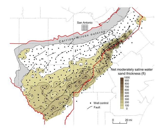
Figure 4-11. Net thickness of sand containing moderately saline groundwater in the Carrizo–upper Wilcox interval. Fault zones modified from Ewing (1990) and Hargis (2009).
