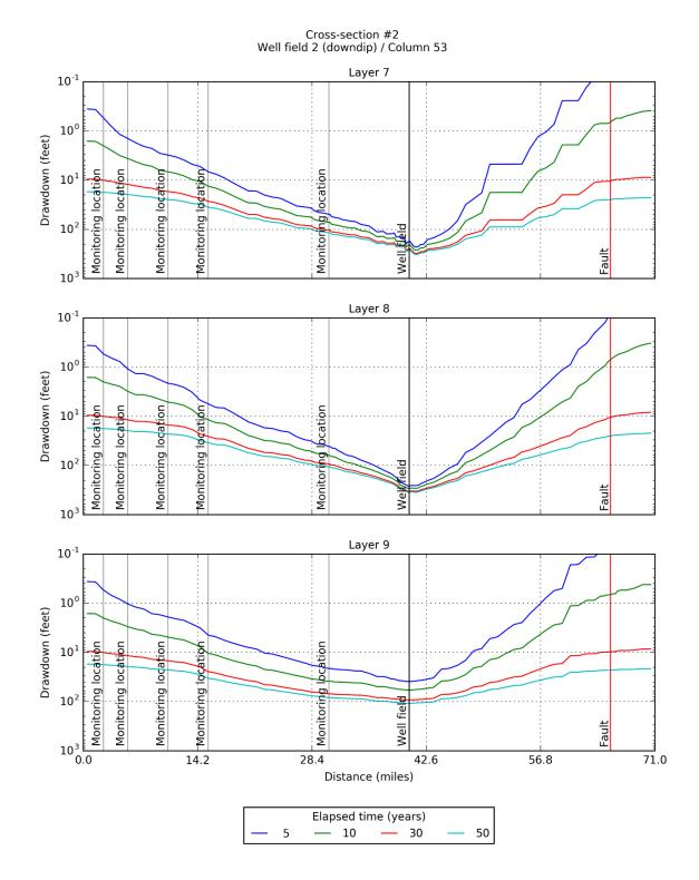
Figure 6-44. Simulated drawdown at 5, 10, 30, and 50 years for model layers 7, 8, and 9 after pumping the up dip Well Field #2 located in PPA #2 at 15,000 AFY produced by the groundwater model with GAM-based hydraulic properties for Carrizo-Wilcox Aquifer.
