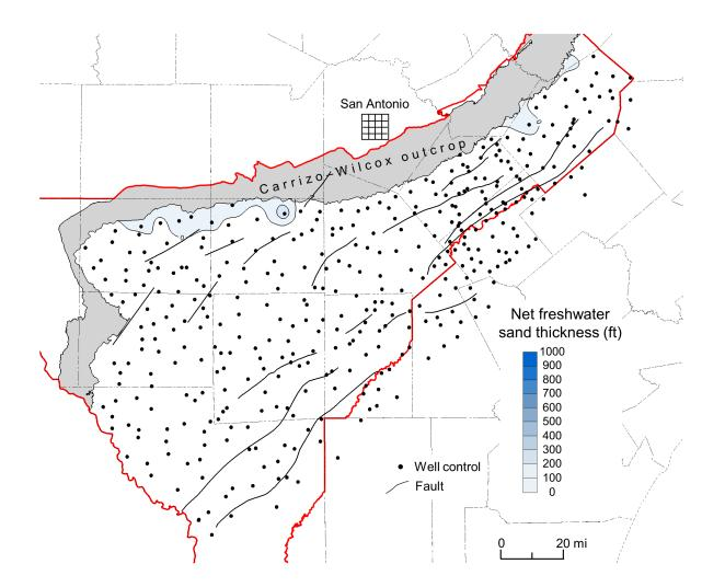
Figure 4-20. Net thickness of sand containing fresh groundwater in the lower Wilcox interval. Fault zones modified from Ewing (1990) and Hargis (2009).
