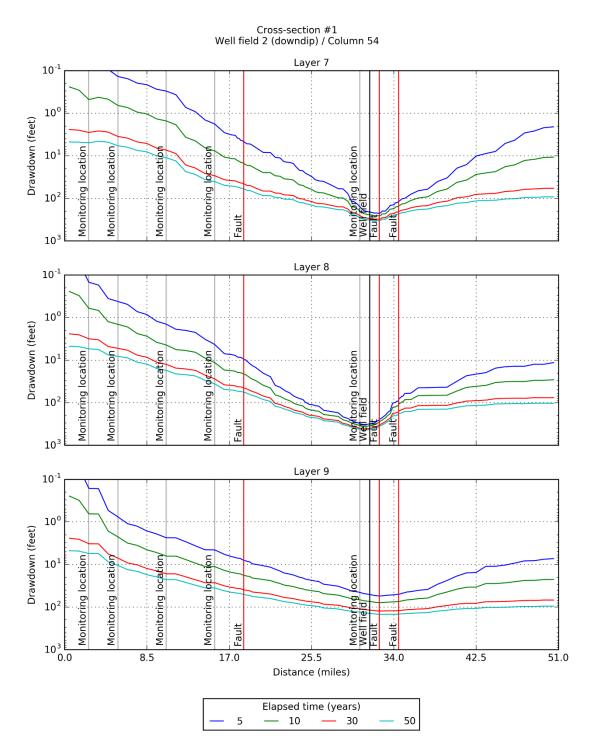
Figure 6-30. Simulated drawdown at 5, 10, 30, and 50 years for model layers 7, 8, and 9 after pumping the up dip Well Field #2 located in PPA #1 at 15,000 AFY as determined by the groundwater model with GAM-based hydraulic properties for Carrizo-Wilcox Aquifer.
