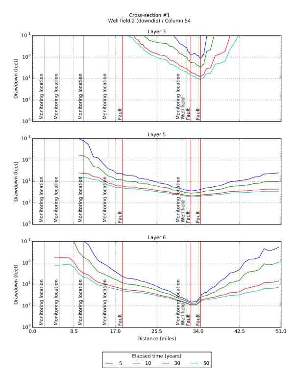
Figure 6-33. Simulated drawdown at 5, 10, 30, and 50 years for model layers 3, 5, and 6 after pumping the up dip Well Field #2 located in PPA #1 at 15,000 AFY as determined by the groundwater model with GHSM-based hydraulic properties for Carrizo-Wilcox Aquifer.
