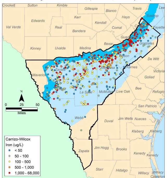
Figure 3-10. Distribution of groundwater iron (Fe) concentrations in the Carrizo-Wilcox aquifer based on the most recent chemical analyses.
