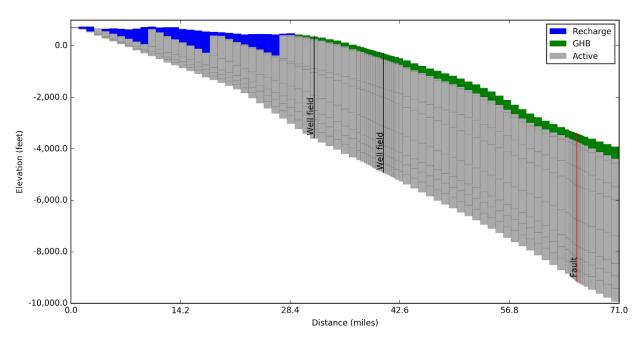
Figure 6-7. Vertical cross-section that shows the nine model layers and the hydraulic boundary conditions used in the groundwater model and the position of two well fields and three fault zones along the transect that intersects PPA #2.
