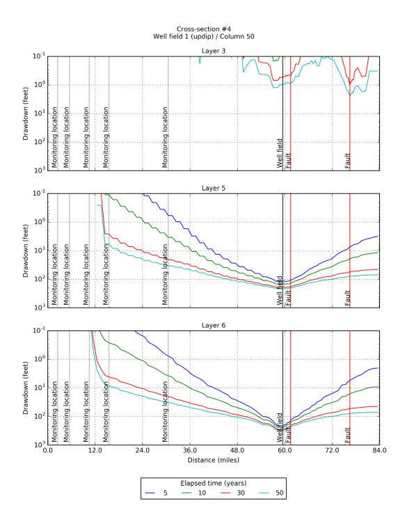
Figure 6-69. Simulated drawdown at 5, 10, 30, and 50 years for model layers 3, 5, and 6 after pumping the up dip Well Field #1 located in PPA #4 at 15,000 AFY produced by the groundwater model with GAM-based hydraulic properties for Carrizo-Wilcox Aquifer.
