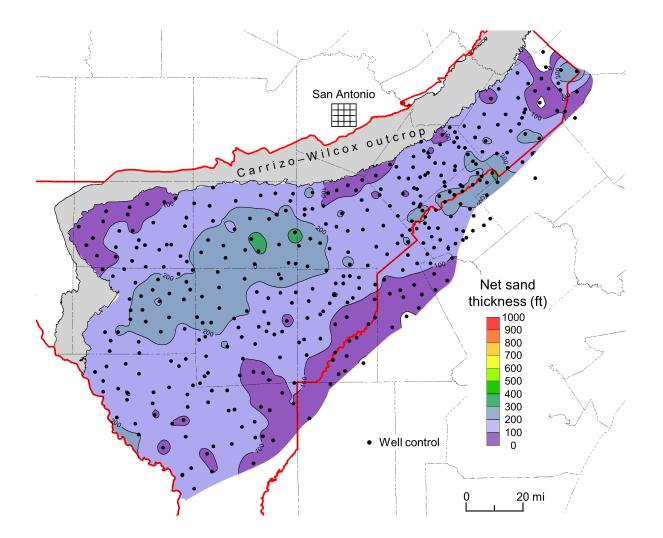
Figure 4-13. Middle Wilcox net sand thickness. The middle Wilcox is typically a low-sand, high-shale interval.
