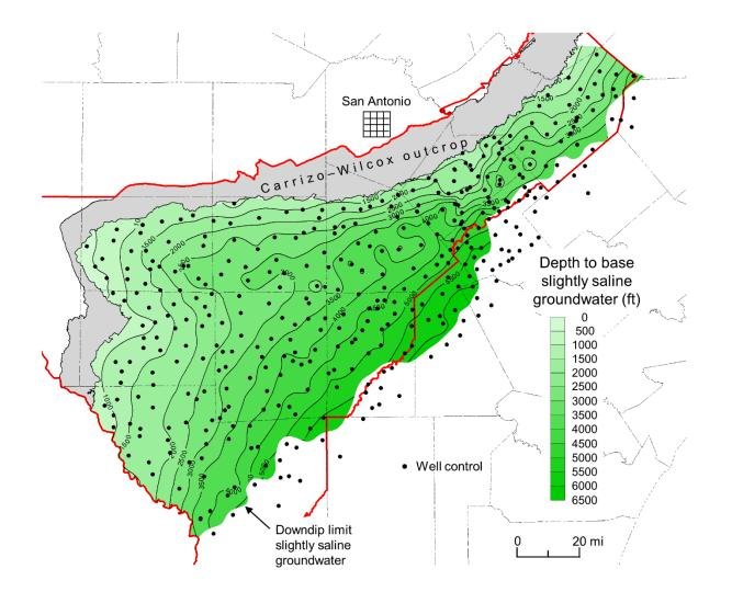
Figure 4-31. Depth from surface to base (deepest occurrence) of slightly saline groundwater in the Carrizo–Wilcox aquifer.
