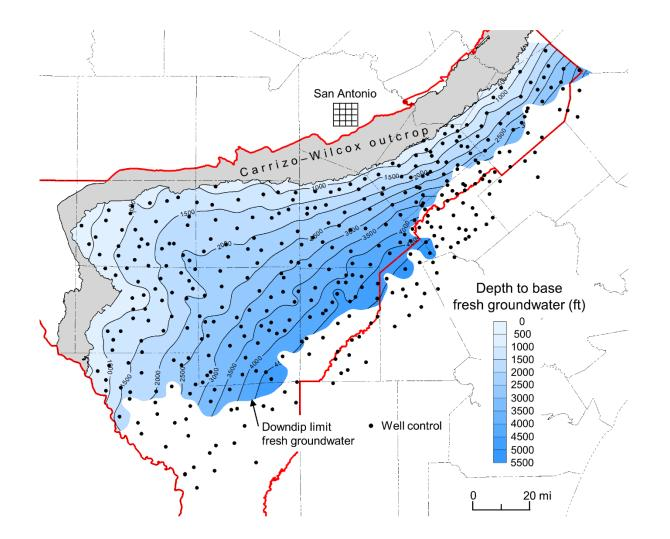
Figure 4-30. Depth from surface to base (deepest occurrence) of fresh groundwater in the Carrizo–Wilcox aquifer. Almost all fresh groundwater is in the Carrizo–upper Wilcox interval.
