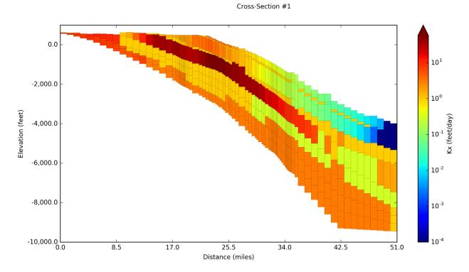
Figure 6-21. Horizontal hydraulic conductivity values in the groundwater model for PPA #1 with properties that are GAM-based for model layers 1 to 9.
