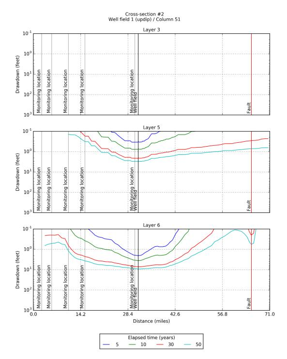
Figure 6-45. Simulated drawdown at 5, 10, 30, and 50 years for model layers 3, 5, and 6 after pumping the up dip Well Field #1 located in PPA #2 at 15,000 AFY produced by the groundwater model with GHSM-based hydraulic properties for Carrizo-Wilcox Aquifer.
