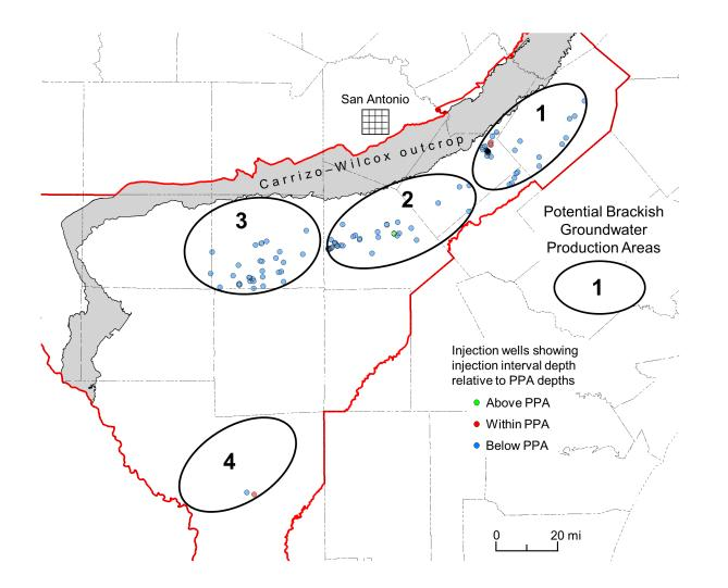
Figure 4-38. Location of Class II injection wells within the potential brackish groundwater production areas. Injection intervals relative to the PPAs are also shown.
