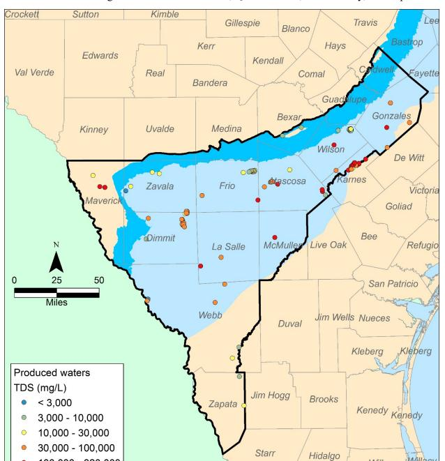
Figure 3-4. Location and TDS concentrations of wells with water samples from the USGS Produced Waters database (http://energy.usgs.gov/EnvironmentalAspects/EnvironmentalAspectsofEnergyProductionan dUse/ProducedWaters.aspx#3822349-data)
