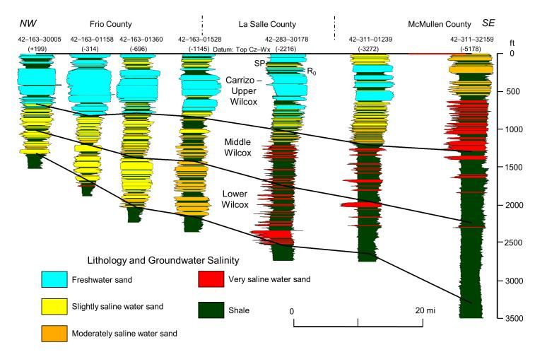
Figure 4-27. Stratigraphic cross section D showing lithologies and groundwater salinities. See Figure 4-1 for location. Well API numbers are shown at top. SP (left side) and resistivity (right side) logs are shown for each well. Subsea elevation of the datum (top Carrizo–Wilcox Aquifer) is also shown for each well.
