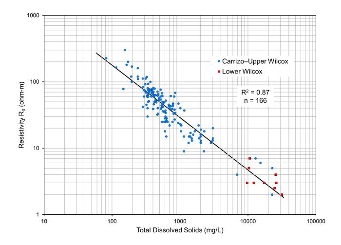
Figure 4-4. Total dissolved solids (TDS) versus deep resistivity (R<sub>0</sub>) for all well pairs in the study area.
