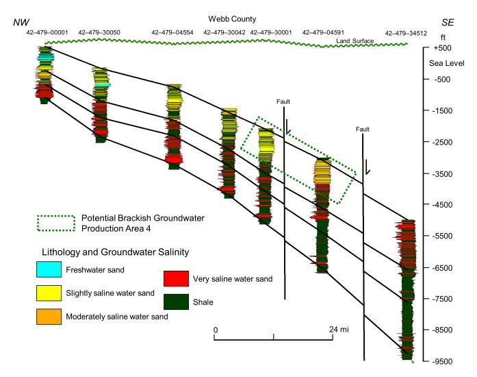
Figure 4-36. Structural cross section F (sea-level datum) showing lithologies and groundwater salinities. Faults and potential brackish groundwater production areas are also shown. See Figure 4-1 for location.
