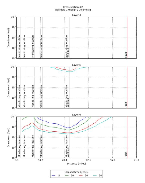
Figure 6-41. Simulated drawdown at 5, 10, 30, and 50 years for model layers 3, 5, and 6 after pumping the up dip Well Field #1 located in PPA #2 at 15,000 AFY produced by the groundwater model with GAM-based hydraulic properties for Carrizo-Wilcox Aquifer.
