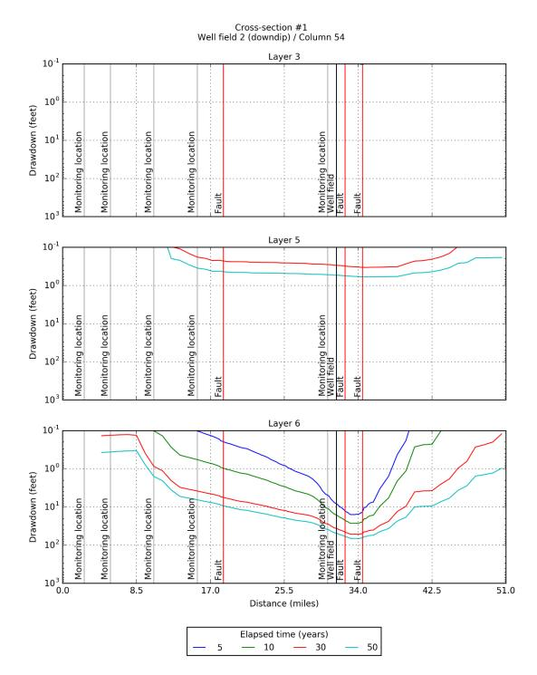
Figure 6-29. Simulated drawdown at 5, 10, 30, and 50 years for model layers 3, 5, and 6 after pumping the up dip Well Field #2 located in PPA #1 at 15,000 AFY as determined by the groundwater model with GAM-based hydraulic properties for Carrizo-Wilcox Aquifer.
