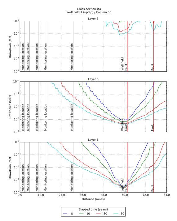
Figure 6-73. Simulated drawdown at 5, 10, 30, and 50 years for model layers 3, 5, and 6 after pumping the up dip Well Field #1 located in PPA #4 at 15,000 AFY produced by the groundwater model with GHSM-based hydraulic properties for Carrizo-Wilcox Aquifer
