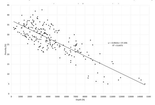
Figure 5-5. Porosity as a function of depth based on porosity data from this study and McBride and others (1991).
