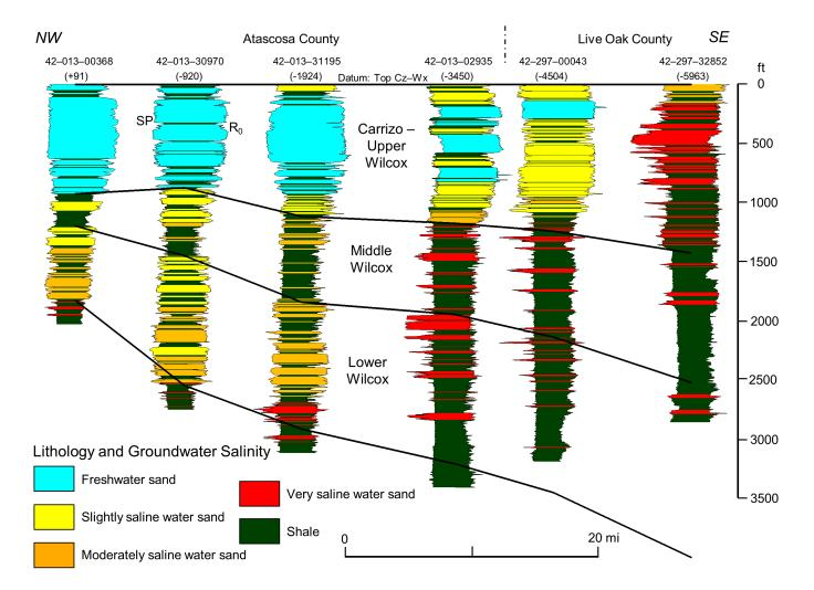
Figure 4-26. Stratigraphic cross section C showing lithologies and groundwater salinities. See Figure 4-1 for location. Well API numbers are shown at top. SP (left side) and resistivity (right side) logs are shown for each well. Subsea elevation of the datum (top Carrizo–Wilcox Aquifer) is also shown for each well.
