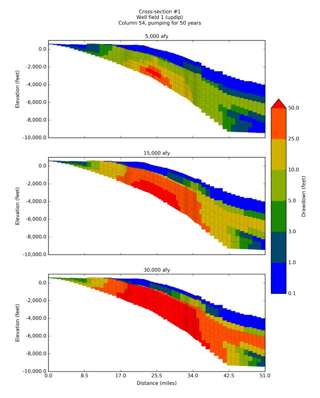
Figure 6-25. Simulated drawdown at 50 years after pumping the up dip Well Field #1 located in PPA #1 at 5,000 AFY, 15,000 AFY, and 30,000 AFY as determined by the groundwater model with GHSM-based hydraulic properties for Carrizo-Wilcox Aquifer.
