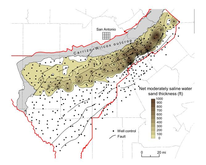
Figure 4-22. Net thickness of sand containing moderately saline groundwater in the lower Wilcox interval. Fault zones modified from Ewing (1990) and Hargis (2009).
