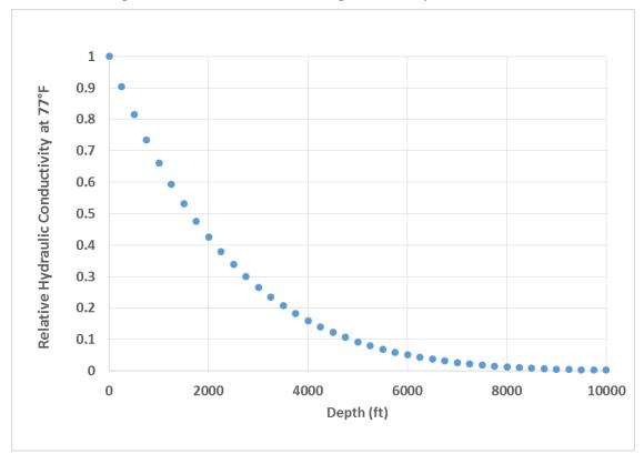
Figure 6-17. Relationship used by the GeoHydroStratigraphic Model to account for hydraulic conductivity decrease with depth caused by a decrease in porosity with depth.
