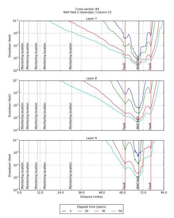
Figure 6-76. Simulated drawdown at 5, 10, 30, and 50 years for model layers 7, 8, and 9 after pumping the up dip Well Field #2 located in PPA #4 at 15,000 AFY produced by the groundwater model with GHSM-based hydraulic properties for Carrizo-Wilcox Aquifer.
