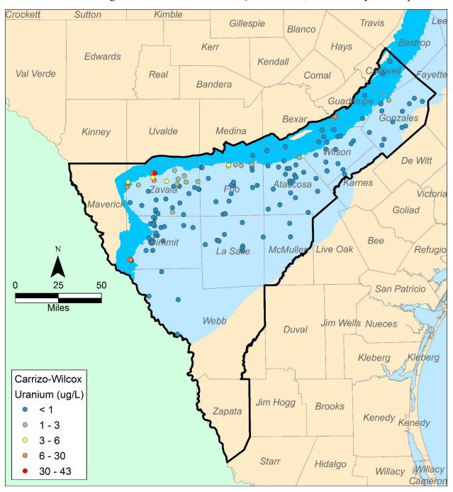
Figure 3-12. Distribution of groundwater uranium (U) concentrations in the Carrizo-Wilcox aquifer based on the most recent chemical analyses.
