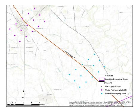
Figure 6-3. Location of the two well fields along cross-section #2. Both well fields are illustrated using the 15 well network used to pump 30,000 AFY.
