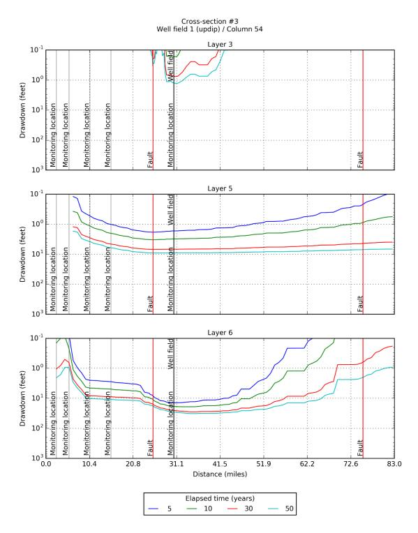
Figure 6-55. Simulated drawdown at 5, 10, 30, and 50 years for model layers 3, 5, and 6 after pumping the up dip Well Field #1 located in PPA #3 at 15,000 AFY produced by the groundwater model with GAM-based hydraulic properties for Carrizo-Wilcox Aquifer.
