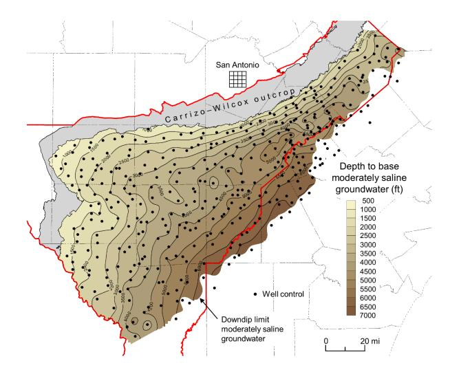
Figure 4-32. Depth from surface to base (deepest occurrence) of moderately saline groundwater in the Carrizo–Wilcox aquifer.
