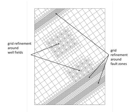
Figure 6-11. Aerial view of the groundwater model for PPA #1 showing the type of grid refinement that occurs in the vicinity of the well fields and faults to reduce from 1-mile by 1-mile grid cells to 1/8-mile by 1/8-mile grid cells.
