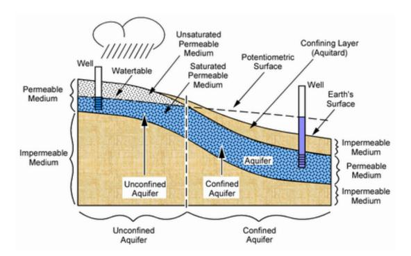
Figure 5-2. Schematic of aquifer transitioning from unconfined an outcrop region, where recharge from precipitation occurs, to confined conditions in the down dip regions of the aquifer (from http://www.geo.brown.edu/research/Hydrology/ge58\_IntrodHydrology/ge58\_index.htm).
