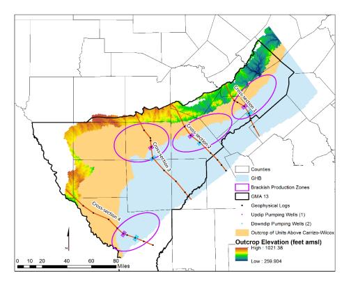
Figure 6-1. Location of transects through the four potential brackish production zones that were used for developing groundwater models for each potential production area.
