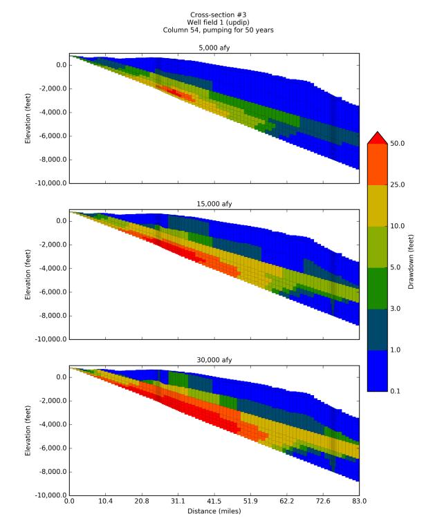
Figure 6-53. Simulated drawdown at 50 years after pumping the up dip Well Field #1 located in PPA #3 at 5,000 AFY, 15,000 AFY, and 30,000 AFY produced by the groundwater model with GHSM-based hydraulic properties for Carrizo-Wilcox Aquifer.
