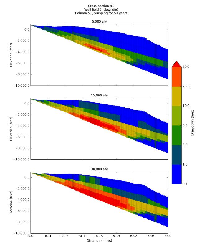
Figure 6-54. Simulated drawdown at 50 years after pumping the up dip Well Field #2 located in PPA #3 at 5,000 AFY, 15,000 AFY, and 30,000 AFY produced by the groundwater model with GHSM-based hydraulic properties for Carrizo-Wilcox Aquifer.
