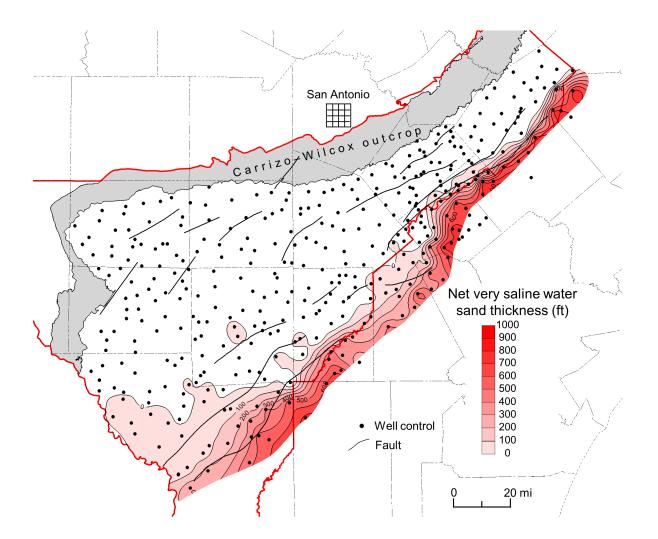
Figure 4-12. Net thickness of sand containing very saline groundwater in the Carrizo-upper Wilcox interval. Fault zones modified from Ewing (1990) and Hargis (2009).
