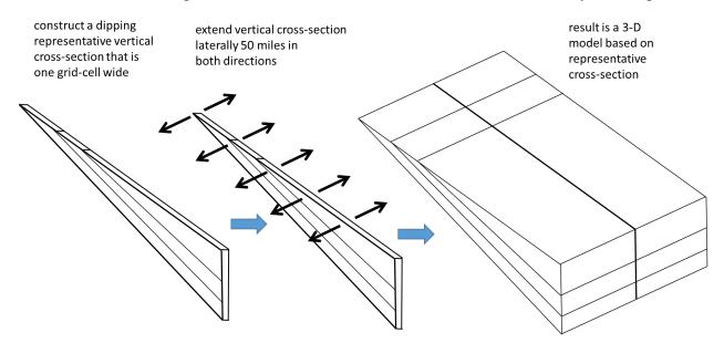
Figure 6-10. Schematic showing the lateral outward replication of a vertical cross-section, which is one grid-cell wide, to construct a three-dimensional model that covers a distance of 50 miles on both sides of the original cross-section.
