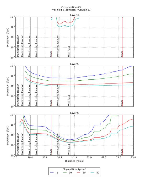
Figure 6-57. Simulated drawdown at 5, 10, 30, and 50 years for model layers 3, 5, and 6 after pumping the up dip Well Field #2 located in PPA #3 at 15,000 AFY produced by the groundwater model with GAM-based hydraulic properties for Carrizo-Wilcox Aquifer.
