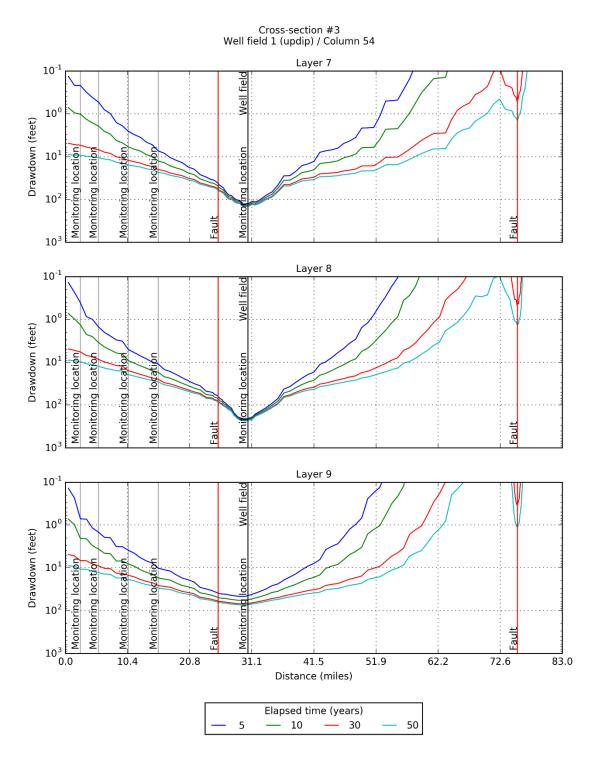
Figure 6-60. Simulated drawdown at 5, 10, 30, and 50 years for model layers 7, 8, and 9 after pumping the up dip Well Field #1 located in PPA #3 at 15,000 AFY produced by the groundwater model with GHSM-based hydraulic properties for Carrizo-Wilcox Aquifer.
