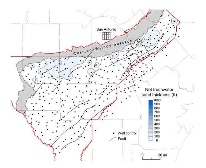
Figure 4-15. Net thickness of sand containing fresh groundwater in the middle Wilcox interval. Fault zones modified from Ewing (1990) and Hargis (2009).
