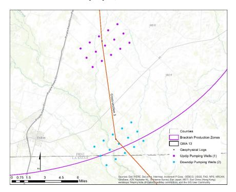
Figure 6-4. Location of the two well fields along cross-section #3. Both well fields are illustrated using the 15 well network used to pump 30,000 AFY.
