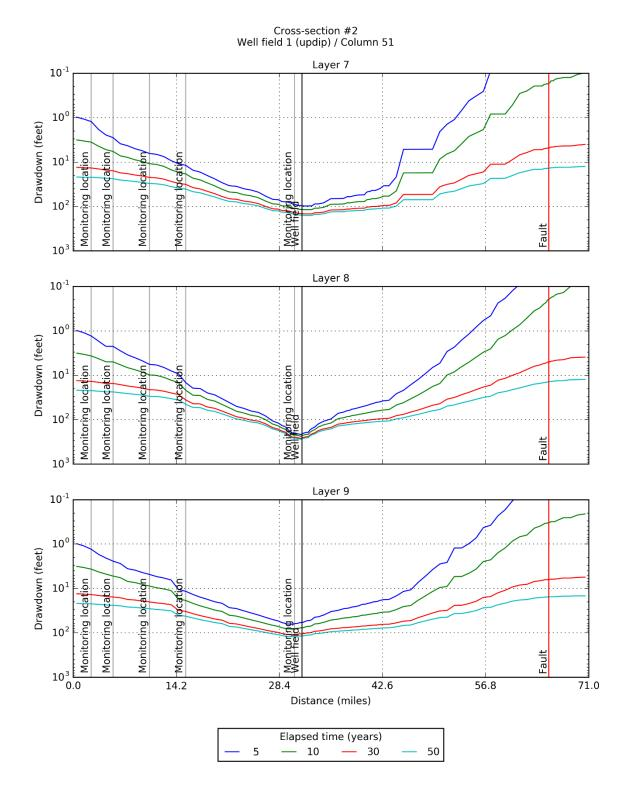
Figure 6-42. Simulated drawdown at 5, 10, 30, and 50 years for model layers 7, 8, and 9 after pumping the up dip Well Field #1 located in PPA #2 at 15,000 AFY produced by the groundwater model with GAM-based hydraulic properties for Carrizo-Wilcox Aquifer.
