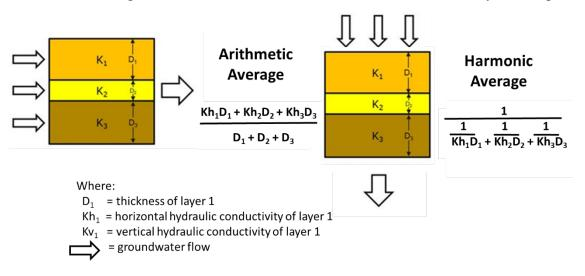
Figure 6-16. Schematic showing the application of an arithmetic average and a harmonic average to calculate equivalent horizontal and vertical hydraulic conductivities based on the assumption of one-dimension flow through uniform layered media.
