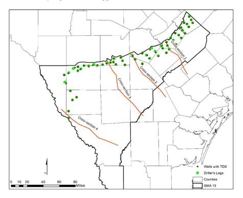
Figure 5-4. Location driller logs and a nearby water well with measured concentrations of Total Dissolved Solids (TDS).
