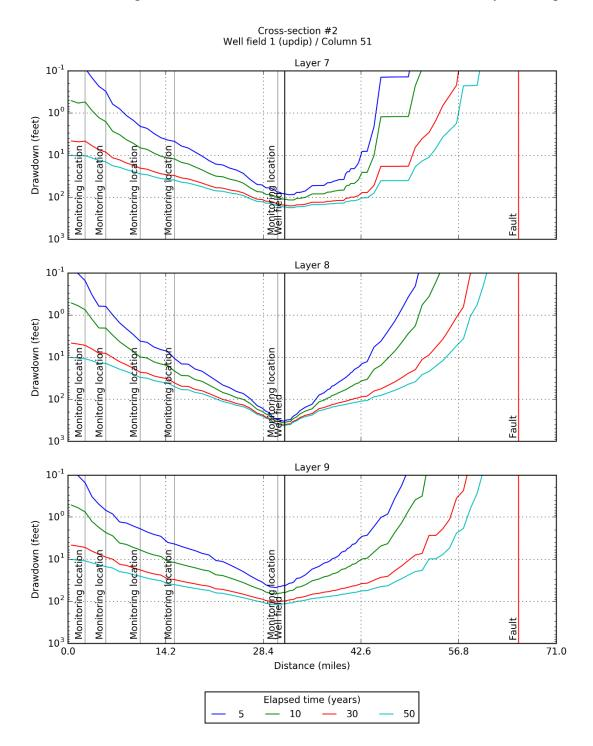
Figure 6-46. Simulated drawdown at 5, 10, 30, and 50 years for model layers 7, 8, and 9 after pumping the up dip Well Field #1 located in PPA #2 at 15,000 AFY produced by the groundwater model with GHSM-based hydraulic properties for Carrizo-Wilcox Aquifer.
