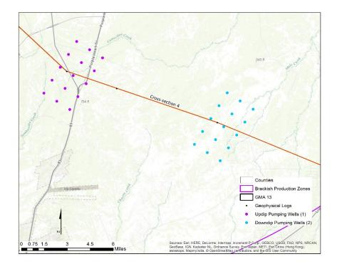
Figure 6-5. Location of the two well fields along cross-section #4. Both well fields are illustrated using the 15 well network used to pump 30,000 AFY.
