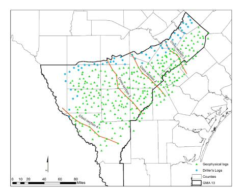
Figure 5-3. Location of the 55 driller and 323 geophysical logs used to construct continuous profiles of sand and clay sequences that support calculations of volumes.
