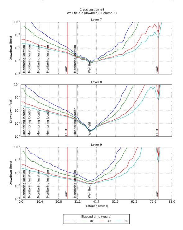
Figure 6-62. Simulated drawdown at 5, 10, 30, and 50 years for model layers 7, 8, and 9 after pumping the up dip Well Field #2 located in PPA #3 at 15,000 AFY produced by the groundwater model with GHSM-based hydraulic properties for Carrizo-Wilcox Aquifer.
