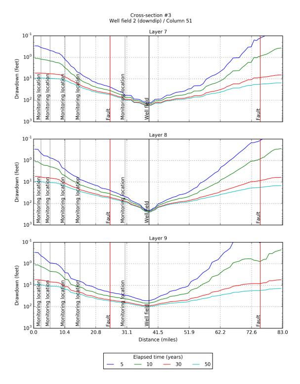
Figure 6-58. Simulated drawdown at 5, 10, 30, and 50 years for model layers 7, 8, and 9 after pumping the up dip Well Field #2 located in PPA #3 at 15,000 AFY produced by the groundwater model with GAM-based hydraulic properties for Carrizo-Wilcox Aquifer.
