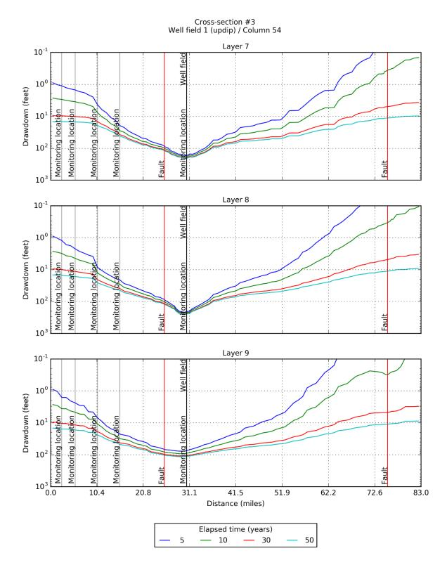
Figure 6-56. Simulated drawdown at 5, 10, 30, and 50 years for model layers 7, 8, and 9 after pumping the up dip Well Field #1 located in PPA #3 at 15,000 AFY produced by the groundwater model with GAM-based hydraulic properties for Carrizo-Wilcox Aquifer.
