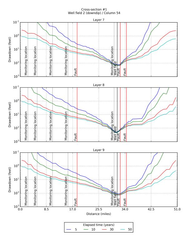
Figure 6-34. Simulated drawdown at 5, 10, 30, and 50 years for model layers 7, 8, and 9 after pumping the up dip Well Field #2 located in PPA #1 at 15,000 AFY as determined by the groundwater model with GHSM-based hydraulic properties for Carrizo-Wilcox Aquifer.
