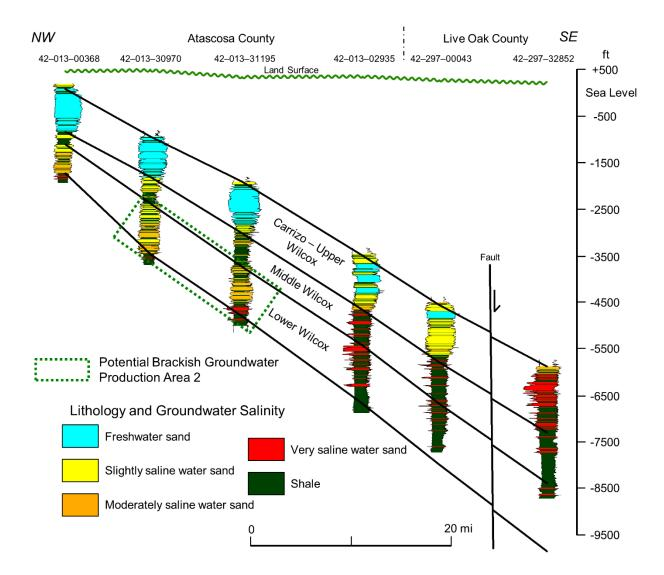
Figure 4-34. Structural cross section C (sea-level datum) showing lithologies and groundwater salinities. Faults and potential brackish groundwater production areas are also shown. See Figure 4-1 for location.
