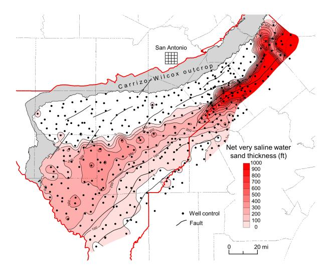
Figure 4-23. Net thickness of sand containing very saline groundwater in the lower Wilcox interval. Fault zones modified from Ewing (1990) and Hargis (2009).
