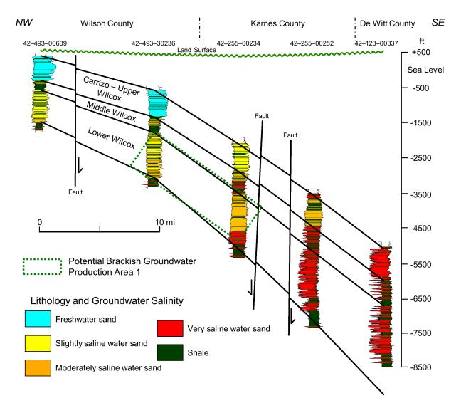
Figure 4-33. Structural cross section B (sea-level datum) showing lithologies and groundwater salinities. Faults and potential brackish groundwater production areas are also shown. See Figure 4-1 for location.
