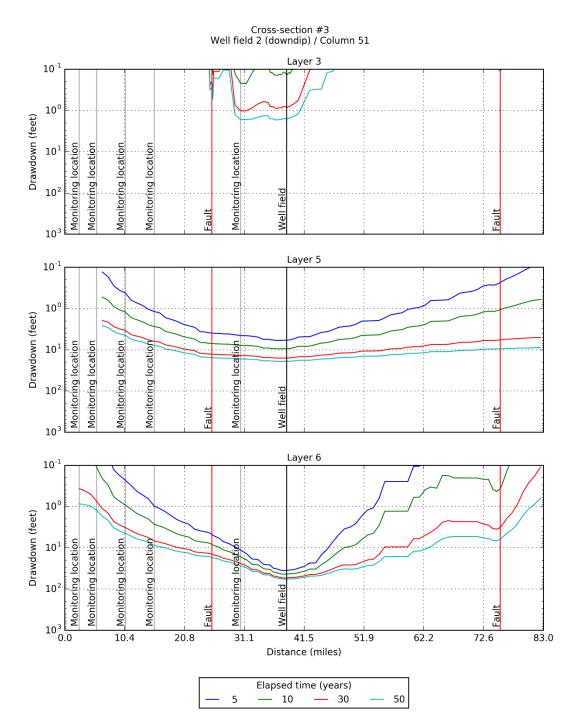
Figure 6-61. Simulated drawdown at 5, 10, 30, and 50 years for model layers 3, 5, and 6 after pumping the up dip Well Field #2 located in PPA #3 at 15,000 AFY produced by the groundwater model with GHSM- based hydraulic properties for Carrizo-Wilcox Aquifer.
