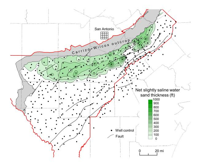
Figure 4-21. Net thickness of sand containing slightly saline groundwater in the lower Wilcox interval. Fault zones modified from Ewing (1990) and Hargis (2009).
