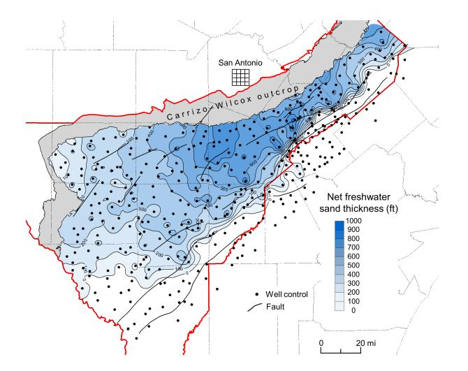
Figure 4-9. Net thickness of sand containing fresh groundwater in the Carrizo–upper Wilcox interval. Fault zones modified from Ewing (1990) and Hargis (2009). Groundwater salinities increase abruptly across some of these regional faults.
