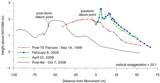
Figure 13. Beach-profile plots from BEG02 in Galveston Island State Park comparing the post-Hurricane lke profile with two prestorm profiles from early 2008 and the post-Tropical Storm Frances profile from September 1998. The old datum point is 0.
