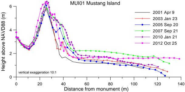
Figure 17. Foredune expansion at MUI01 on Mustang Island.
