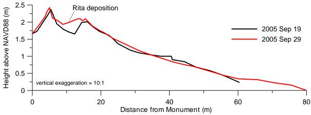
Figure 12. Plot of pre- and post-Rita beach profiles measured at Galveston Island State Park.
