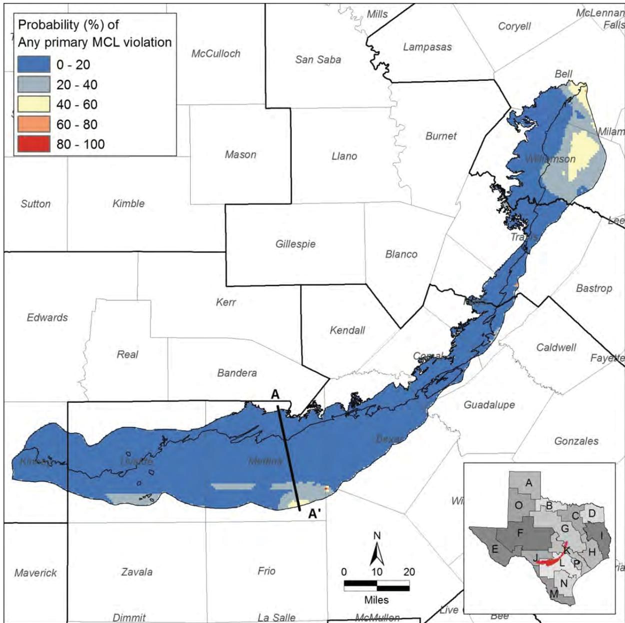
Figure 47. Edwards (BFZ) Aquifer groundwater probability of any primary maximum contaminant level (MCL) violation and cross section schematically illustrating total saturated thickness of the aquifer and depth from land surface.
