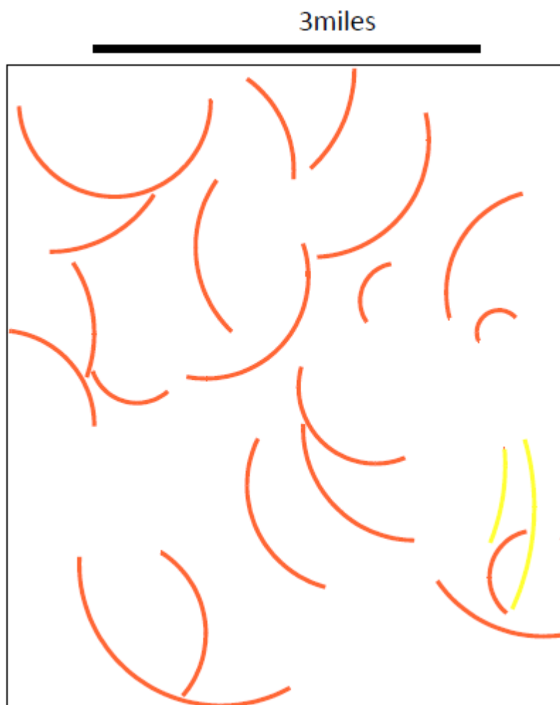
Figure 1.2-10. Map view of interpreted channel morphologies from stratal slicing of the baseline 3-D survey (approximately equivalent to the Tuscaloosa “A-B-C” intervals).
