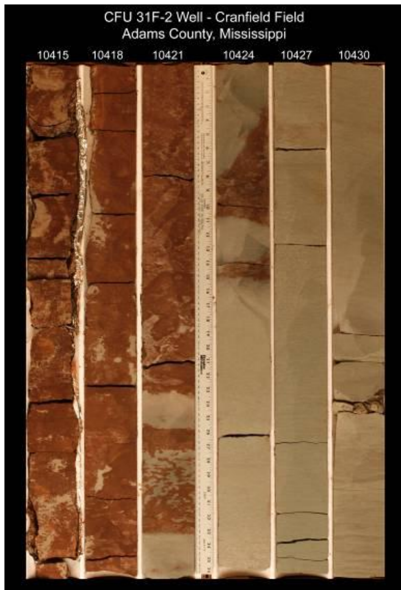
Figure 1.2-6. Overbank mudstone deposits in slatted core from the top of the reservoir interval.
