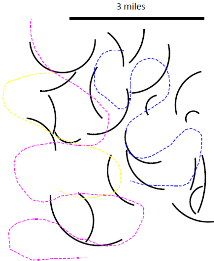
Figure 1.2-7. Interpreted channel morphologies from stratal slicing of the baseline 3-D survey (approximately equivalent to the Tuscaloosa “D-E” interval).
