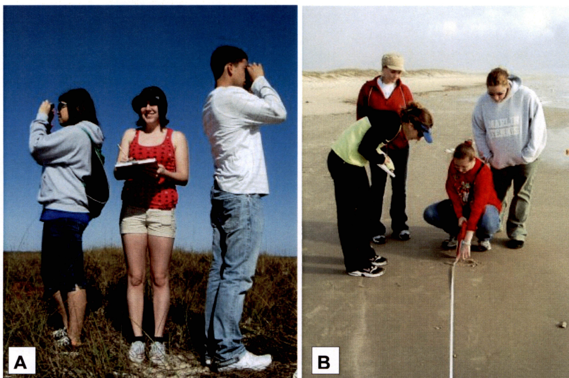
Figure 3. Students (A) using a sighting compass to measure dune orientation and (B) measuring how far along the shoreline the float (an orange) drifted to determine longshore current.
