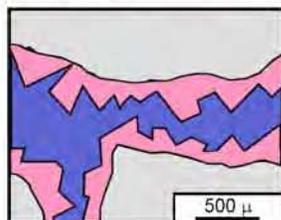
Dolomite type 5: Medium- to coarse-crystalline planar-e dolomite; clear crystals lining void space and fractures filled by late dolomite and/or calcite.
