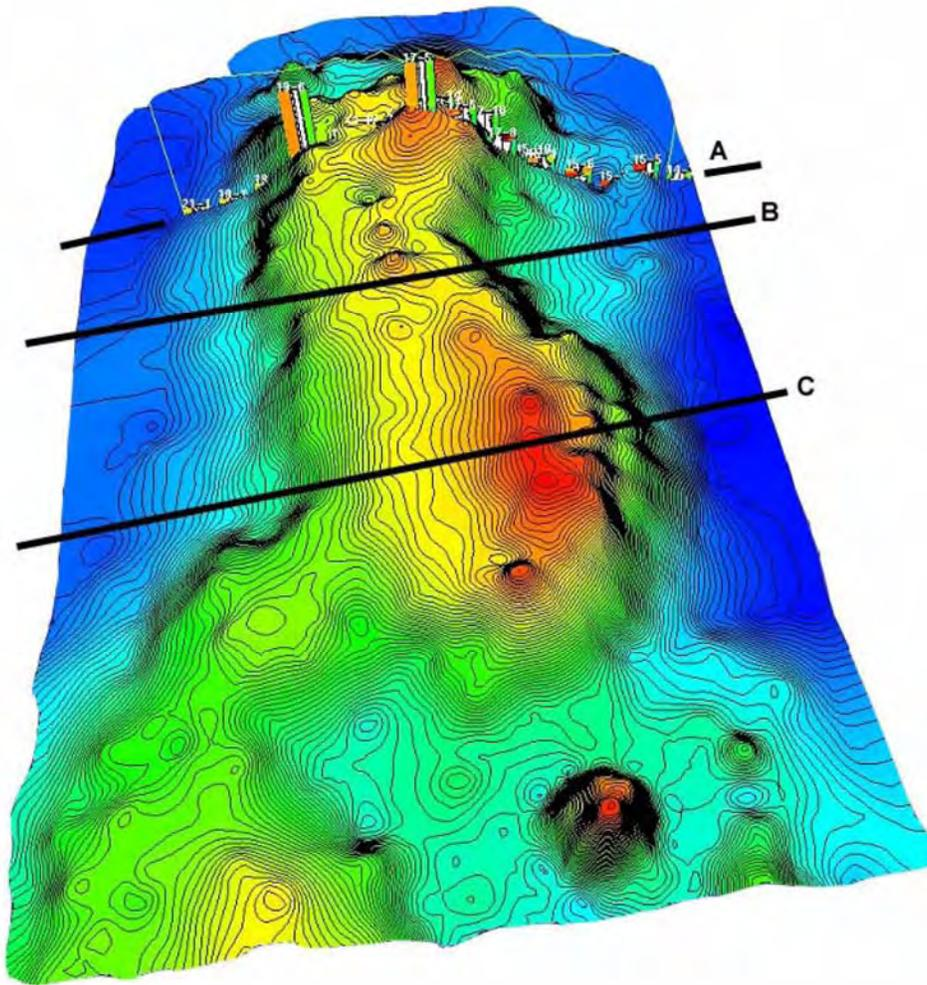
Figure 26. Structure-contour map of the top Virgilian (CISCO) carbonate at SACROC. Note change in architectural style from flat in the south (near C) to more rugose, narrow, and irregular to the north (near A). After Janson and Kerans (2007).
