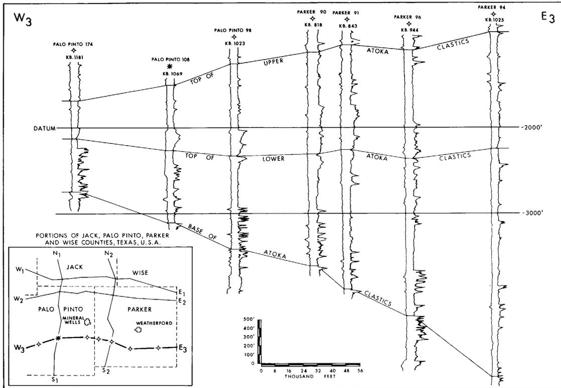
Figure 17. West-east SP- and resistivity-log correlation of Atokan-age units in Palo Pinto and Parker Counties (after Ng, 1979). According to upper and lower log picks of Ng (1979), lower Atokan siliciclastics appear to thin and onlap westward; however, the high-resistivity log interval is relatively uniform in thickness and does not indicate substantial thinning or onlap. The upper Atokan shale-dominated interval is equivalent to the Smithwick Formation.
