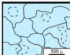
Dolomite type 6: Coarse- to very coarse crystalline nonplanar-a dolomite; dark, inclusion-rich crystals, with serrated, irregular, curved, or otherwise distinct boundaries; undulose extinction; vague nonmimic replacement of grains.
