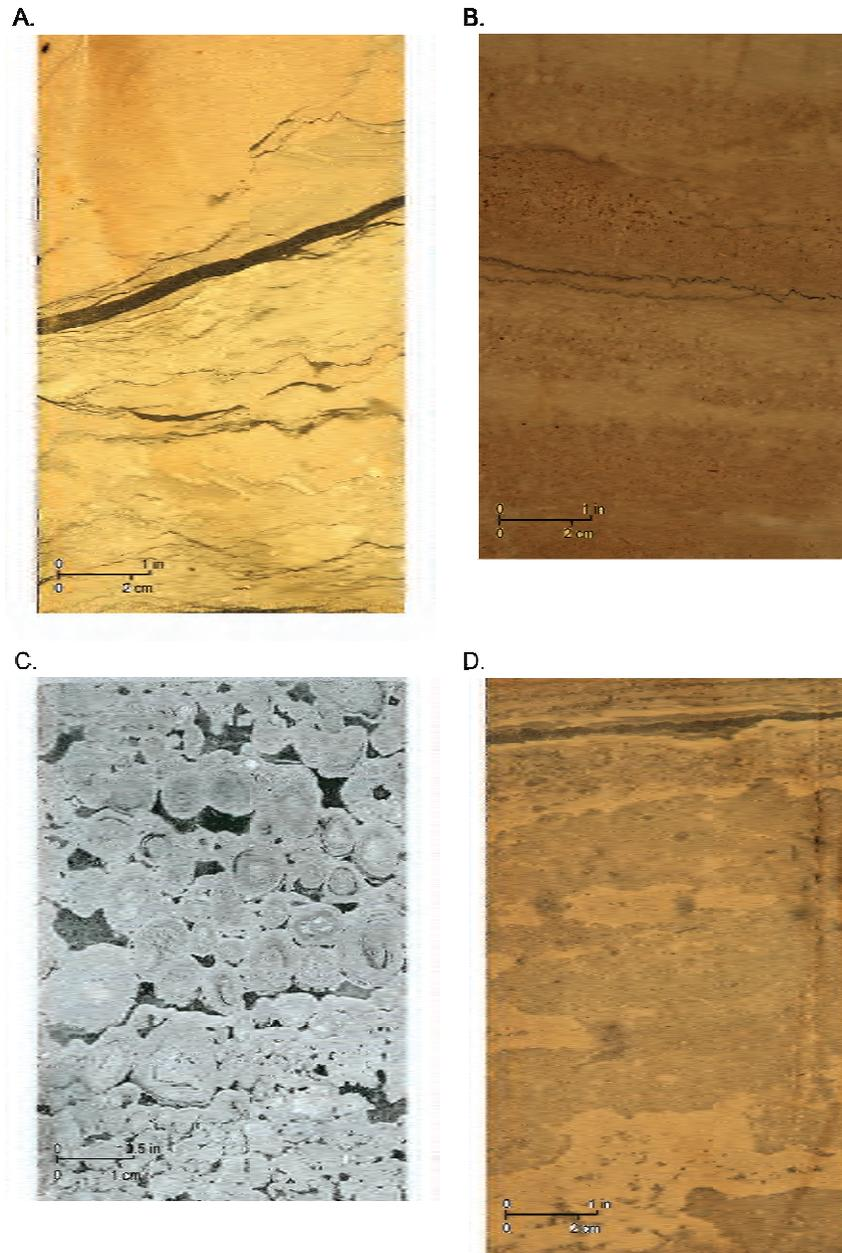
Figure 17. Artesia Group dolostone facies: (A) Queen shoal cross-laminated grainstone; (B) Queen tidal-flat packstone; (C) Yates shelf-crest shoal, pisolite grainstone; and (D) Queen lagoon bioturbated wackestone to packstone. Cores A, B, and D are from HSA No. 475 well, Ward-Estes, Ward County; C is from Gulf PDB-04 well, Eddy County, New Mexico.
