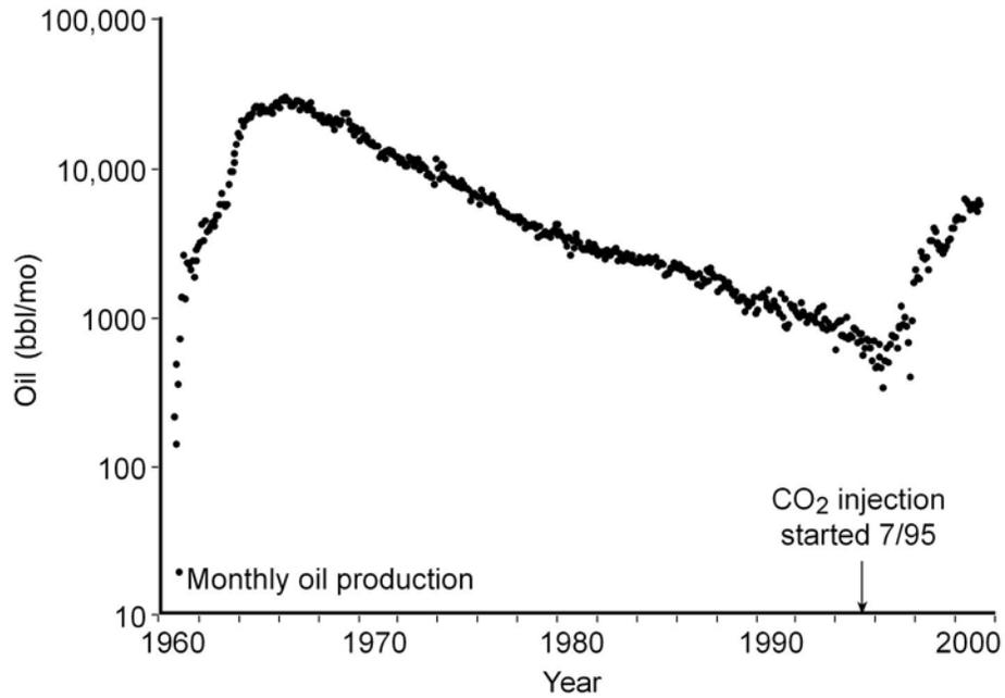
Figure 33. Monthly oil production from East Ford Unit (Bell Canyon), showing production improvement after change from primary to secondary production with initiation of CO<sub>2</sub> injection in 1995. Field location shown in figure 2. From Dutton and others (2003).
