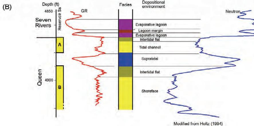
Figure 30. McFarland reservoir: (A) structure map on top of the Queen Formation; State University Units No. 1 and 2 are outlined; and (B) representative well log of the upper Queen productive-sandstone interval. Production is from interpreted tidal-channel and shoreface (probable beach ridge) sandstone. Supratidal carbonate provides baffle between productive sandstones. Modified from Holtz (1994).
