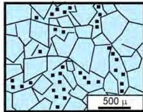
Dolomite type 4: Medium- to coarse-crystalline planar-e mosaic dolomite; clear or cloudy core, clear rim texture; not replacement features; occurs in mottles or breccias or near stylolites.
