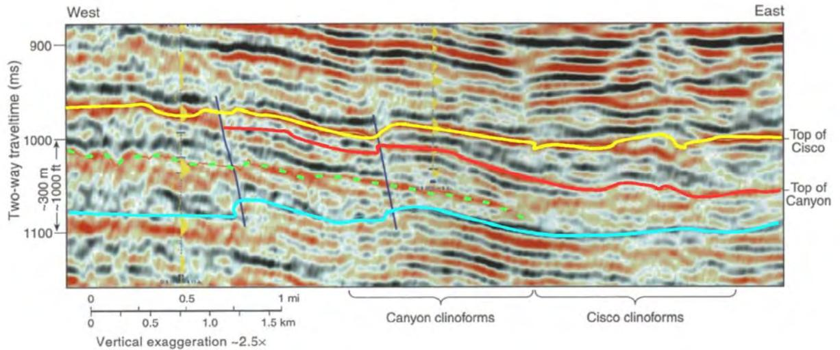
Figure 40. West-to-east (basinward) dip-section seismic line through South Dagger Draw field, Eddy County, New Mexico (after Tinker and others, 2004). Yellow line is interpreted top of Cisco (Virgilian), whereas red line is top of Canyon (Missourian) and blue line is possible base of Canyon. Note low-angle sigmoidal, clinoformal architecture of both successions.
