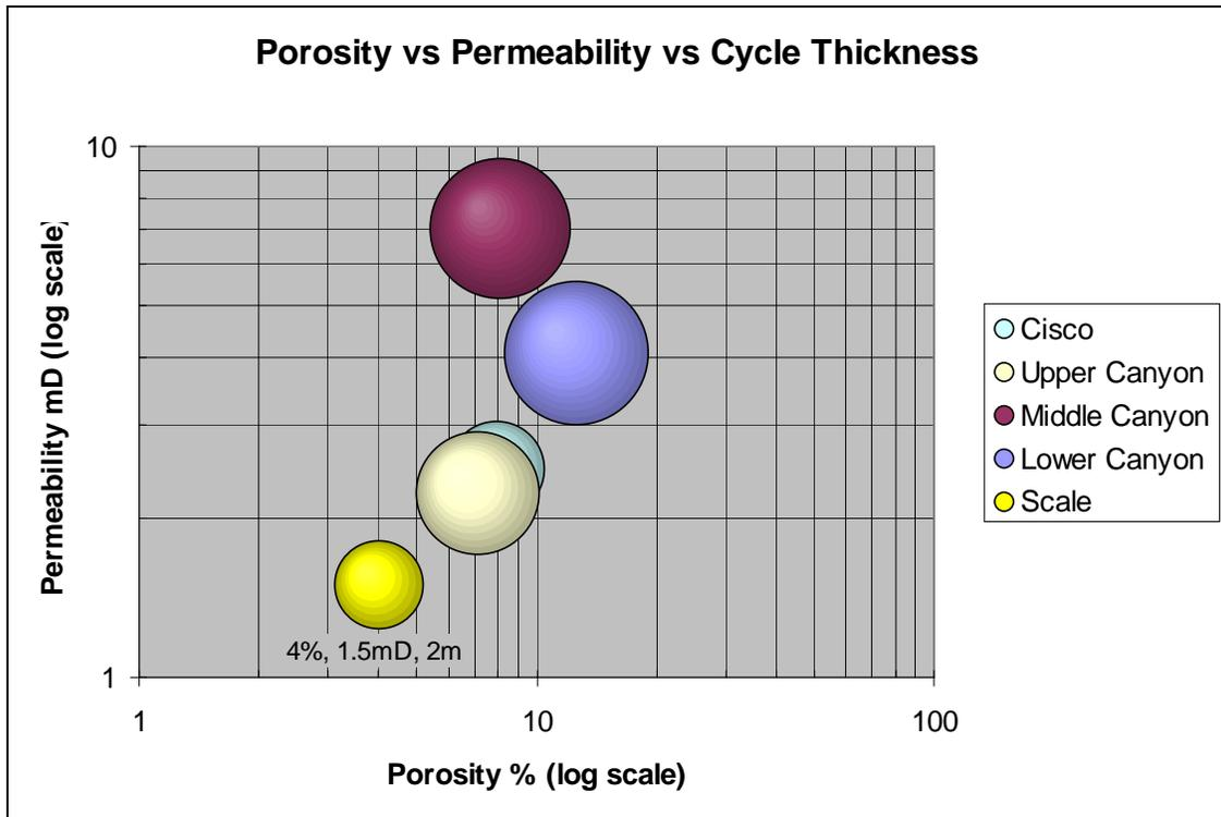
Figure 44. Summary bubble chart of porosity, permeability, and cycle thickness for Missourian and Virgilian carbonate succession in South Andrews field area (data from Saller and others, 1999a). Bubble area corresponds to cycle thickness. Overall, the lower Canyon interval (lower Missourian) has the best reservoir quality. Values used are averages of three wells' data. Note that original values did not include cycles in sequences with porosity less than 4 percent.
