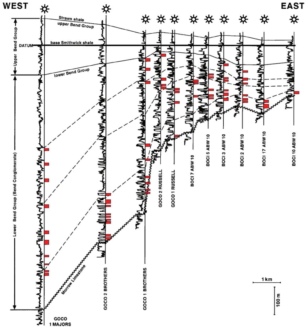
Figure 12. Gamma-ray log west-east correlation of entire Atokan interval (Bend and Smithwick Formations) within Broken Bone Graben. Small red bars on right-hand side of each well log indicate producing reservoir-quality sandstones. Note large number of reservoir-quality sandstones within lower unit that are disconnected from reservoir-grade intervals on upper flank of the structure (after Brister and others, 2002).
