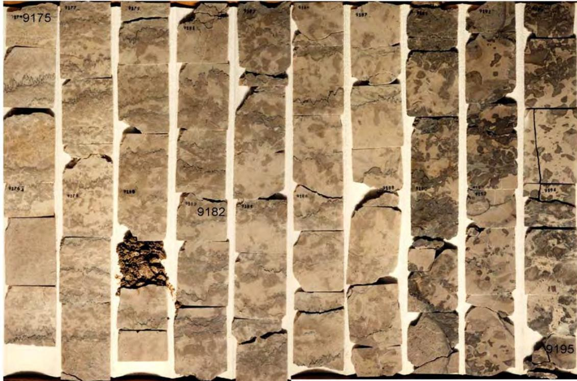
Figure 36. Upper Canyon core photographs, core description, and isotopic profiles (after Saller and others, 1999a, b). Note extensive textural alteration throughout the interval, which makes picking cycle boundaries difficult. Below 9,189 ft the interval seems to be highly brecciated, which may suggest some form of debris flow not indicated on the original interpretation.
