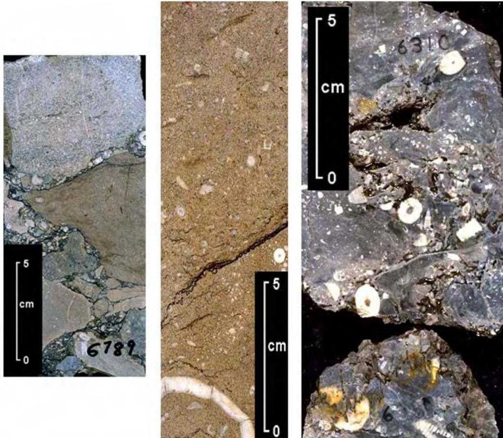
Figure 24. Core slab photos of typical Virgilian (Cisco) facies. Left photograph is a debris flow containing large lithoclasts and crinoidal debris. Middle image is crinoidal turbidite with steeply dipping beds to the left. Right photograph illustrates a stromatactid mud-mound facies with abundant, large, crinoid debris. After Janson and Kerans (2007).
