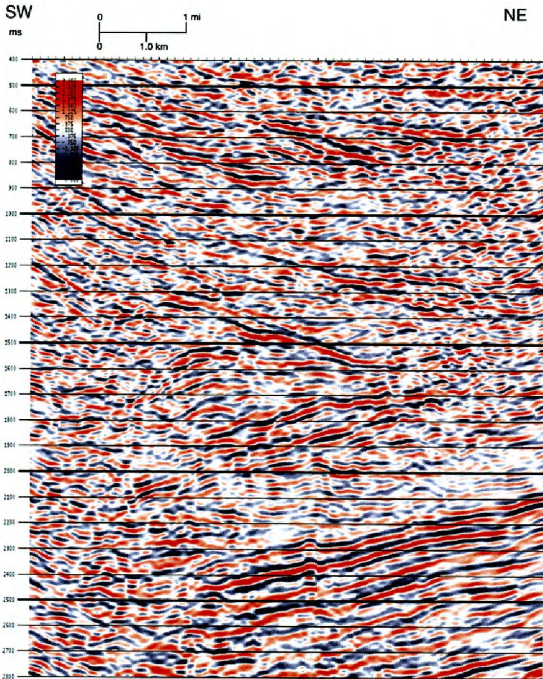
Figure 41. Uninterpreted seismic line trending SW-NE through Pakenham field (Terrell County). Seismic line illustrates structural complexity present in this part of Val Verde Basin. Figure should be compared with figure 37 for geologic and structural interpretation of this area. Figures 39 and 40 illustrate alternative, seismic-based, geologic and structural interpretations of the area.
