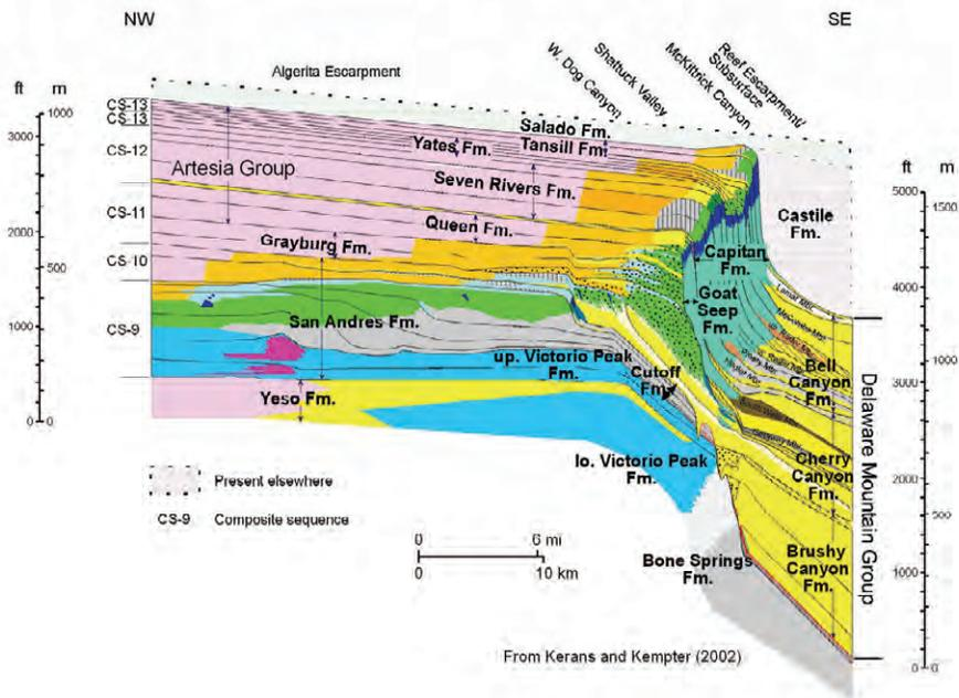
Figure 4. Northwest-southeast schematic cross section of uppermost Leonardian to Ochoan strata, Guadalupe Mountains area, showing formations, carbonate-bearing members of the Delaware Mountain Group, and boundaries of high-frequency sequences and composite sequences. Modified from Kerans and Kempter (2002).
