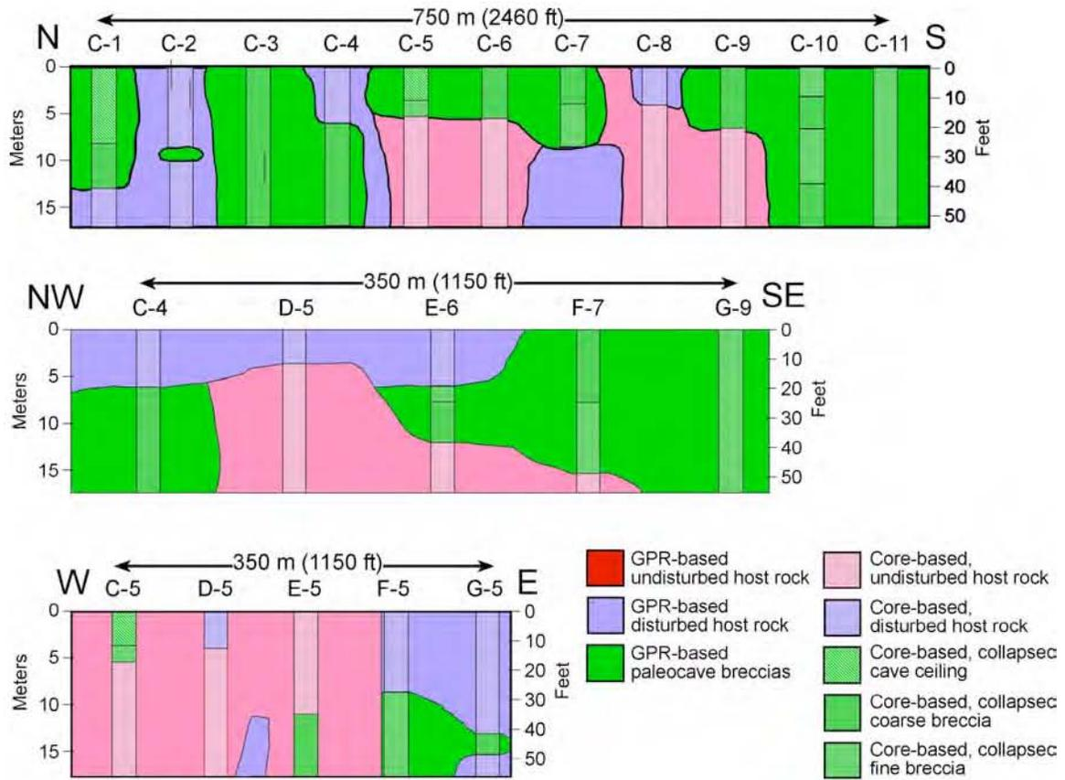
Figure 38. Simplified facies cross sections using core and GPR data. See Figure 35 for location of wells used on lines of sections. From Loucks et al. (2004).
