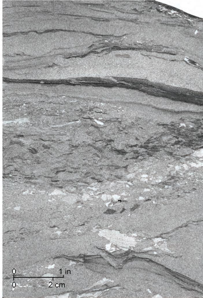
Figure 24. Queen intraclastic, fine-grained sandstone of possible tidal-channel origin. This sample lies below a marine-derived cycle-top dolostone bed and may record a transgressive ravinement surface. Similar samples elsewhere may mark high-frequency sequence boundaries within siliciclastic intervals where no marine-derived sediment was deposited during the highstand depositional phase (HSA No. 475 well, 2945.5 ft, North Ward-Estes reservoir, Ward County).
