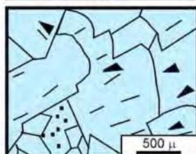
Dolomite type 7: Coarse- to very coarse crystalline nonplanar-c dolomite milky white to clear crystals with undulose extinction and curved crystal faces (saddle dolomite); void filling; associated with authigenic quartz and late calcite.
