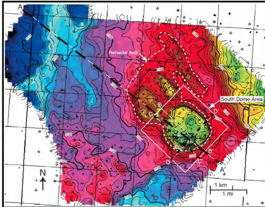
Figure 17. Seismic structure map of the Upper Pennsylvanian-lowest Permian carbonate across Reinecke field at 5-m contours. Seismic lines A-A' (Figure 16), C-C' and D-D' (figure 18) illustrated by thick dashed black line. All three seismic cross sections go through main mound area and have data down to the Ordovician (Ellenburger).
