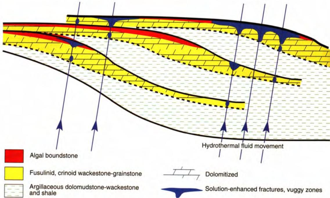
Figure 56. Conceptual dolomitization model for Missourian and Virgilian succession at Dagger Draw, Northwest Shelf. Dolomitization is thought to be diagenetically late, and fluids migrated into the succession from below via faults and fractures. After Tinker and others (2004).
