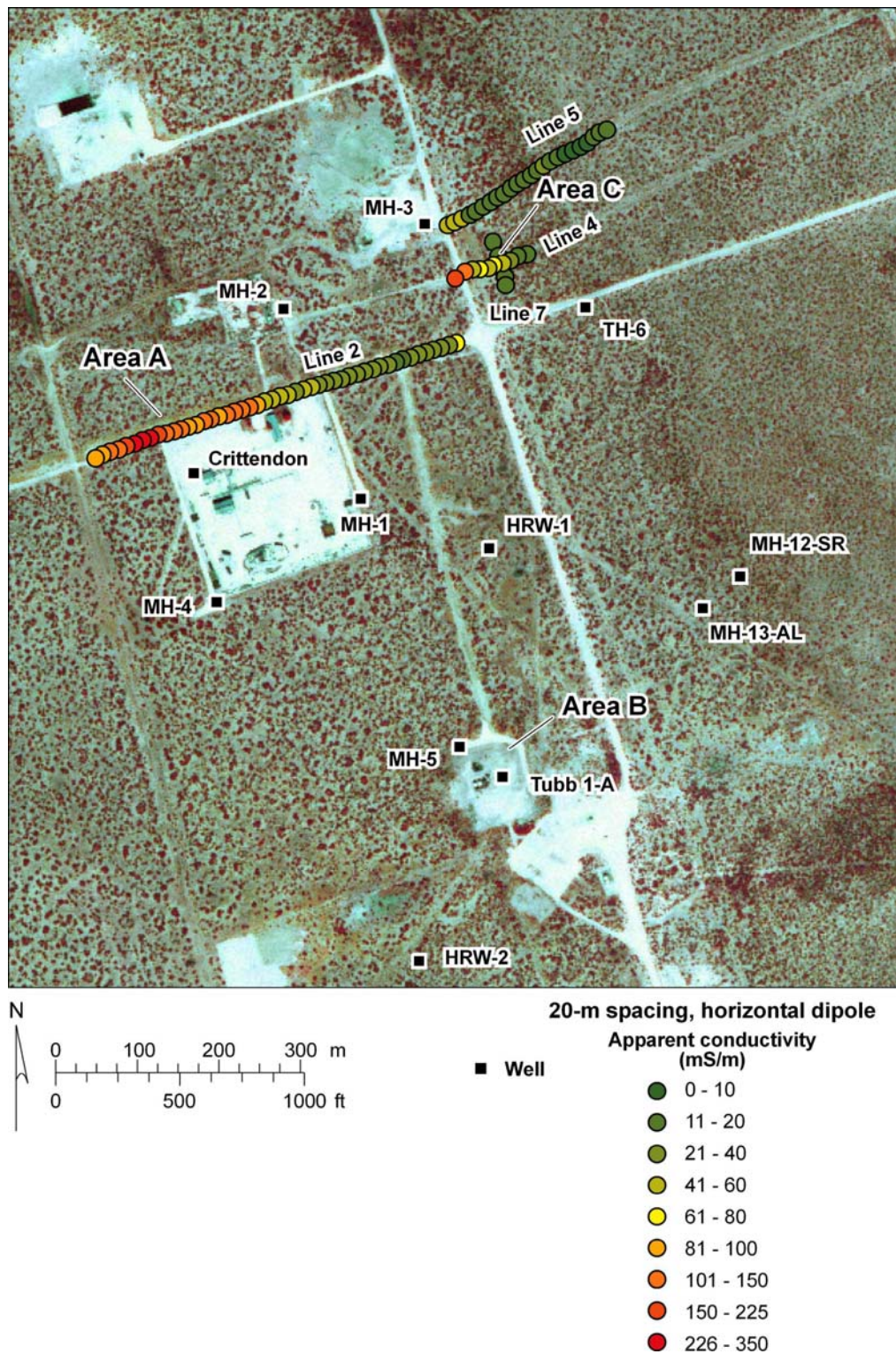
Figure 4. Apparent ground conductivities measured along EM lines 2, 4, 5, and 7 using a Geonics EM34-3 instrument operating at a 20-m coil separation, 1600 Hz primary frequency, and horizontal dipole coil orientation. The nominal exploration depth reaches 12 m (table 1), but the upper third of that depth range is the most significant contributor to the measured value.
