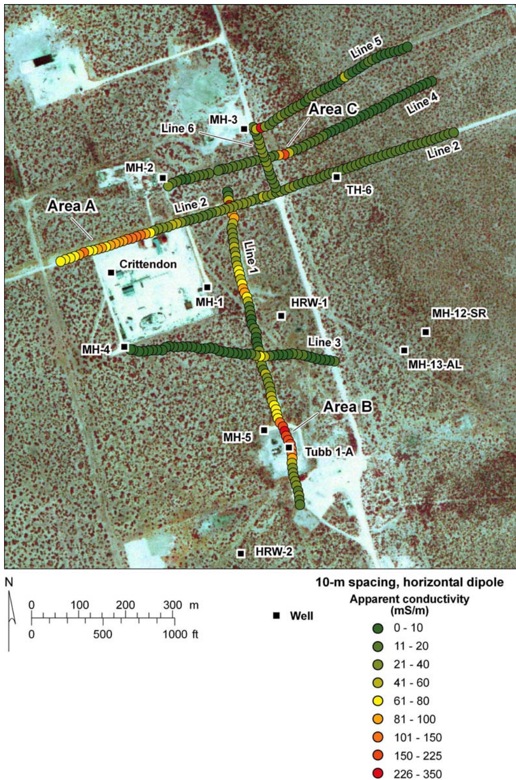
Figure 2. Apparent ground conductivities measured along EM lines 1 through 6 using a Geonics EM34-3 instrument operating at a 10-m coil separation, 6400 Hz primary frequency, and horizontal dipole coil orientation. The nominal exploration depth reaches 6 m (table 1), but the upper third of that depth range is the most significant contributor to the measured value.
