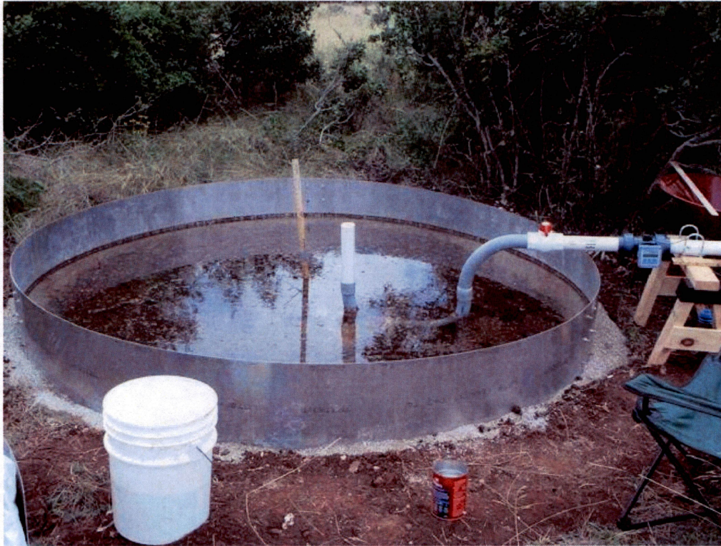
Figure 4. Typical ring infiltrometer installation.
