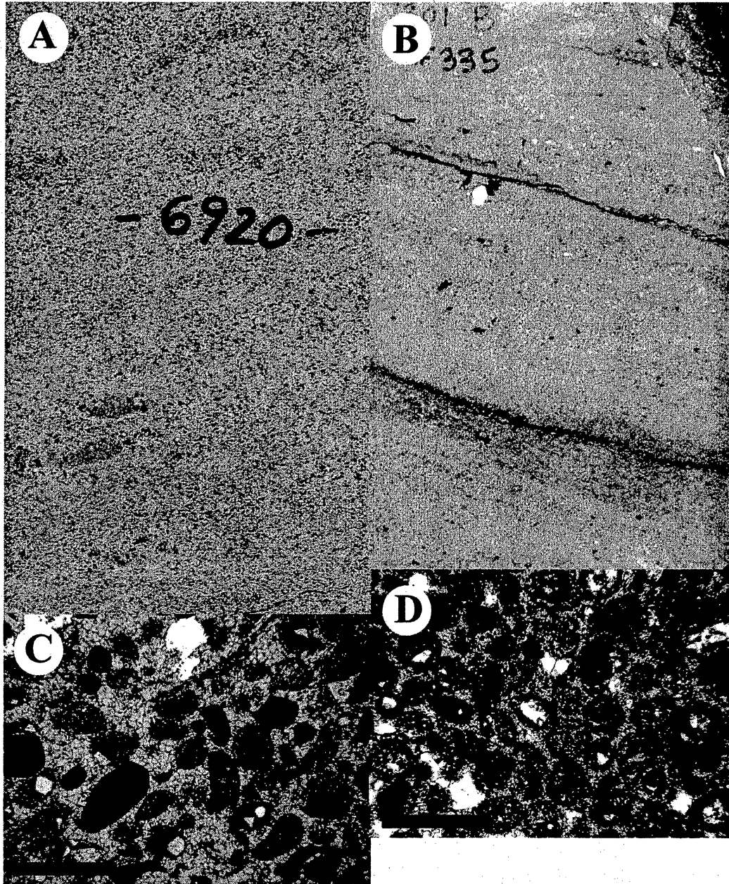
Figure 15. Core and thin-section photomicrographs of Lower Clear Fork and Abo grainstones. A. Slab photo of Lower Clear Fork ooid grainstone showing cross laminations. FCU 6122, depth: 6,920 ft. Core is 10 cm wide. B. Slab photo of Abo skeletal grainstone showing inclined laminations. FCU 7322, depth: 7,301 ft. Core is 10 cm wide. C. Photomicrograph of Lower Clear Fork ooid limestone grainstone showing oomoldic pores. FCU 5927, depth: 6,913 ft. Scale bar is 1 mm. D. Photomicrograph of Lower Clear Fork ooid dolostone grainstone wackestone showing interparticle and minor moldic pores. FCU 4828, depth: 7,137 ft. Scale bar is 1 mm.
