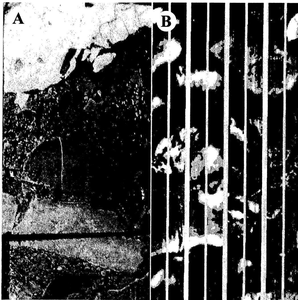
Figure 41. Image log and core photo images of polymict karst conglomerate. Wichita. Core: FCU 6122, depth: 7,201 ft. Image log: FCU 2564, depth: 7,171–7,182 ft. Core is 4 inches wide.
