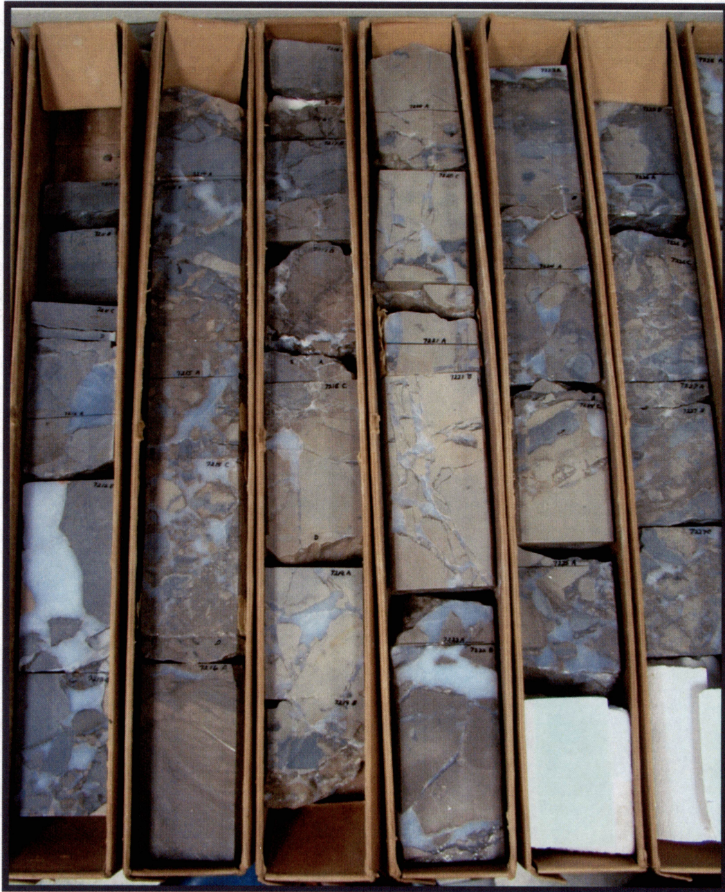
Figure 32. Core slab box photo of breccias developed at the Abo/Wichita contact in FM-1 core. Amoco University Consolidated # IV-25, depths: 7,211–7,228 ft. Core pieces are 4 inches wide.
