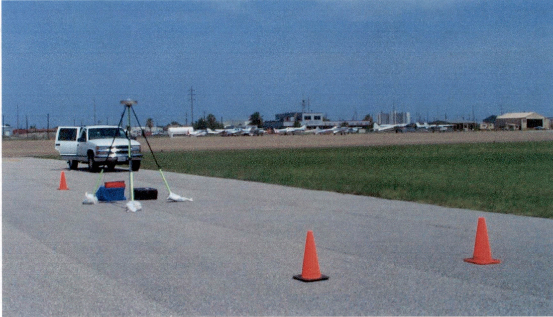
Figure 3. Geodetic receiver and fixed height pole with antenna as base station setup on unused taxiway at Scholes Field in Galveston, Texas.
