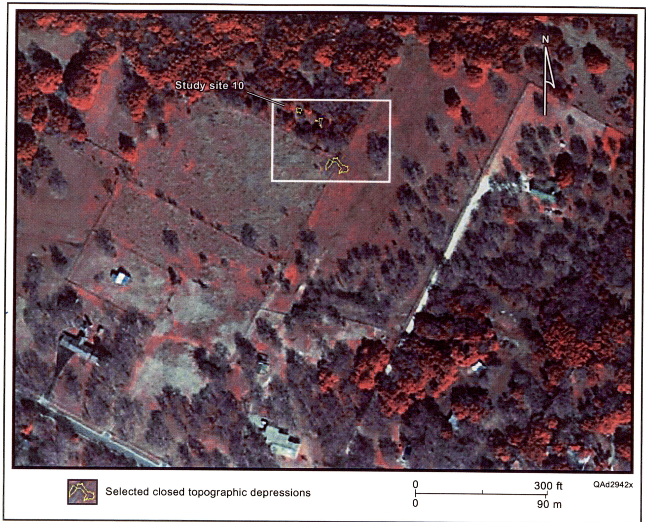
Figure 14. Location of selected, remotely sensed, closed topographic depressions at study site 10 that are superimposed on high-resolution, pan-sharpened QUICKBIRD satellite imagery. The remotely sensed, closed topographic depressions were identified from the topographic map constructed from lidar data shown in figure 13.
