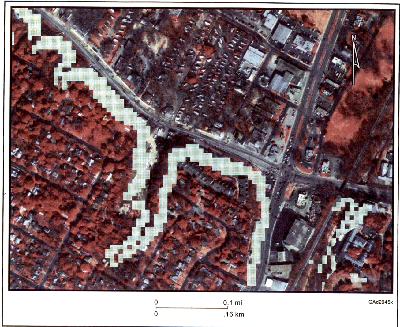
Figure 17. Close-up of areas mapped within the Del Rio-Buda-Eagle Ford Formations in the northeast part of study site 11 that have ground slopes between 12^{\circ} and 52^{\circ} (patterned area). These higher slope areas are superimposed on a pan-sharpened, high-resolution QUICKBIRD satellite image for visualization of natural and cultural features. Geologic setting shown in figure 15.
