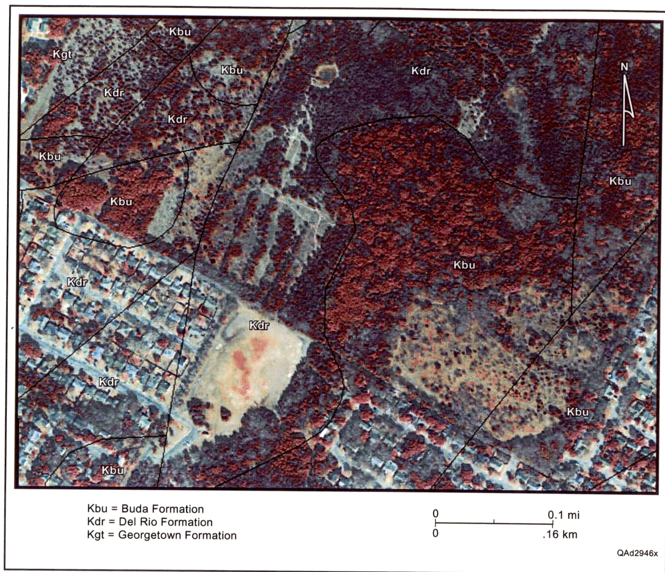
Figure 18. Geology of study site 12 within the Del Rio-Buda-Eagle Ford Formations outcrop belt. Geology is superimposed on a pan-sharpened, high-resolution QUICKBIRD satellite image for visualization of natural and cultural features. Geologic setting shown in figure 15.
