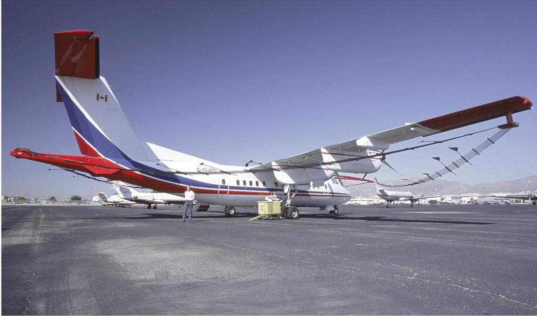
Figure 17. Fugro Airborne Surveys' Megatem II airborne TDEM system in El Paso, Texas, August 22, 2001. The transmitter loop is attached to the wing tips and booms at the front and rear of the aircraft. Cables trailing the aircraft tow the EM receiver and magnetometer (not shown). Photograph by David M. Stephens.
