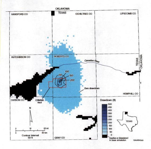
Figure 4. Drawdown of water levels in the Ogallala aquifer in 2050 in the vicinity of Roberts County, Texas, owing to the "CRMWA" groundwater project assumed to initially pump 30,000 acre-feet per year. Drawdown determined from the difference between water levels simulated with versus without the project. Pumping was assigned to 16 model cells, representing 23 wells, with 7 model cells have 2 wells.
