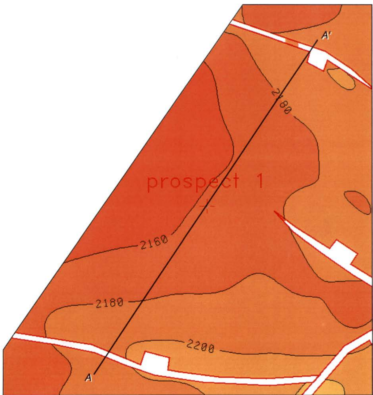
Figure 44. Prospect 1 location posted on a time-structure map of MFS16 (contour interval = 20 ms). The structure map depicts subsurface topography at the L sand reservoir level.
