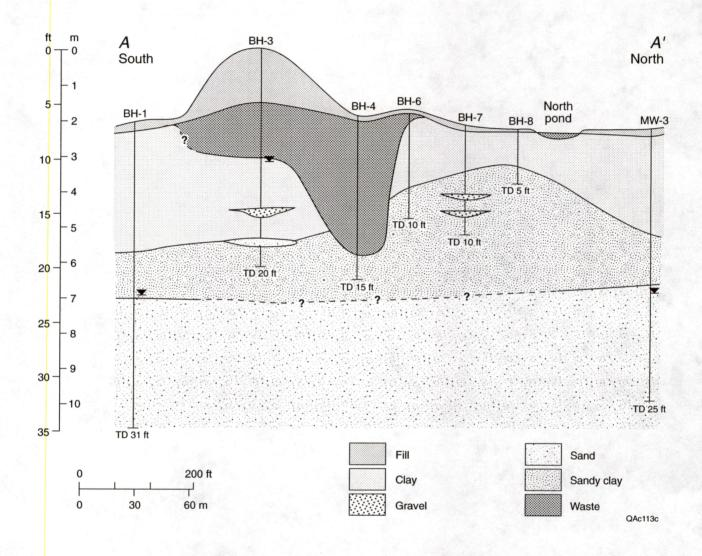
Figure 4.4. South-north cross section A–A′ of the waste-disposal area and local stratigraphy. Line of section shown in figure 3.2. Initial water levels shown.
