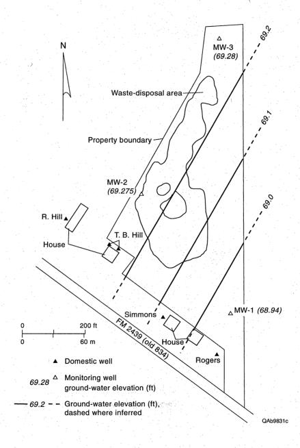
Figure 4.8. Ground-water elevation data from the uppermost aquifer beneath the Roeling Vacuum site, July 31, 1997.
