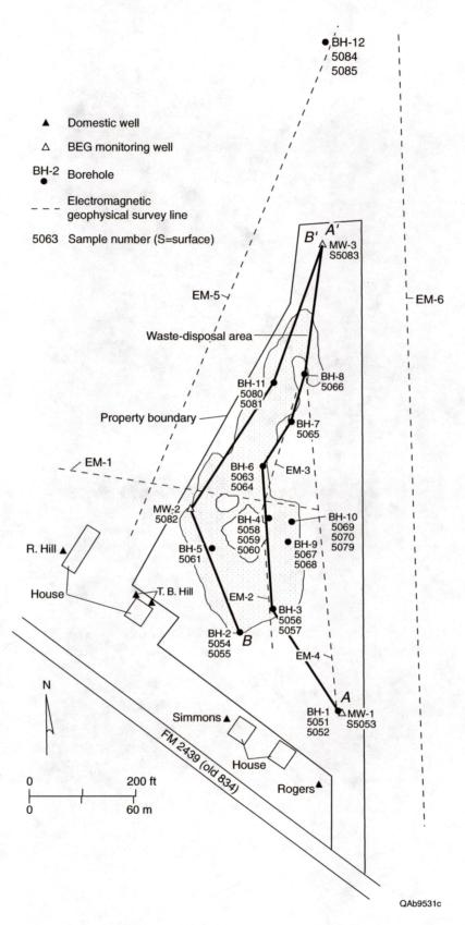
Figure 3.2. Domestic-well, monitoring-well, borehole, and EM survey line locations at the Roeling Vacuum site, including borehole sample numbers. Section lines A–A' and B–B' shown in figures 4.4 and 4.5.
