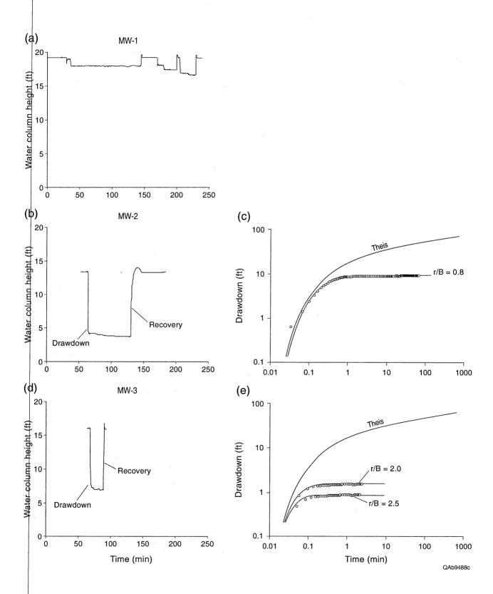
Figure 4.9. Graphical results of drawdown tests.
