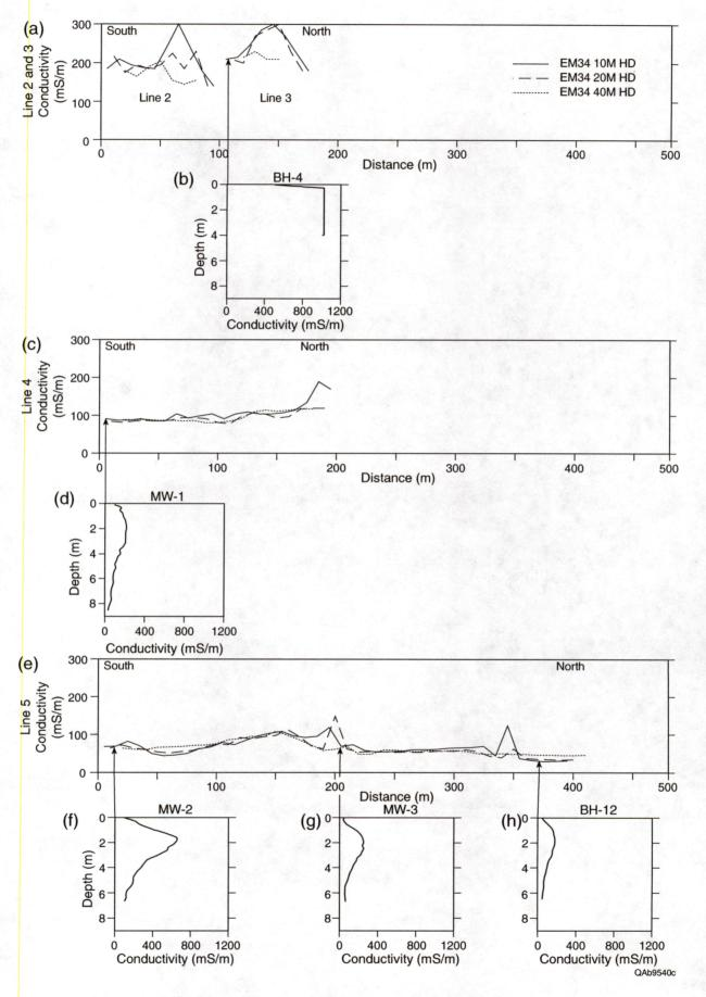
Figure 4.3. EM 34-3 and EM 39 combined electromagnetic geophysical-survey data.
