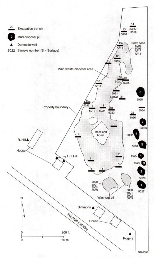
Figure 3.1. Trench and surface impoundment sample locations, Roeling Vacuum site.
