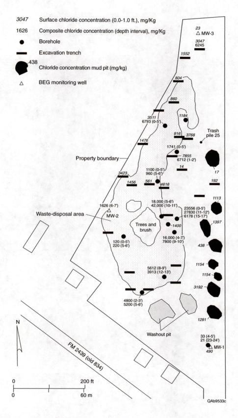
Figure 4.7. Results of chloride analyses in boreholes, trenches, and surface soils.
