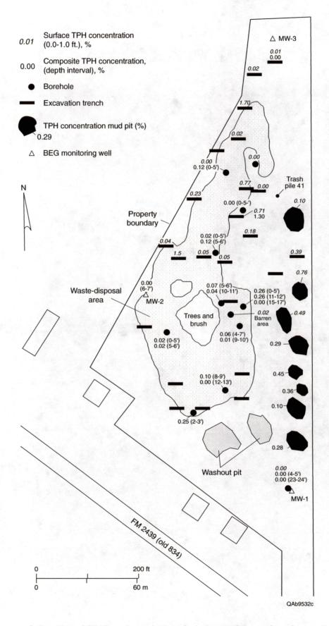
Figure 4.6. Results of TPH analyses in boreholes, trenches, and surface soils.
