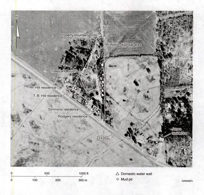
Figure 2.2. Layout of the Roeling Vacuum site, showing surrounding property use, domestic wells, and the approximate property boundary.
