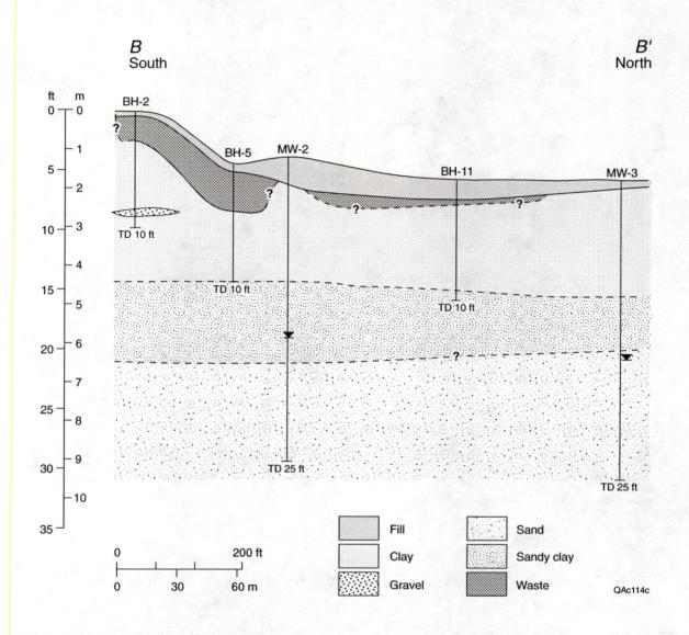
Figure 4.5. South-north cross section B–B' of the waste-disposal area and local stratigraphy. Line of section shown in figure 3.2. Initial water levels shown.
