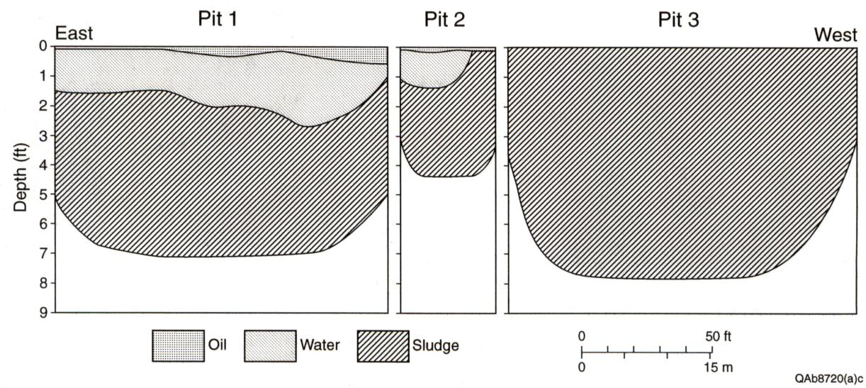
Figure 3. Profile of pit-fluid layers.
