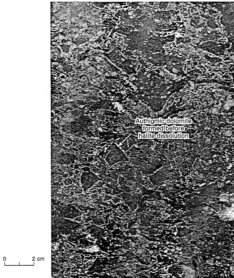
Figure 26 (cont.). Typical textures diagnostic of insoluble residue formed under conditions of regional low-angle salt dissolution and passive letdown of overlying strata. (c) Insoluble residue formed by dissolution of mudstone-halite mixtures. Gruy Federal Rex White core, 613 ft below datum.
