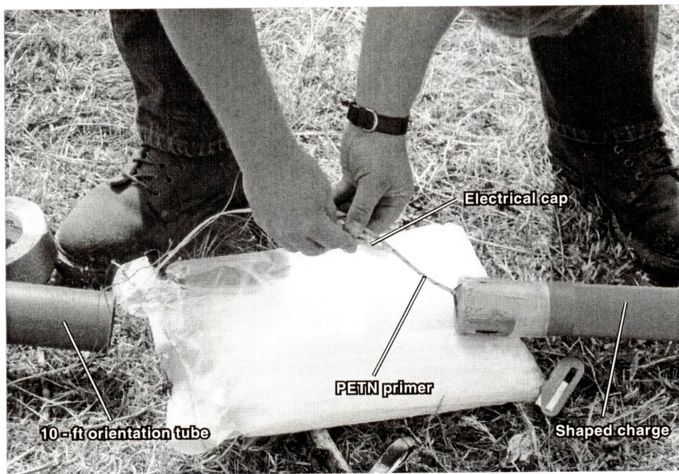
Figure 44. Low-velocity-emulsion shaped charge being prepared for detonation.
