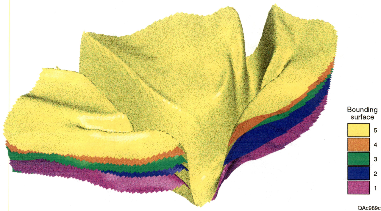
Figure 29. Bounding surfaces stacked to form the model. This view shows the purple, blue, green, orange, and yellow surfaces.
