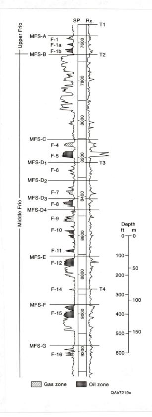
Figure 3. Type log from well 74-3 in Umbrella Point field. SP and shallow resistivity curves shown. MFS horizons correspond to those shown in cross section A–A'. Zone designations indicated for productive interval. Dominant produced fluid type indicated by color.
