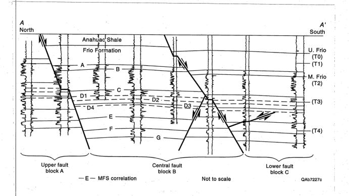
Figure 4. Dip-normal cross section of Umbrella Point field. Line of section shown in figure 1. MFS correlations marked by letter. High-frequency cycles indicated by designations D1, D2, D3, and D4.
