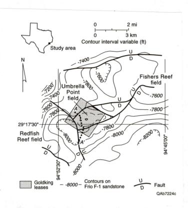
Figure 1. Semiregional structure map contoured on the top of the Frio Formation showing the geologic context of Umbrella Point field. Other similar Frio sandstone fields shown.
