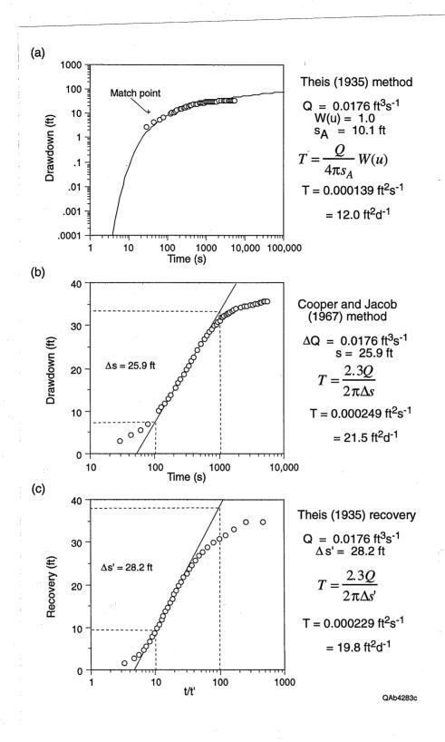
Figure 9. Interpretation of pumping test results at B007 in Fort Wolters using the (a) Theis method, (b) Jacob method, and (c) Theis recovery method.
