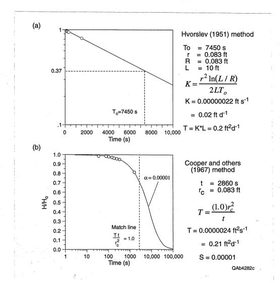
Figure 6. Interpretation of bail test results at WOLTERS-1 in Fort Wolters using the (a) Hvorlslev (1951) method and (b) Cooper and others (1967) method.
