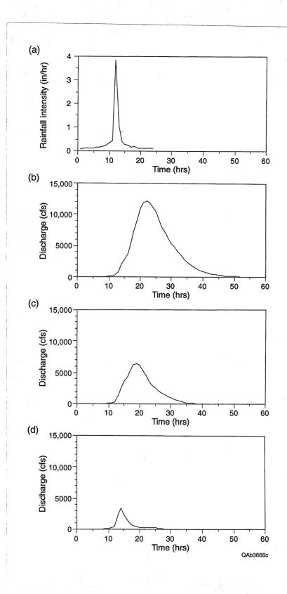
Figure 17. Flood hydrograph analysis of Fort Wolters, including (a) 100-yr 24-hr SCS Type II distributed rainfall intensity and the 100-yr flood hydrographs near the camp boundary of (b) Rocky Creek (point A, fig. 15), (c) Rippy Branch (point B, fig. 15), and (d) a northwest tributary to Rocky Creek (point C, fig. 15).
