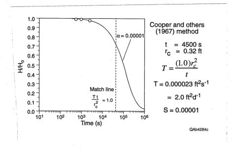
Figure 8. Interpretation of bail test results at FWT-B003 in Fort Wolters using the Cooper and others (1967) method.
