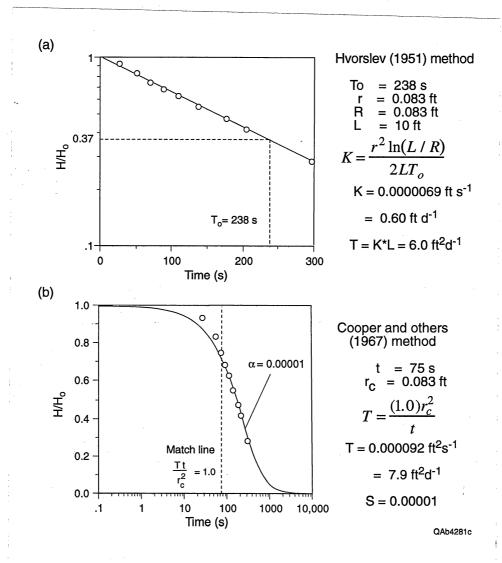
Figure 7. Interpretation of bail test results at WOLTERS-2A in Fort Wolters using the (a) Hvorlslev (1951) method and (b) Cooper and others (1967) method.
