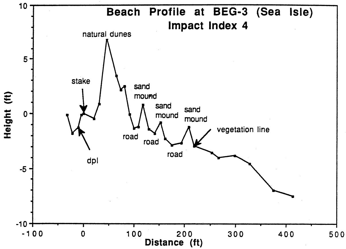
Figure 3. Beach and dune profile at BEG-3 showing substantial modifications to the dune system caused by beach maintenance activities. The high natural dunes formed after Hurricane Alicia. Subsequent construction of sand mounds seaward of the backbeach road and episodic seaward movement of the road and sand mounds have resulted in major modifications to the backbeach and dune system.
