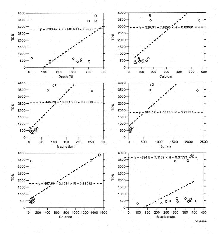
Figure 11. Relation of total dissolved solids in the Edwards and associated limestones aquifer with depth and anion-cation analyses from water wells nearby Camp Mabry.
