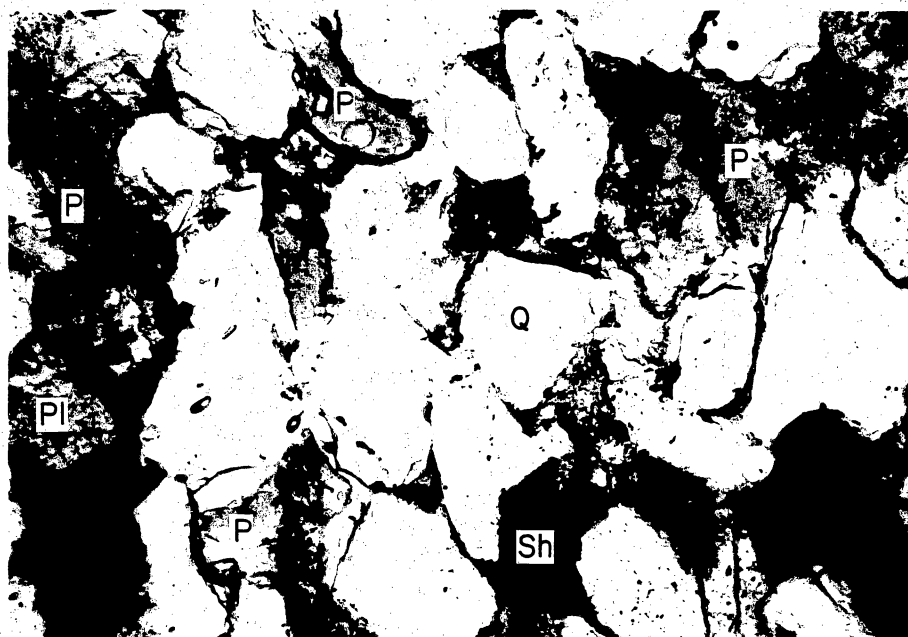
Figure 17. Photomicrograph of abundant secondary porosity (P) produced by dissolution of clay-rich rock fragments. Framework grains include quartz (Q), plagioclase (Pl), and shale rock fragment (Sh). From Forest Winch-State No. 4 (Lobo 2, 9,330 ft). Horizontal dimension of photo is 1.3 mm.
