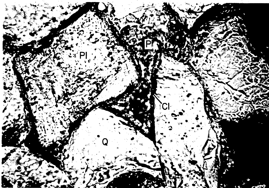
Figure 14. Photomicrograph showing chlorite grain-rimming cement (Cl), primary porosity (P), and quartz (Q) and plagioclase (Pl) framework grains. From Forest Winch-State No. 4 (Lobo.1, 8,869 ft). Horizontal dimension of photo is 0.5 mm.
