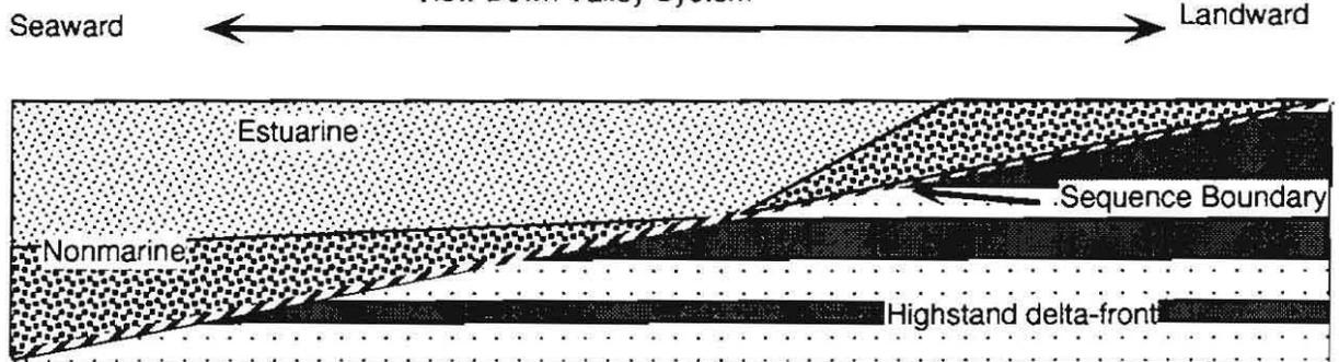
**Figure 23**—Objective criteria for distinguishing incised valley-fill deposits from distributary channellbelt deposits
