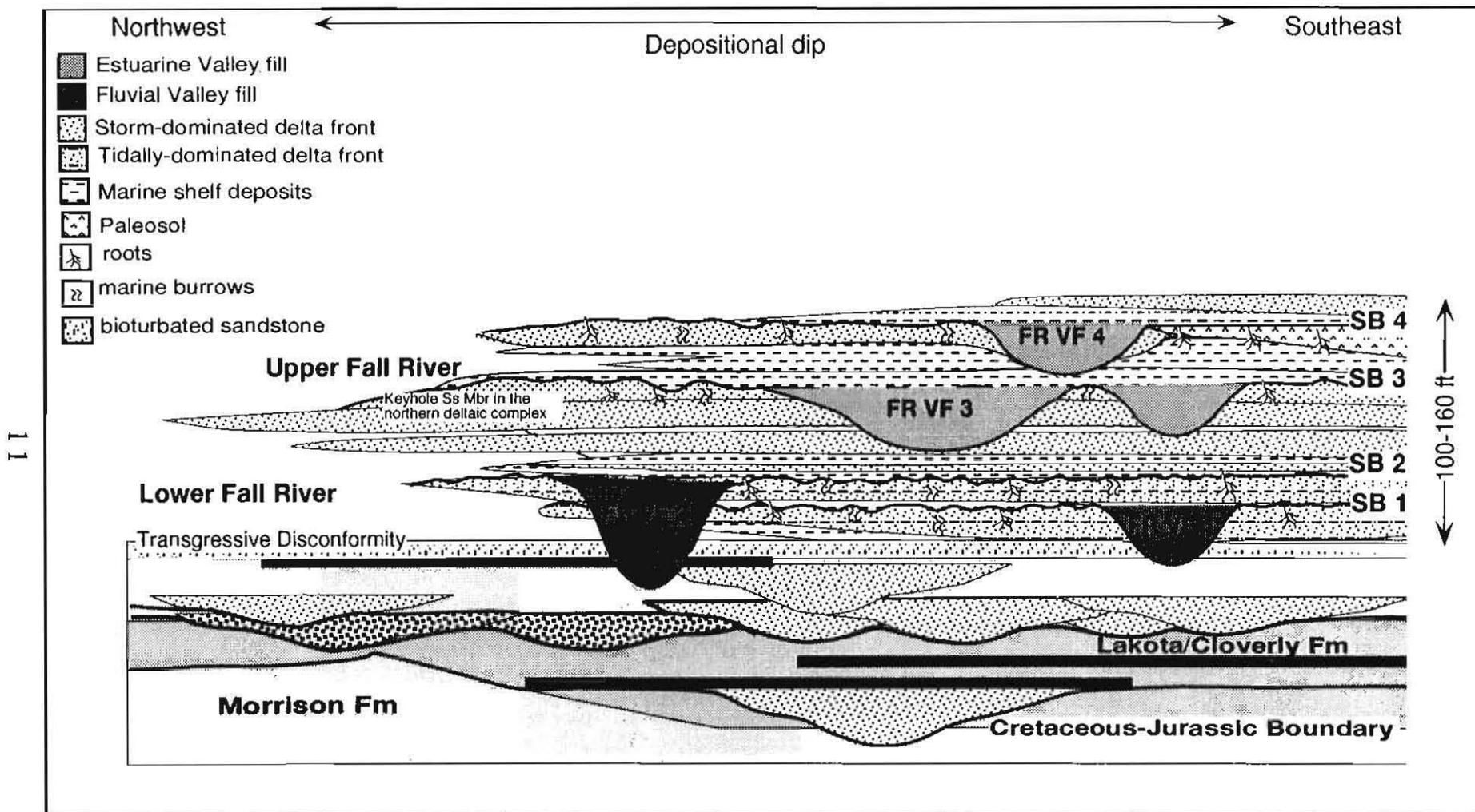
**Figure 5**—Schematic stratigraphic cross section across the Black Hills showing the arrangement of shallow-marine and valley-fill facies tracts in short-term stratigraphic cycles that comprise unconformity-bounded depositional sequences in the Fall River Formation. In the Black Hills region, these sequences are correlated across two deltaic complexes that are separated by a paleohigh, the Belle Fourche Arch. The northern deltaic complex contains the Keyhole Sandstone Member.
