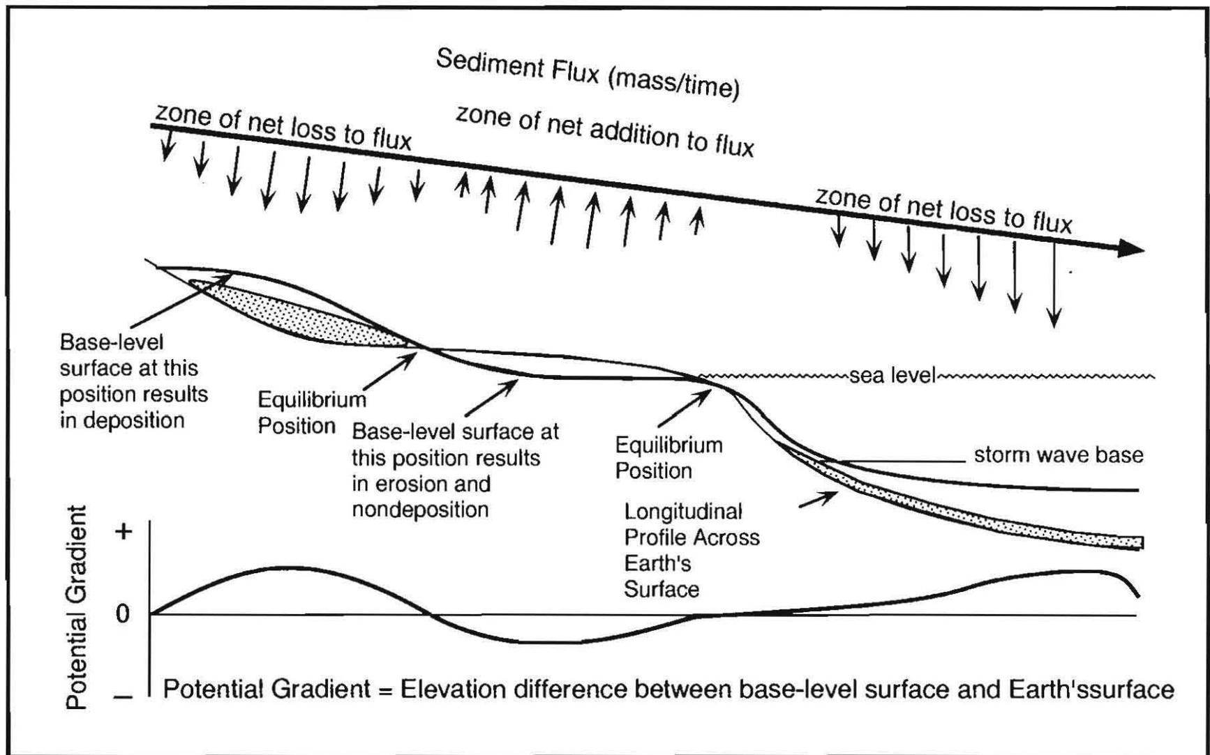
**Figure 9**—Base level is an imaginary potentiometric surface that fluctuates up and down with respect to Earth's surface in response to the energy budget of sediment supply and transfer.
