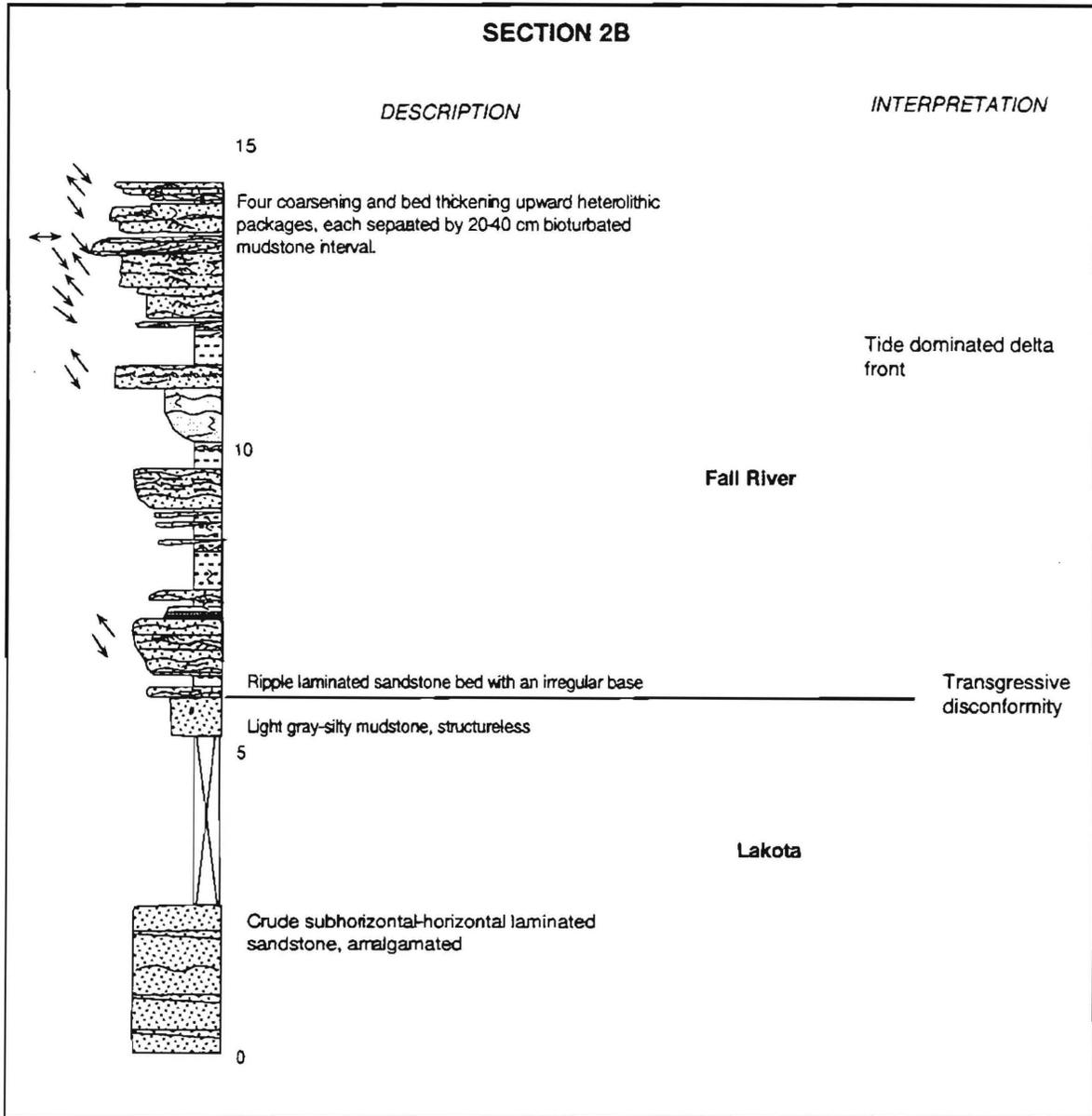
**Figure 85** –Stratigraphic section at location 2B showing four distinct cycles within the first Fall River Sequence
