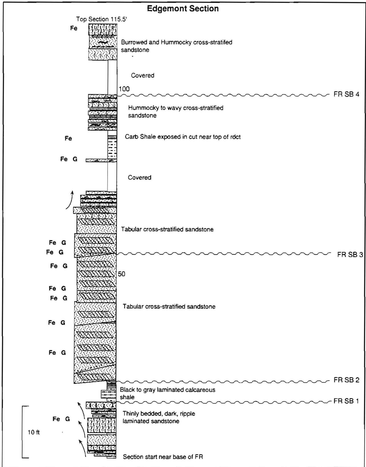
Figure 86—Vertical profile of the Fall River Formation at Edgemont Roadcut.
