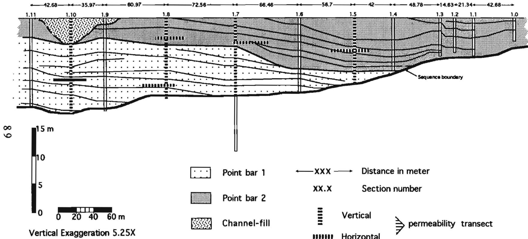
Figure 44— Cross section of SC 4 sandstone bodies at Clifton Canyon
