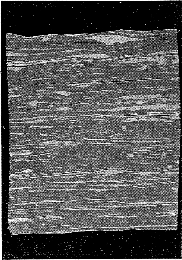
Figure 15. Core photographs of lower distal delta-front facies. Core slabs are 3.5 inches wide. (a) Sparsely burrowed (horizontal burrows as siltstone-filled pods) dark-gray shale with thin lenses and laminae of siltstone and very fine sandstone typical of the thickest deltaic successions in the Cleveland cores. From Maxus Glasgow No. 2 at 7,273 ft (log depth). (b) Heavily burrowed (vertical and horizontal burrows) dark gray shale and siltstone/very fine sandstone that occur in the thinnest deltaic successions. From Maxus Glasgow No. 2 at 7,184 ft (log depth).
