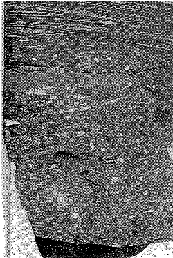
Figure 18. Core photograph of carbonate grainstone in uppermost part of the distal shelf facies. Core slab is 3.5 inches wide. This highly fossiliferous deposit (table 5) is interpreted to represent current-concentrated fossil material that accumulated in an area of sediment starvation on the Cleveland shelf. Note the thin, uneven, nonfossiliferous hardground abruptly truncating the fossil bed about 3 inches above its base. Several bored pelecypod fragments lie below the hardground; a more mud-rich but less fossiliferous thin bed overlies it. Black, organic-rich, fossiliferous clay shale directly underlies the grainstone. Lenticular laminated siltstone and shale of lower distal delta-front and prodelta facies of the lower Cleveland Formation directly overlie the grainstone. From Maxus Glasgow No. 2 at 7,282.5 ft (log depth).
