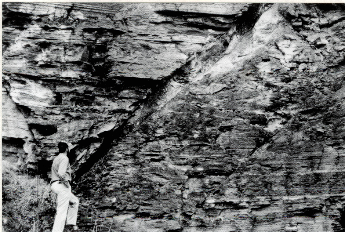
Figure 11. Reverse fault in mudstone with convoluted shaly gouge.
