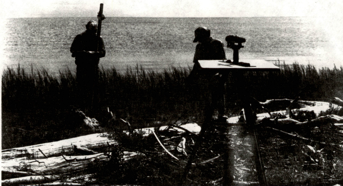
Figure 6. Photograph of plane table, telescopic alidade, and profiling rod used to taking elevations along transects.
