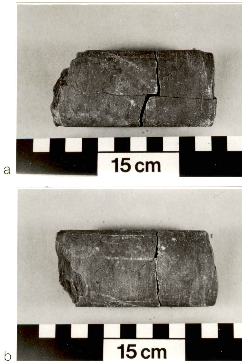
Figure 4. Experimentally compacted Anahuac shale core (9,067.3 ft, 2,764 m) showing (4a), development of vertical and horizontal extension fractures as well as (4b), irregular vertical fracture systems.
