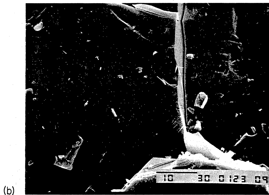
Figure 22. SEM images (a, b) of grain boundary crack, Arkla Scott No. 5, 7,453.3 ft.
